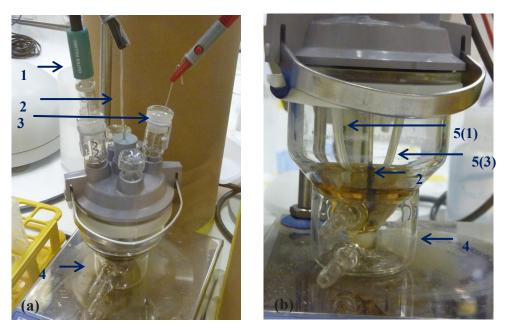
Figure 2.2 Electrochemical reduction system in Ar-glovebox. 1. Ag/AgCl reference electrode; 2. Pt-working electrode; 3. Pt-counter electrode; 4. glass vessel with magnetic stirring bar; 5. Galvanic cells.
