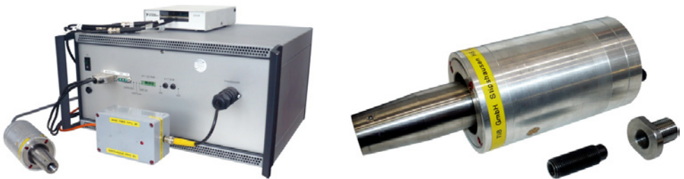
(a) Amplifier TIB S250K, transformer and converter TIB HS USW 1000 with customised National Instruments I/O connector block SCB-68
