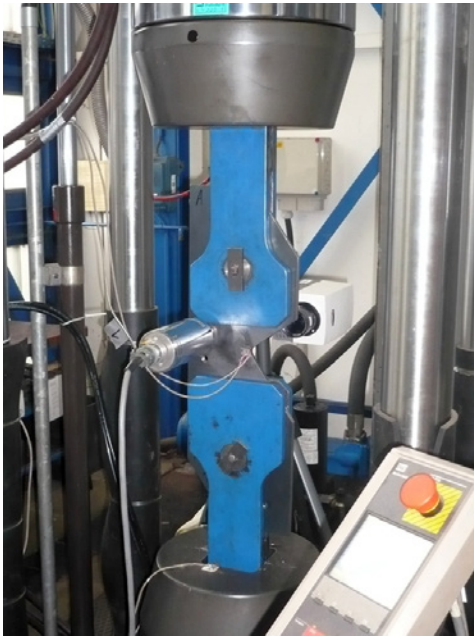
(a) Testing machine, hydraulic grips, mounting fork adapters, plate specimen and infrared camera
