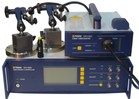
Figure 5.2: Polytec OFV-5000 vibrometer controller, differential fibre-optic interferometer OFV-552, OFV-151 reflector for single-point measurements and two magnetic stands with articulated arm for manual positioning of the laser sensors.
