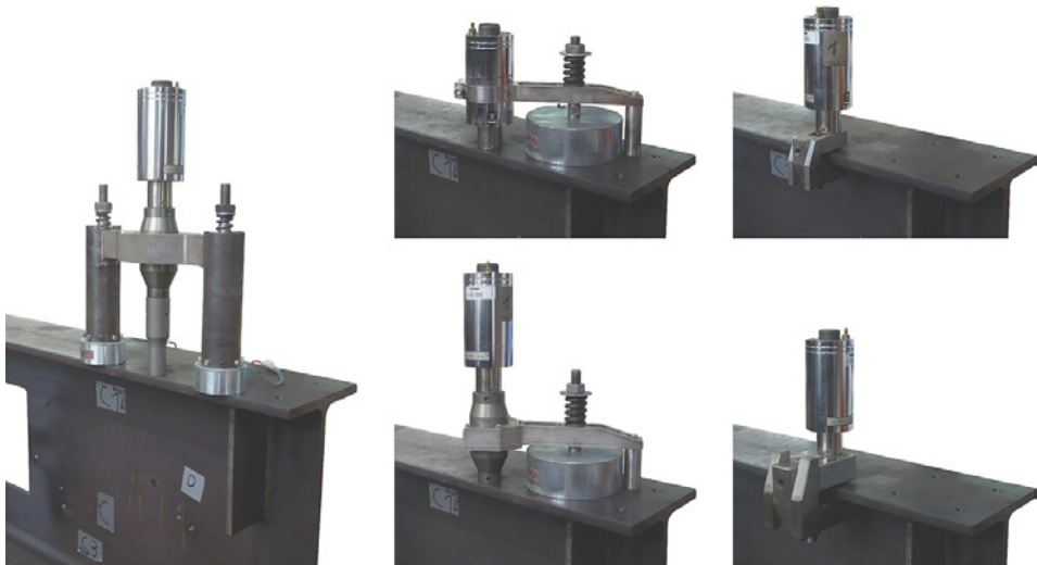
Figure 4.13: Portable coupling devices for in-situ ultrasound excitation.
