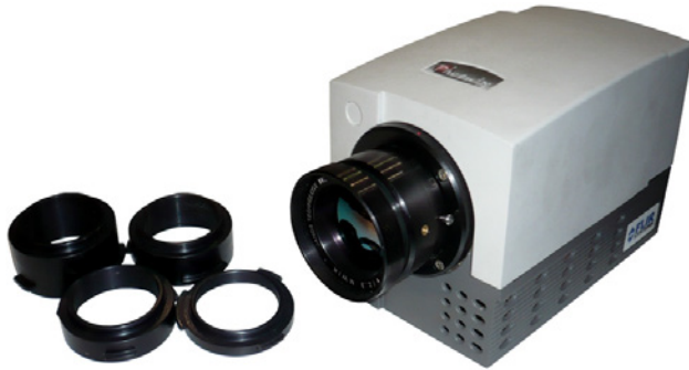
Figure 4.14: Infrared camera head Flir Phoenix DTS (separate digitalisation box not shown) and Janos MWIR Asio 50 mm lens with four extension rings.
