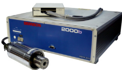
(a) Ultrasound generator Branson 2000b and converter Branson CR20 with customised National Instruments I/O connector block SCB-68
