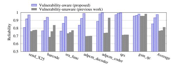
Figure 5.8: Comparison between our vulnerability-aware binding and the vulnerability-unaware binding with the sequence of 10%, 20% and 30% area overhead
