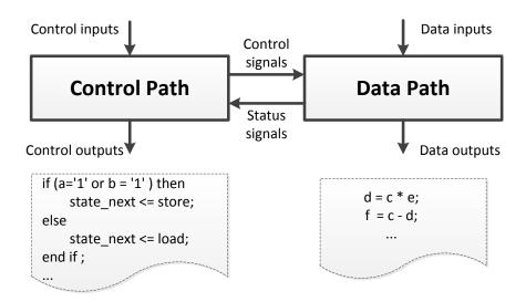
Figure 4.1: RTL control and data paths with code examples
