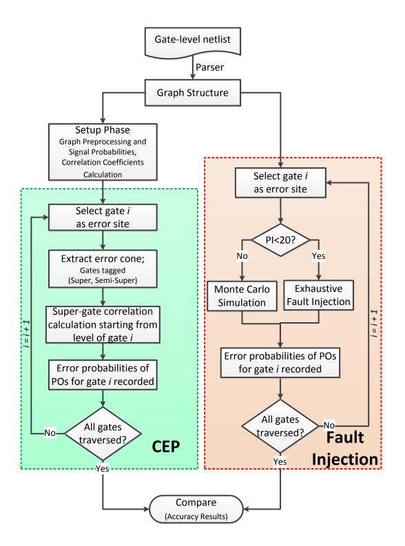
Figure 3.10: Error probability estimation and validation flow
