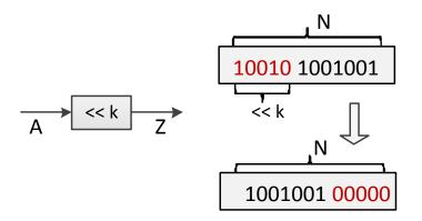
Figure 4.10: Shift operation EPP
