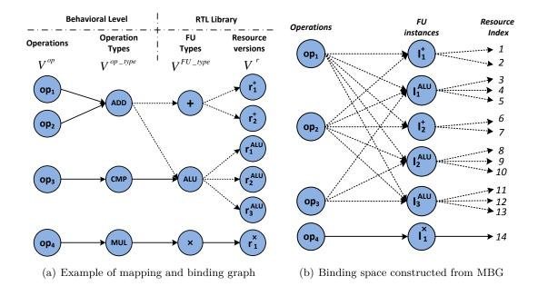
Figure 5.2: An example of resource allocation and binding space determination
