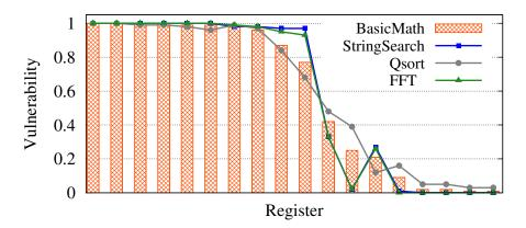
Figure 4.19: Vulnerability ranking of the registers sorted based on the BasicMath workload
