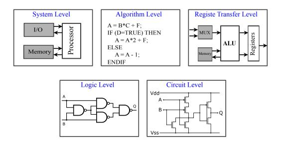
Figure 2.5: Illustration of the design at different abstraction levels
