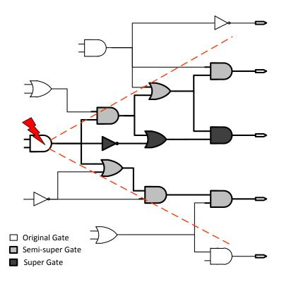
Figure 3.5: Error propagation paths and error cone
