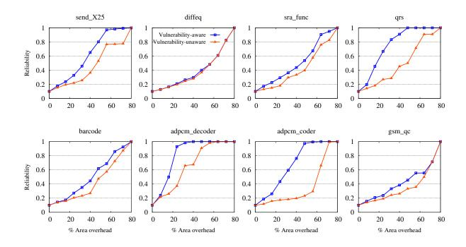
Figure 5.5: The achieved reliability with different level of register protection
