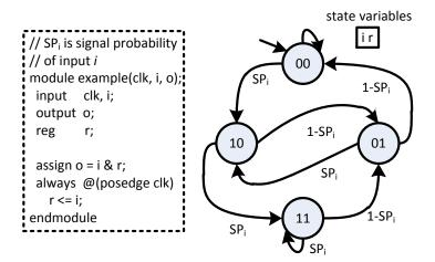
(a) A simple example of an RTL design and the corresponding fault-free DTMC
