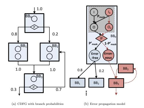
Figure 4.11: Control data flow graph example and our adopted error propagation model
