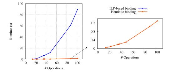
Figure 5.7: Comparison on the runtime of the ILP-based and heuristic binding
