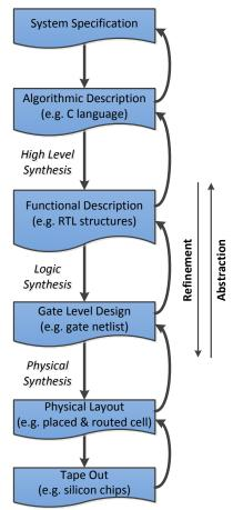
Figure 1.1: A typical digital system design flow
