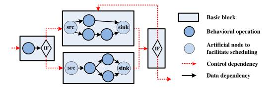
Figure 6.1: An example of control and data flow graph
