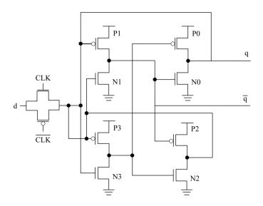
Figure 2.8: Schematic of a DICE latch [3]
