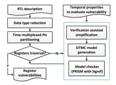
Figure 4.12: Register vulnerability evaluation flow in control paths
