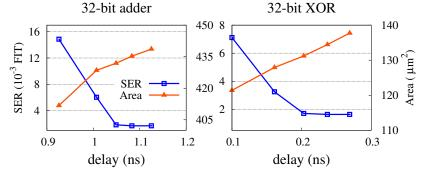
Figure 6.5: Characteristics of two FUs with different hardening levels
