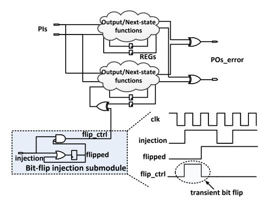
Figure 4.6: Construction of the error checking module
