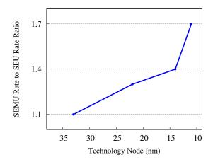
Figure 2.3: Single-event multiple upsets (SEMU) rate to SEU rate ratio for the SRAMs with Siliconon-Insulator CMOS process [1]
