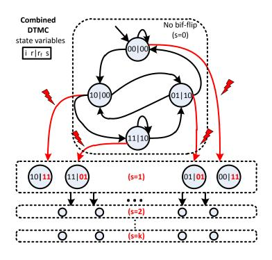
(c) Combined DTMC with soft error in register  $\boldsymbol{r}$
