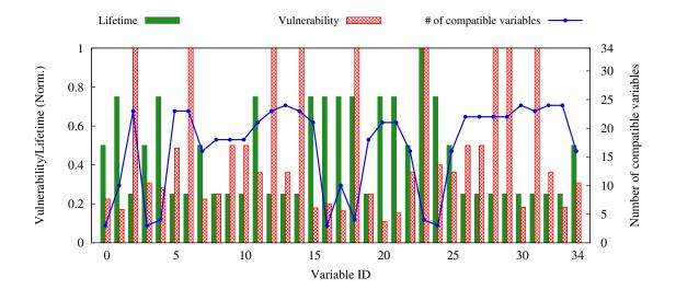
Figure 5.1: The lifetime, vulnerabilities and compatibilities of the variables in the *barcode* benchmark
