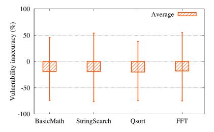
Figure 4.20: Inaccuracy of the register vulnerabilities in related work [5] due to random inputs assumption
