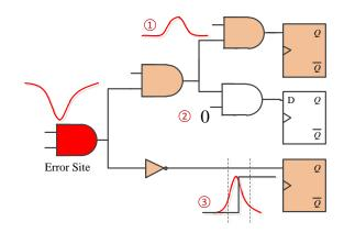
Figure 2.7: Three masking effects in the combinational logic
