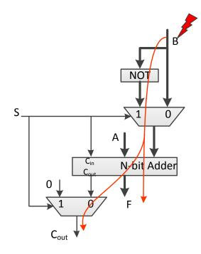
Figure 4.8: RTL-level error propagation
