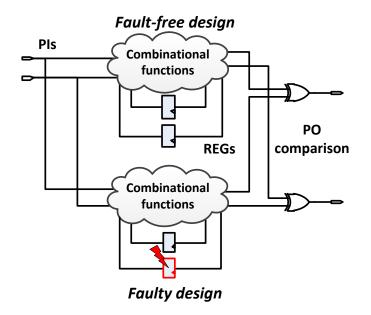
Figure 4.2: Structural view of the RTL error evaluation
