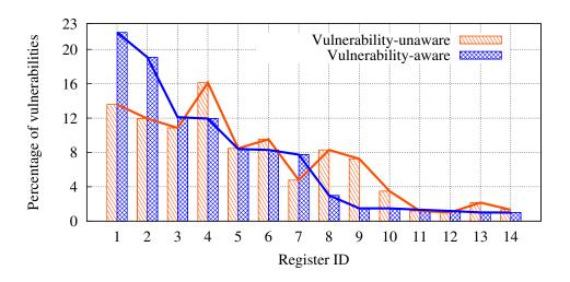
Figure 5.6: Vulnerability distributions of the registers in the vulnerability-unaware baseline and vulnerability-aware binding scenarios for *barcode* benchmark
