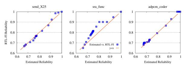
Figure 5.9: Comparison of the reliability values from our behavioral estimation and RTL FI
