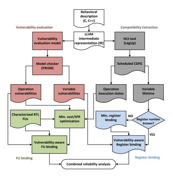
Figure 5.3: Reliability-aware register and FU binding flow
