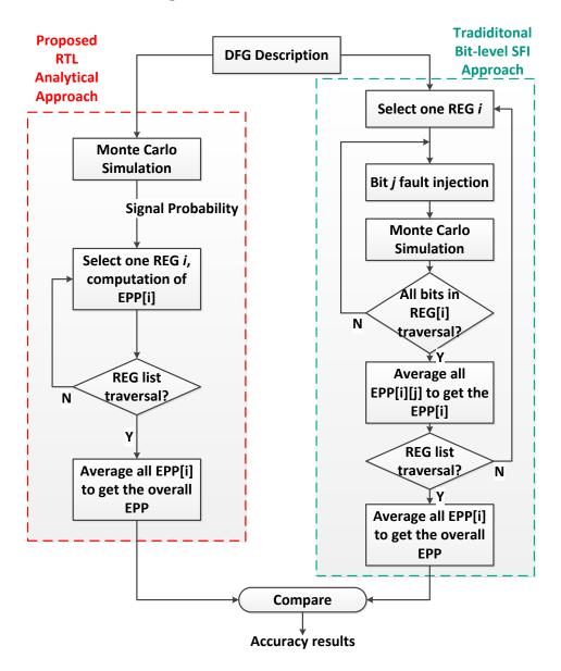
Figure 4.15: Validation Flow of the EPP rules
