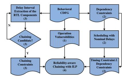
Figure 6.4: Work flow of the proposed operation chaining based on ILP
