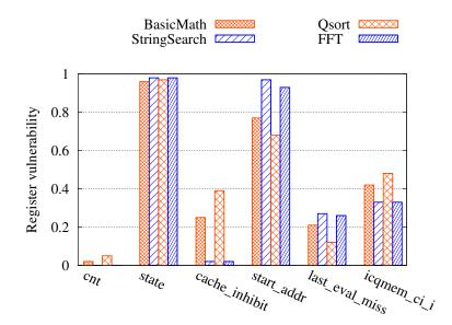
Figure 4.18: Vulnerabilities of representative registers in OR1200 IC FSM with four different workloads
