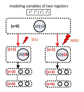
Figure 4.4: Example of modeling the SEU and MBU
