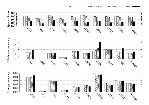
Figure 3.11: Speedup, maximum and average inaccuracy for considering variant correlation depths
