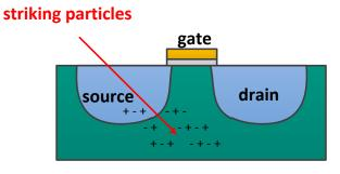
Figure 2.1: Particle striking and the induced ionization in a transistor
