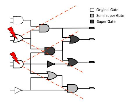
Figure 3.9: Propagation paths with multiple error cones
