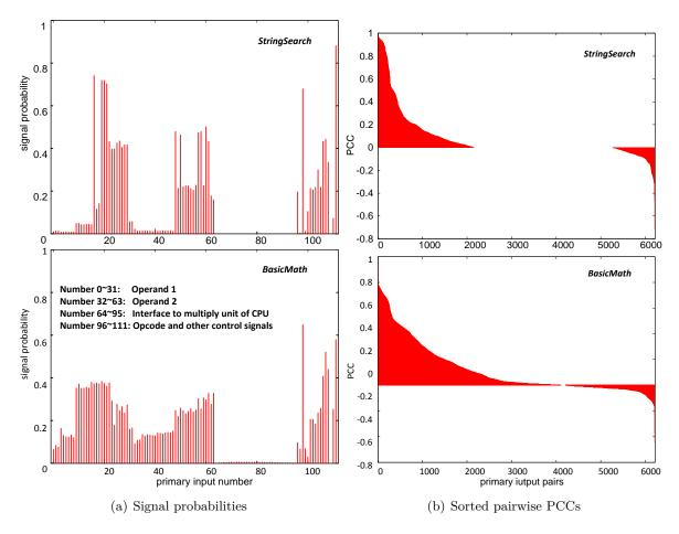
Figure 3.12: Primary input statistics of OpenRISC ALU running applications StringSearch and Basic-Math
