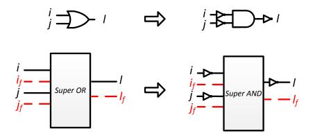
Figure 3.7: Super-AND equivalent of Super-OR gate
