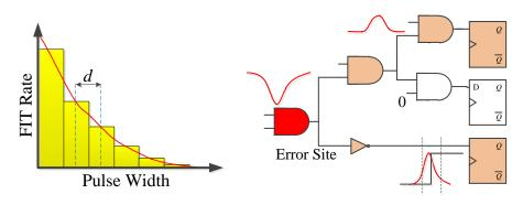
(a) FIT Rate of each pulse width inter- (b) Error propagation with electrical, logic val for the error site gate and timing window masking
