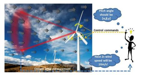
Fig. 1.9.: Sketch of the general idea of Lidar assisted wind turbine pitch control system (Background picture source: Microsoft office template)
