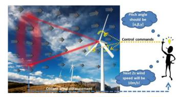
Fig. 1.: Sketch of the general idea of Lidar assisted wind turbine pitch control system (Background picture source: Microsoft office template)
