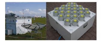
Fig. 3.2: A Sodar system (left), and the antenna array of the Sodar system (right) (Source: Metek)
