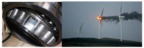
(a) Damages on the gearbox bearing (Source: (b) Generator failure by over speed (Source: BBC) NOAA)
