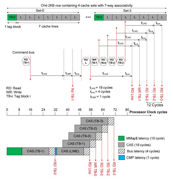
Figure 6.20: Timing and sequence of commands to fill the *DTC* after a *DTC* miss for a data block that belongs to Set-1 in the RBM-A7 policy
