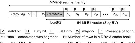
Figure 5.5: MMap\$ segment entry; proposed *SB-Policy* adds an additional Seg-Row field to MMap\$ entry for set balancing
