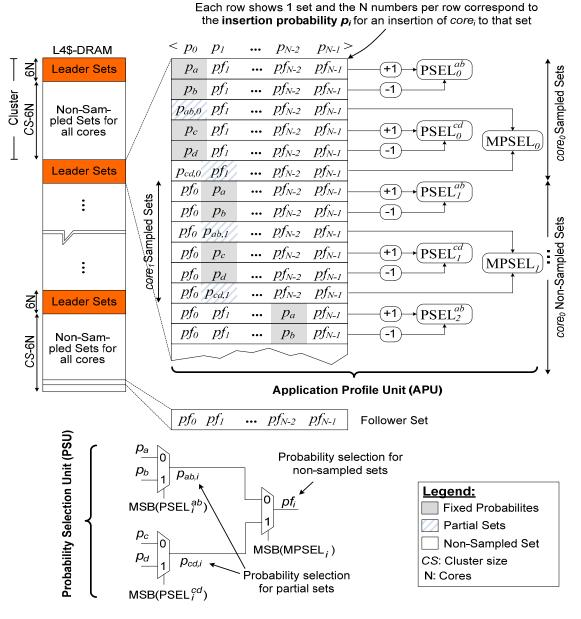
Figure 5.3: Adaptive DRAM Insertion Policy for an N-core system
