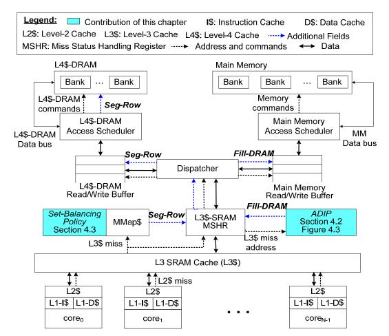
Figure 5.1: Proposed DRAM cache hierarchy for an N-core system; *Fill-DRAM* field indicates whether an incoming block from off-chip memory should be inserted into the L4\$-DRAM or not; *Seg-Row* field is used for set balancing
