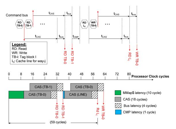
Figure 6.11: Timing and sequence of commands for L4 DRAM read hit that his in the row buffer for configurable row buffer mapping policy
