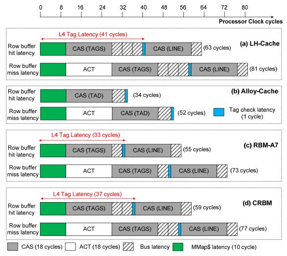
Figure 6.12:L4 DRAM cache Latency breakdown for a 2KB row size (a) LH-Cache [77, 78] (b) Alloy-Cache [102] (c) RBM-A7 [proposed] (d) CRBM [proposed]
