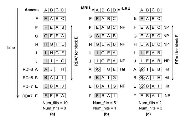
Figure 5.2: Example illustrating DRAM insertion probability of (a) 1, (b) <sup>1</sup>/<sub>2</sub>, and (c) <sup>1</sup>/<sub>4</sub> Block insertion shown as grey, hits shown as shades, NP stands for block not placed in DRAM cache, RD stands for reuse distance
