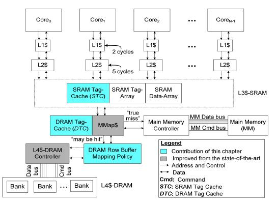
Figure 6.1: SRAM/DRAM cache hierarchy highlighting the novel contributions
