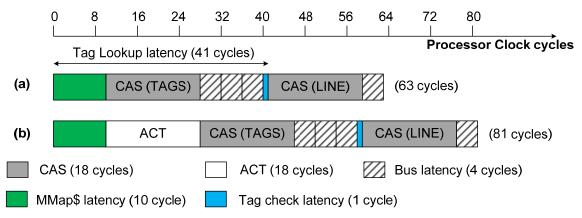
Figure 2.9: LH-Cache (a) row buffer hit latency (b) row buffer miss latency for 2KB row size with T = 3 and A = 29 (see Section 4.2 for details of DRAM cache timing parameters)
