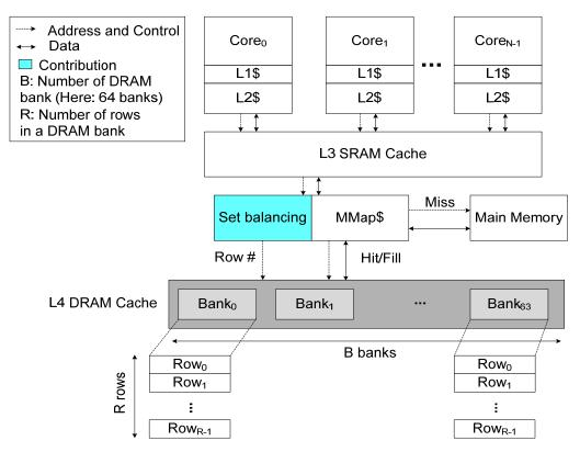
Figure 3.3: High level view of the proposed Set balancing policy
