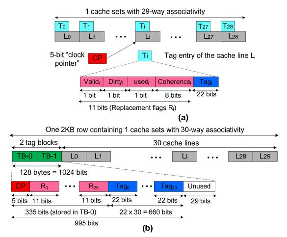
Figure 6.10: (a) Overview of "pseudo LRU" policy (b) how the tag entry fields are organized in configurable row buffer mapping policy
