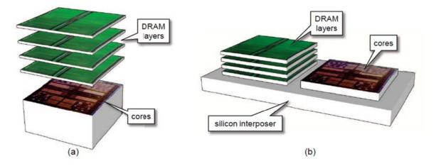
Figure 2.4: Die-stacked DRAM with multi-core chip [77, 78] implemented as (a) a vertical stack (b) silicon interposer
