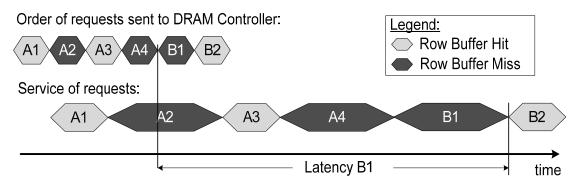
Figure 2.7: Example showing inter-core interference at the DRAM bank
