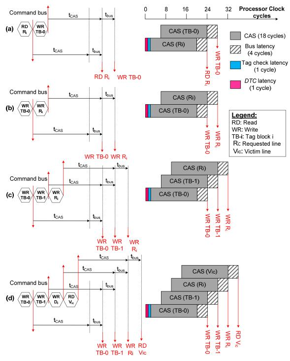
Figure 6.18: Timing and sequence of commands to update the tags in the DRAM cache after a *DTC* hit in the configurable row buffer mapping policy for an L4 DRAM row buffer hit (a) read request (b) write/write-back request (c) fill request with clean victim block eviction (d) fill request with dirty victim block eviction
