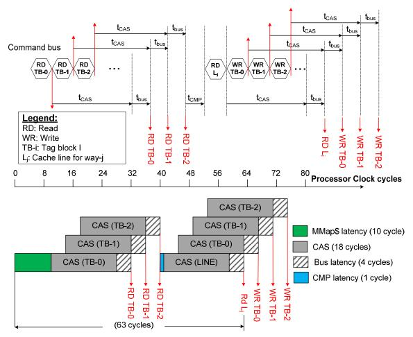
Figure 6.9: Timing and sequence of commands for L4 DRAM hit that his in the row buffer for LH-Cache
