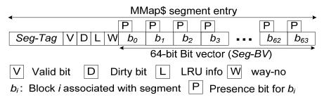
Figure 6.13: MMap\$ entry covering a 4KB memory segment for LH-Cache [77, 78]
