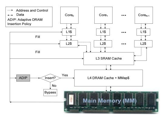
Figure 3.2: High level view of the proposed Adaptive DRAM Insertion Policy
