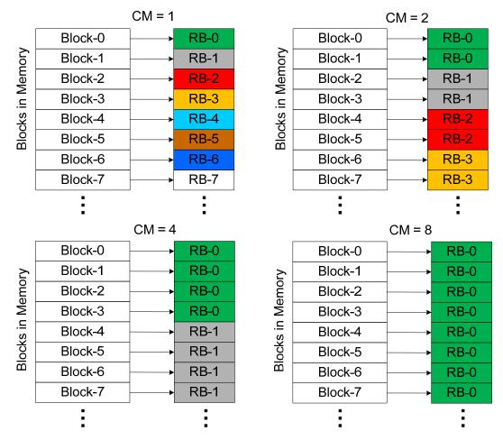
Figure 6.6: Block mapping for configurable row buffer mapping policy with different values of CM
