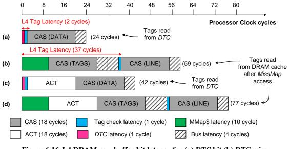
Figure 6.16: L4 DRAM row buffer hit latency for (a) *DTC* hit (b) *DTC* miss L4 DRAM row buffer miss latency for (c) *DTC* hit (d) *DTC* miss
