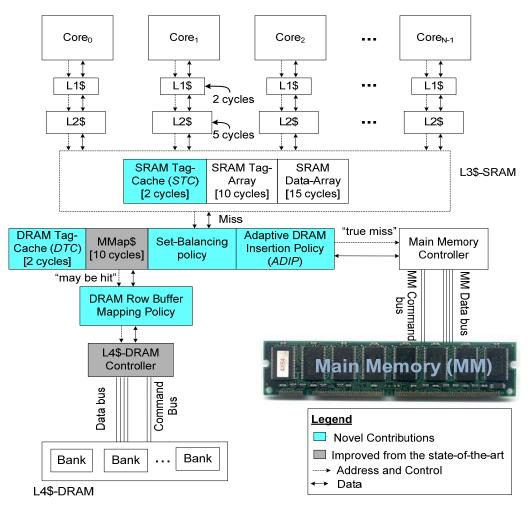
Figure 3.1: Proposed SRAM/DRAM cache hierarchy for an N-core system
