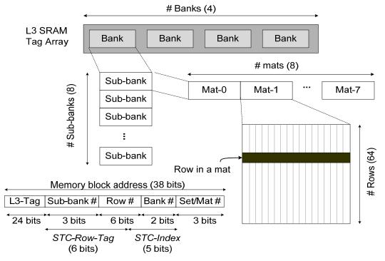
Figure 6.21: Layout of a large L3 SRAM tag array [124]
