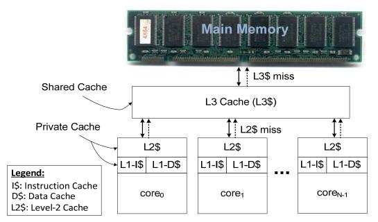
Figure 2.3: A typical three-level multi-core cache hierarchy
