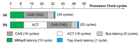
Figure 2.13: Alloy-Cache (a) row buffer hit latency (b) row buffer miss latency (see Section 4.2 for details of DRAM cache timing parameters)
