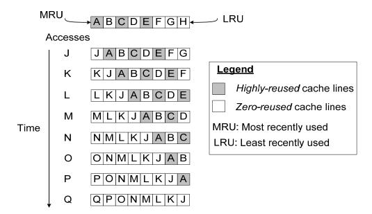
Figure 2.6: Example showing inter-core cache contention between thrashing and nonthrashing applications
