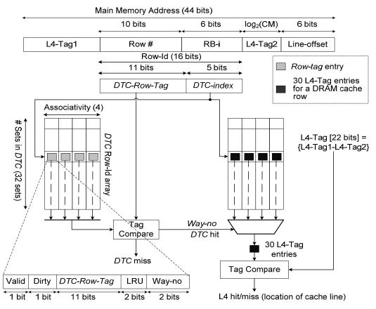
Figure 6.15: DRAM Tag Cache (*DTC*) Organization for configurable row buffer mapping policy
