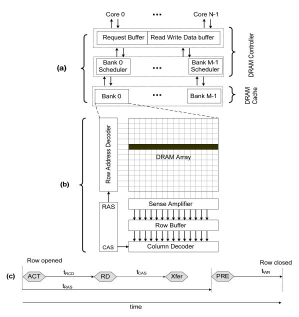
Figure 2.5: (a) DRAM organization (b) DRAM bank organization (c) Timing diagram for a DRAM bank access
