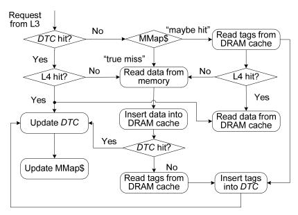
Figure 6.17:DTC and MMap\$ lookup following an L3 SRAM miss
