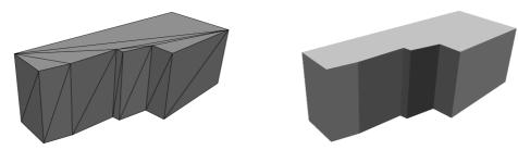
Fig. 105: Net level and object level representation of building model Source: (Breunig, Butwilowski, Golovko, et al. 2013, 102), visualized with ParaViewGeo
