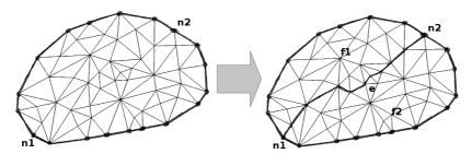
Fig. 79: Example of insertEdge operation, represented on object and on net level
