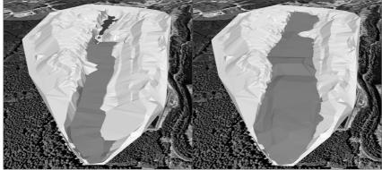
Fig. 14. 3D model of Piesberg landfill site with cells of different usage (1982 and 1993).
