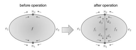
Fig. 81: Adding new cell-tuples when performing insertEdge method
