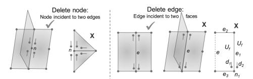
*Fig.* 82: *Examples of valid and invalid spatial configurations for node and edge delete operations*
