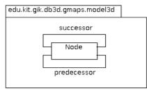
Fig. 98: Basic Node class (of model3d package) extended with temporal field
