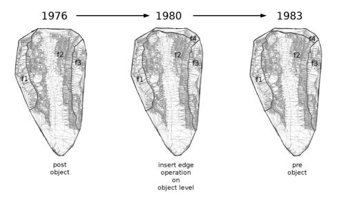
Fig. 100: Adding a new face at object level (in 1980) through insertEdge method
