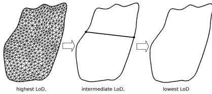
Fig. 26: A subsurface fault, depicted in three levels of detail
