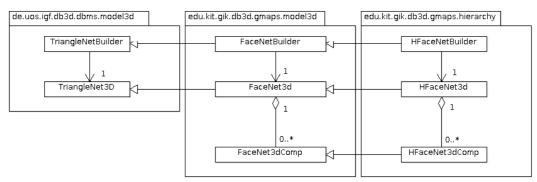
Fig. 84: Architecture of hierarchical net builder as an extension of the cell net builder architecture
