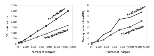
*Fig. 101: Runtimes of net component construction (left); memory consumption of net component construction (right)*
