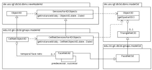
Fig. 93: The extraction of a 3D face net from a temporal cell net object as class diagram
