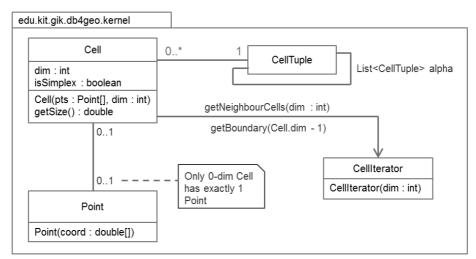
Fig. 107: Classes of dimension-independent cell model approach
