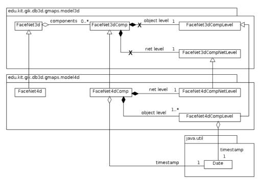
*Fig.* 96: *The temporal net components (with their NL and OL) of temporal face nets in a class diagram*
