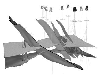
Fig. 2: Typical subsurface model with two strata boundary layers, seven fault layers and visualized well data Source: Visualization using GOCAD software, data from GOCAD workshop 2009
