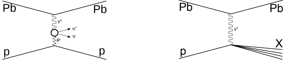
Figure 71: Examples of ultra-peripheral proton-nucleus interactions. Left panel: A quasi-real photon from the field of the lead ion fluctuates into a neutral \rho meson (circle) which interacts with the incoming proton via a colour-singlet state (pomeron exchange) and decays into \pi^+ and \pi^- mesons. Right panel: A quasi-real photon \gamma^* interacts with a parton leading to the break-up of the proton.
