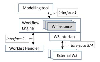
Figure 2.5: Basic Architecture of a WfMS (WfMC Reference Model)
