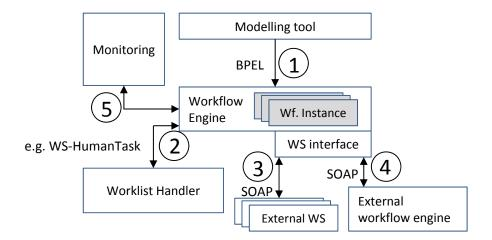
Figure 6.1: Classical architecture of a WfMS in SOA.
