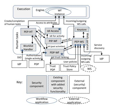
Figure 6.3: Architecture of a WfMS with FIM Support
