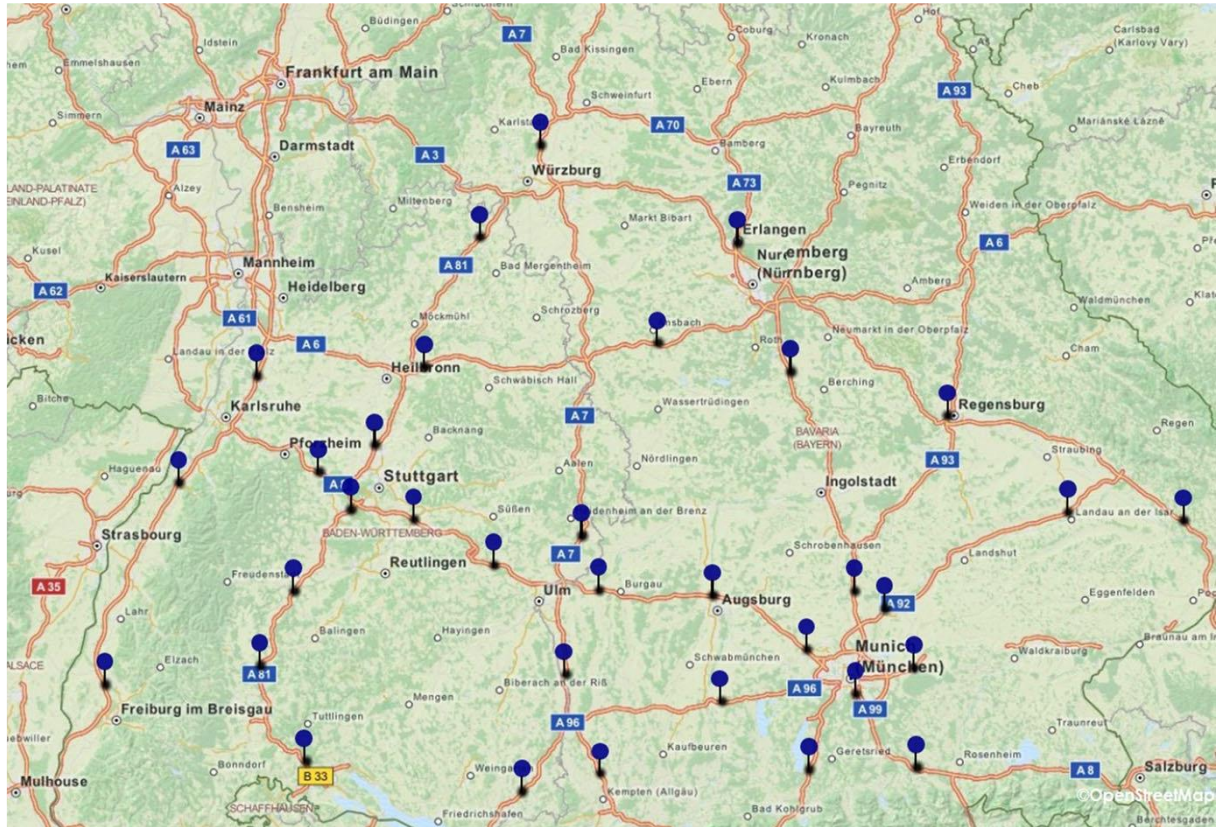
Fig. 3 Allocation of fast charging stations in scenario 3 (100 km range, 80 % coverage)
