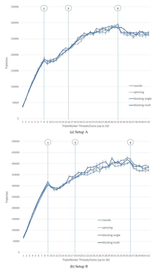
Figure 13: Throughput of of parallel processing of LUBM 200 with OWL LD rule set; number of cores adapted to number of threads (average of 5 runs).
