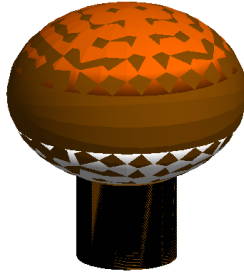
Figure 3.9.: PMT (8”) as implemented in GEANT4. The body consists of borosilicate glass filled with vacuum. A 0.1 mm thin photo-cathode is placed behind the glass front. At the back of the PMT, a thin layer of aluminium with high reflectivity is added. A tube of low reflectivity describes the rubber encasing of the PMT.
