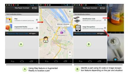
Figure 7.2: Localization of parts in SRA application
