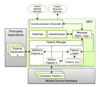
Figure 5.1: Device feature extension model
