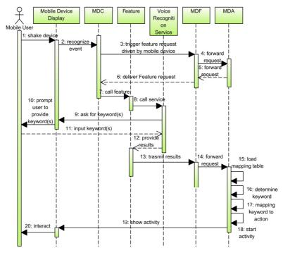
Figure 5.6: Sequence diagram for feature Speech Commander
