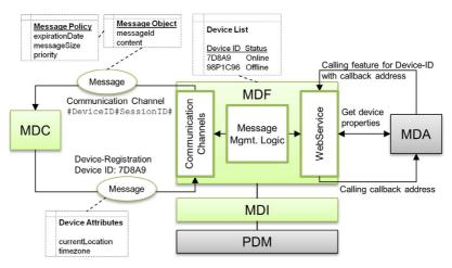
Figure 4.17: Message model workflow
