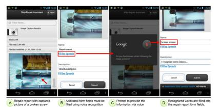
Figure 7.3: Voice-based information capturing in the repair report
