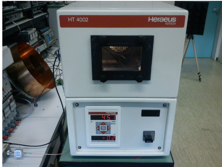
Figure 5.25: Temperature chamber used for the calibration measurement at different temperatures. The part under test is put inside and heated or cooled during the measurement.
