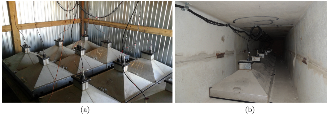
Figure 4.8: (a) Interior of the aluminum huts, housing the scintillator detectors of Tunka-Grande. (b) There are also underground detectors, in a tunnel at a depth of 1.5 m. They are shielded versus electrons and photons, to measure the remaining muonic shower component.
