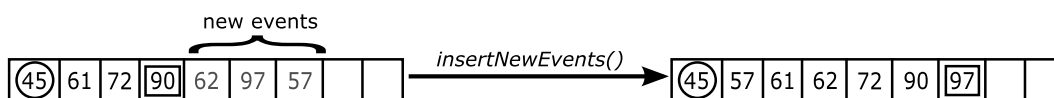
Figure 10.5: During event execution, newly created events are appended to the target LP’s FEL in an unsorted fashion. In a subsequent step, the new events are inserted into the FEL in non-decreasing timestamp order.
