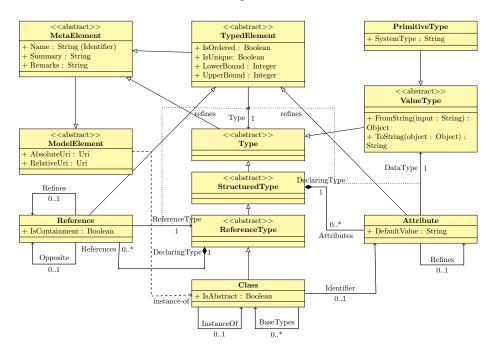
Figure 1. The meta-metamodel NMeta (simplified)
