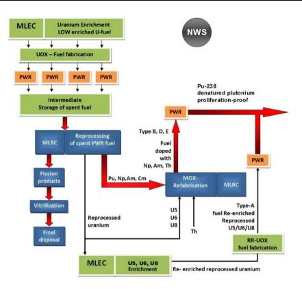
Figure 14.1: Transition phase for the production of proliferation-proof plutonium in NWSs (Reprocessing and Refabrication will in reality be collocated but shown separately here).
