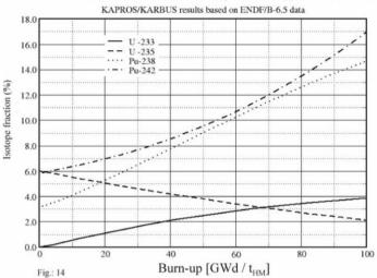
Mass fractions as a function of burn-up for fuel type E with thorium
