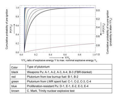
Figure 9.46b: Cumulative probability  $P(Y|Y_0)$  for pre-ignition and cumulative probability  $1-P(Y|Y_0)$  to attain  $Y|Y_0$  for Case 2.
