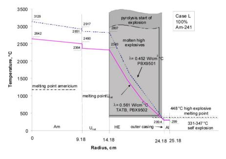
Figure 11.9: Radial temperature profile for a reactor-americium based HNED (option L 100% Am-241).
