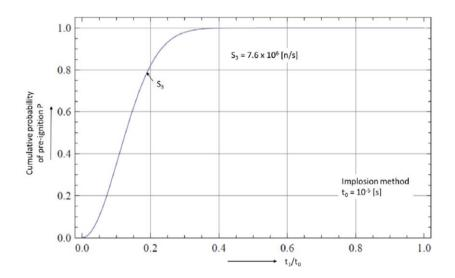
Figure 16.11: Cumulative probability of pre-ignition for a time period  $10^{-5}$ s and spontaneous fission neutron source  $S_3 = 7.6 \times 10^6$  n/s.
