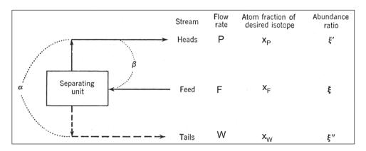
Figure 3.1: Separating unit and definitions.
