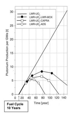
Figure 7.17: Balance of plutonium (normalized to 1 GW(e)) from a cluster of M=8 UOX-PWRs with 10 GW(e) total power operating in either the once through direct spent fuel disposal mode (straight line). The polygon type lines show the pluto-nium inventory (normalized to 1 GW(e) for the cases of UOX-PWRs operating in symbiosis with either MOX-PWRs or FR-burners (CAPRA-type) or ADSs.
