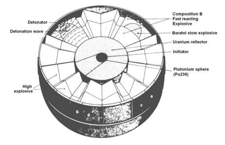
Figure 9.3: Design of the first plutonium NED (Fat Man) [33].
