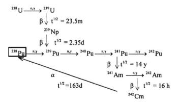
Figure 12.1: Different production routes for Pu-238.
