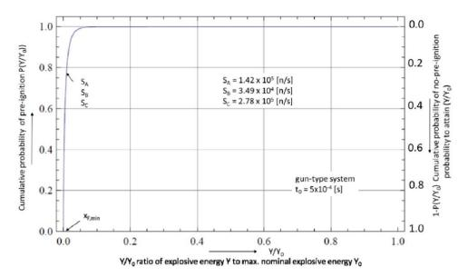
Figure 18.7: Cumulative probability of pre-ignition as a function of the ratio *x* of the attainable nuclear explosive yield *Y* to the maximum nominal yield *Yo* for the time period of compaction  $t_0 = 5 \times 10^{-4}$  s. Spontaneous fission and ( $\alpha$ ,n)-neutron sources *S*<sub>A</sub>, *S*<sub>B</sub>, and *S*<sub>C</sub>.
