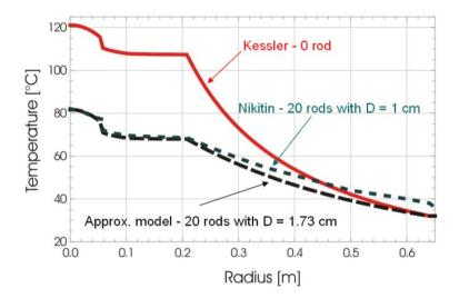
Figure 10.19: The radial temperature distribution of the cases of 0 and 20 aluminum rods of 1 cm and 1.73 cm diameter inserted. Alpha-particle heat power P = 0.144 kW (low-technology case).
