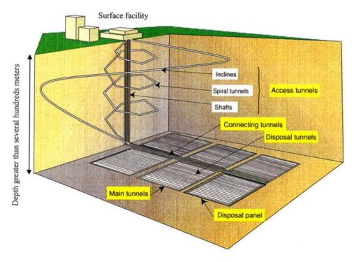
Figure 7.10: Deep repository for HLW and  $\alpha$ -emitter contaminated decay heat producing waste [15].
