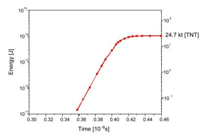
Figure 9.11: Energy release as function of time 10<sup>-6</sup> s.
