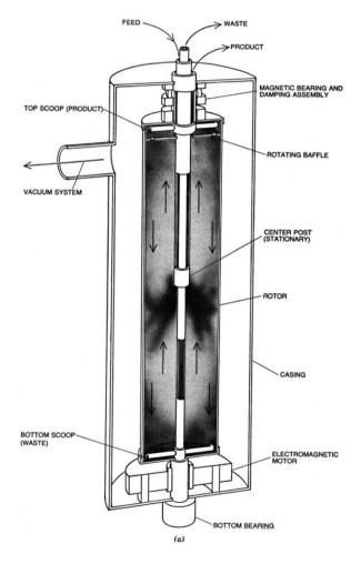
Figure 15.2: Gas Ultra-Centrifuge design [15].
