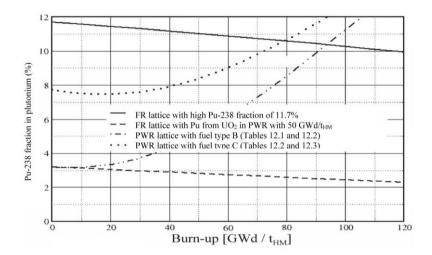
Figure 12.5: Plutonium-238 fraction in fuel in thermal and fast neutron spectrum as a functiion of burnup.
