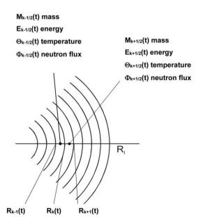
Figure 9.5: Spherical shells of the HNED for the numerical analysis.
