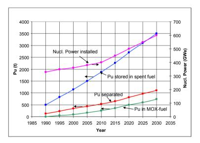
Figure 1.1: Nuclear power installed as well as plutonium stored in spent fuel elements, plutonium separated and plutonium in MOX fuel until 2030 [18].
