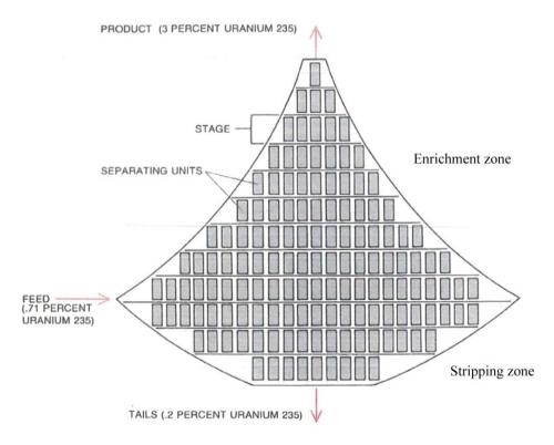
Figure 15.3: Ideal cascade; is made up of stages, each one consisting of a number of gas ultra-centrifuges operating in parallel to provide the required flow of material [15].
