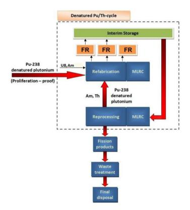
Figure 14.3: Incineration of proliferation-proof plutonium in FRs. Future civil international proliferationproof fuel cycle.
