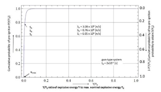
Figure 18.10: Cumulative probability of pre-ignition as a function of the ratio x of the attainable explosive yield Y and the maximum nominal yield  $Y_0$  for the time period  $t_0=2x10^{-5}$ s (implosion method) as well as spontaneous fission and ( $\alpha$ ,n)-neutron sources of  $S_A$ ,  $S_B$ , and  $S_C$ .
