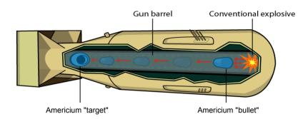
Figure 11.4: Gun-type HNED based on reactor-americium [47,48] (adapted).
