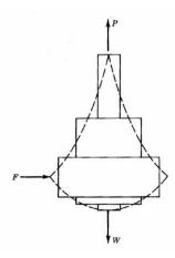
Figure 3.4: Ideal cascade approximation using squere sections.
