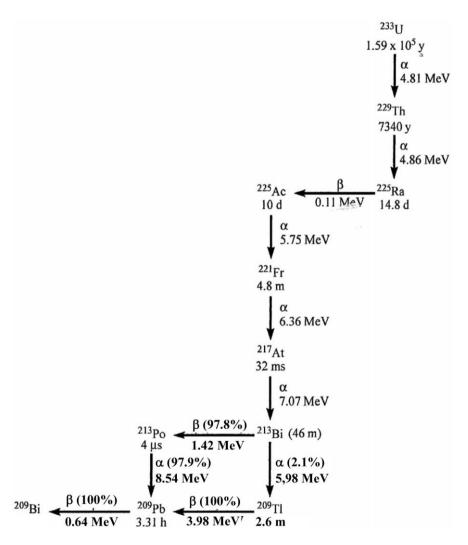
Figure 17.5: Decay chain of U-233 [15, slightly adapted].
