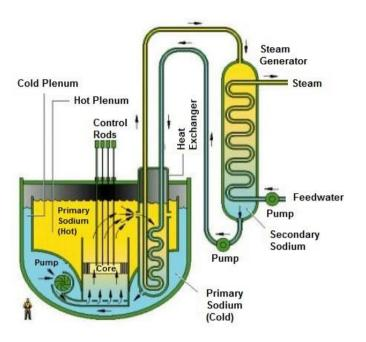
Figure 6.2: Design scheme of a pool type SFR (AREVA).
