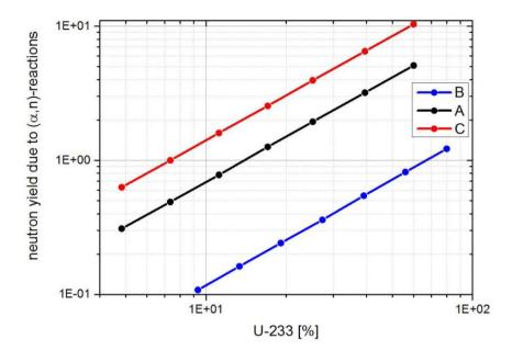
Figure 18.2: Neutron Yield from  $(\alpha,n)$ -reactions with light elements as impurities in uranium during enrichment in the 6 enriching stages of the 10 stages gas ultra-centrifuge cascade ( for fuel type examples A, B, and C).
