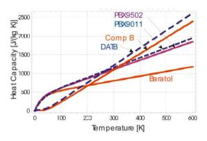
Figure 10.14: Heat capacity of chemical high explosives down to cryogenic temperatures.
