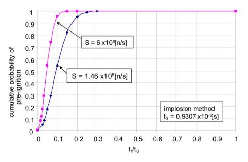
Figure 9.26: Cumulative probability of pre-ignition (Case B for 0.11 TPa) and two different spontaneous fission neutron sources.
