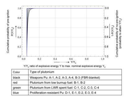
Figure 9.46a: Cumulative probability  $P(Y|Y_0)$  for pre-ignition and cumulative probability  $1-P(Y|Y_0)$  to attain  $Y|Y_0$  for Case 1.
