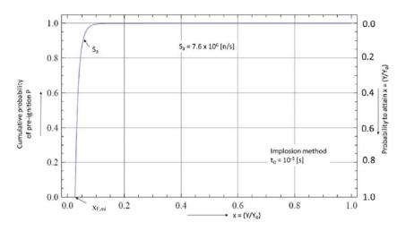
Figure 16.12: Cumulative probability of pre-ignition as a function of the ratio x of the attainable explosive yield Y and the maximum nominal yield  $Y_0$  for the time period  $t_0=10^{-5}$  s (implosion method) and spontaneous fission and ( $\alpha$ ,n)-neutron source of  $S_3=7.6 \times 10^6$  n/s.
