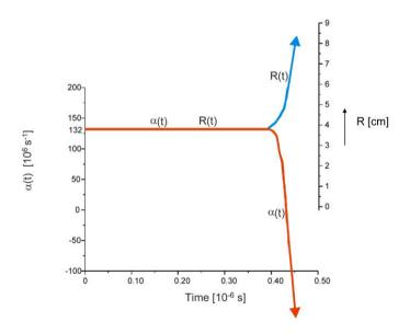
Figure 9.9: Rossi  $\alpha$  (t) and outer radius, R(t), of the Pu sphere as a function of time.
