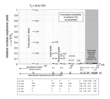
Figure 9.47: Relative nuclear explosive  $Y/Y_0$  with cumulative probability for achievement for the different plutonium compositions (weapon-grade and reactor-grade).
