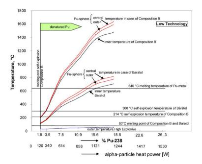
Figure 10.9: Temperature profiles in an HNED with low technology and different values of alpha-particle heat power.
