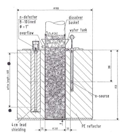
Figure 8.19: Arrangement for measurement of hulls in the dissolver basket [3].
