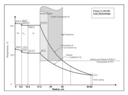
Figure 10.6: Temperature profiles in a low technology HNED with an alpha-particle heat power of 0.144 kW.
