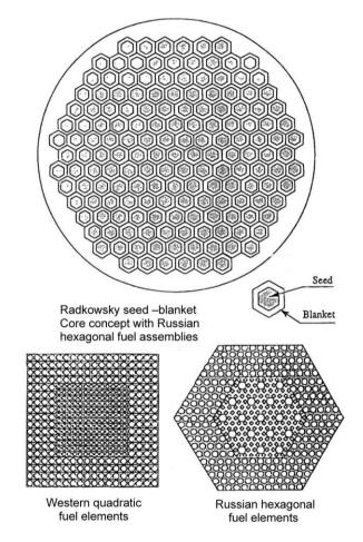
Figure 17.3: This design concept can operate with 19,95% U-235 enriched uranium<sup>1</sup> [5,6] or it allows the incineration of plutonium (weapons plutonium [6,7]) in the seed part of the seed-blanket assembly and it can achieve conversion of U-233 via neutron capture in thorium-232 in its blanket part.
