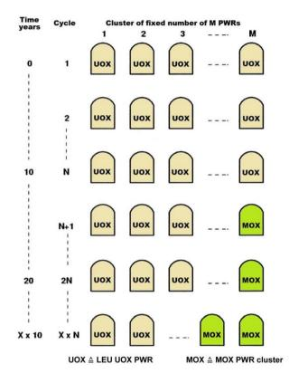
Figure 7.13: Scenario for plutonium multi-recycling in the SGR mode for a cluster of M of PWRs.
