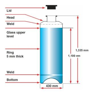
Figure 7.7: Borosilicate HLW container [13].
