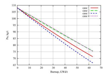
Figure 13.6: Plutonium content in the fuel during burnup [17].
