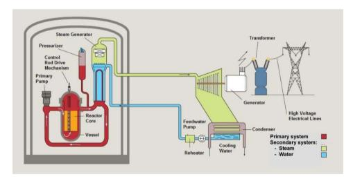
Figure 5.1: Main design principles of the European Pressured Water Reactor (AREVA).
