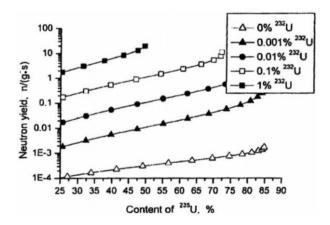
Figure 16.5: Neutron yield from ( $\alpha$ ,n)-reactions of light elements in 19.95% re-enriched uranium and different U-232 contents (decay chain of U-232 not taken into account [5]).
