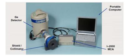
Figure 8.5: Multi-channel analyzer with Ge-detector used by IAEA [30,31,34].
