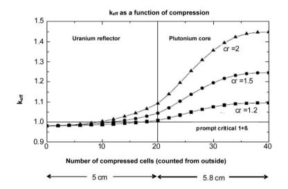
Figure 9.20:  $k_{eff}$  as a function of the compression ratio and the number of compressed spherical shells (from outside). The natural-uranium reflector of 5 cm thickness and the plutonium sphere of 5.8 cm radius are subdivided into 20 radial shells each (only every second result shown, cr = compression ratio).
