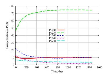
Figure 13.14: Fractions (%) of the different plutonium isotopes as a function of time in the radial blanket fuel elements. The initial plutonium composition with 11.4% Pu-238 remains always above 8% Pu-238 (proliferation-proof) over the full irradiation time period in the FBR [30].
