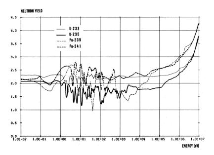
Figure 4.11: Neutron yield as a function of energy of incident neutron causing fission for U-233, U-235, Pu-239, Pu-241 [32].
