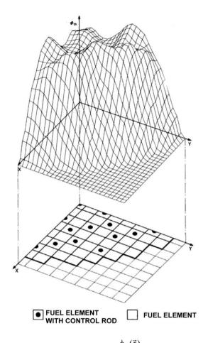
Figure 4.5: Spatial distribution of the thermal neutron flux,  $\phi_{th}(\vec{r})$ , in a PWR core with partially inserted control rods [24].
