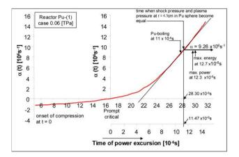
Figure 9.31: Dependence on time of Rossi alpha,  $\alpha(t)$ , after compression or after transition through prompt criticality (0.06 TPa case).
