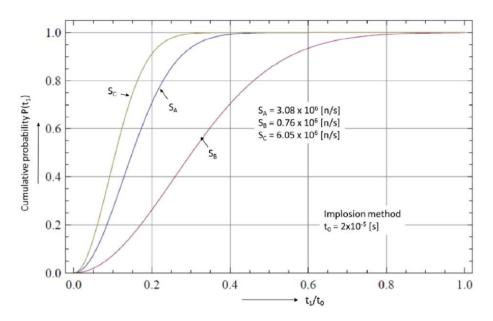
Figure 18.8: Cumulative probability of pre-ignition for a time period  $t_0 = 2 \times 10^{-5}$ s and internal spontaneous and  $(\alpha, n)$ -neutron sources  $S_A, S_B$ , and  $S_C$  as a function of  $t_1/t_0$ .
