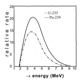
Figure 8.8: Theoretical anti-neutrino energy spectra for U-235 and Pu-239 [35].
