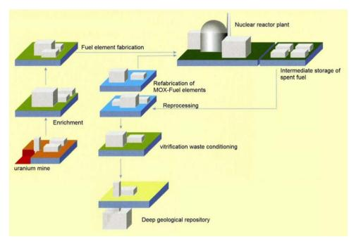
Figure 7.12: The closed nuclear U/Pu (MOX) fuel cycle for PWRs.
