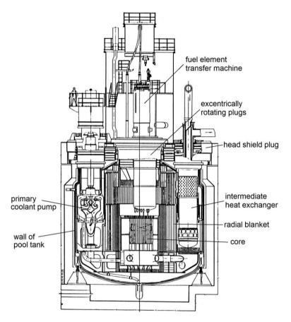
Figure 6.4: BN-600 pool type sodium cooled fast reactor [9].
