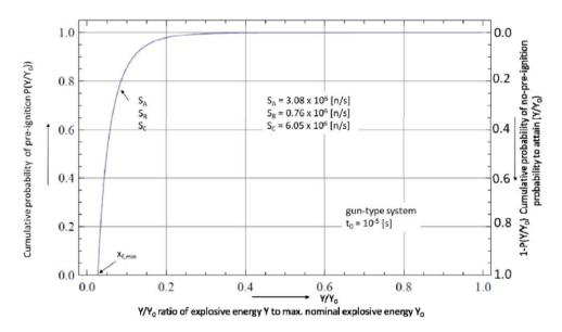
Figure 18.11: Cumulative probability of pre-ignition as a function of the ratio x of the attainable explosive yield Y and the maximum nominal yield  $Y_0$  for the time period  $t_0=10^{-5}$ s (implosion method) as well as spontaneous fission and  $(\alpha,n)$ -neutron sources of  $S_A$ ,  $S_B$ , and  $S_C$ .
