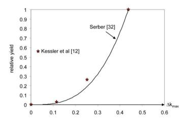
Figure 9.12: Comparison of Serber relation [32] and calculations by Kessler et al. [12].
