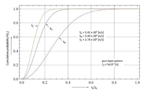
Figure 18.5: Cumulative probability of pre-ignition for a time period of  $t_0 = 5 \times 10^{-4}$  s of compaction by gun-type system as a function of  $t_1/t_0$ . Spontaneous and  $(\alpha, n)$ -neutron source,  $S_A$ ,  $S_B$ , and  $S_C$
