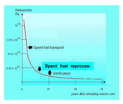
Figure 7.4: Radioactivity of 1 t of spent fuel as a function of time.
