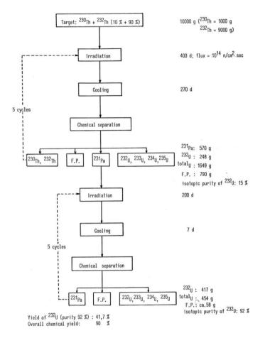
Figure 16.3: Production scheme for U-232 after irradiation of Th- 230 and Th- 232 [2,3].
