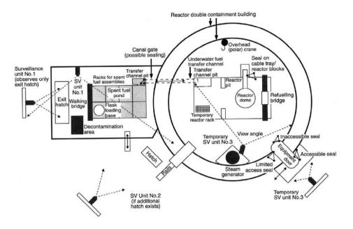
Figure 8.2: Material balance area of a Light Water Reactor.
