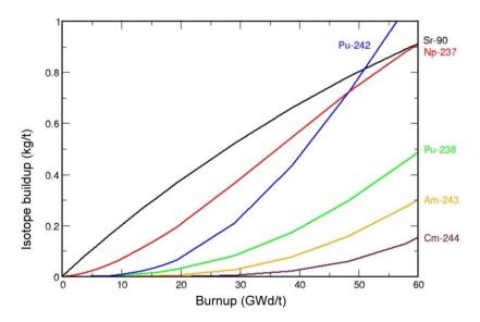
Figure 4.8b: Isotope concentrations for Pu-242, Sr-90, Np-237, Pu-238, Am-243, Cm-244 as a function of burnup [GWd/ton] of LWR fuel. Initial fuel enrichment: 5% U-235 [32].
