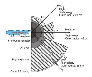
Figure 10.2: Assumed geometric dimensions for three classes of technology.
