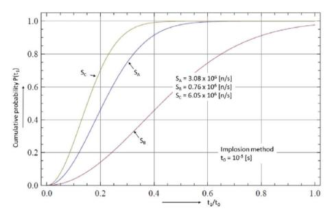
Figure 18.9: Cumulative probability of pre-ignition for a time period  $t_0=10^{-5}$ s and internal spontaneous and  $(\alpha,n)$ -neutron source  $S_A$ ,  $S_B$ , and  $S_C$  as a function of  $t_I/t_0$ .
