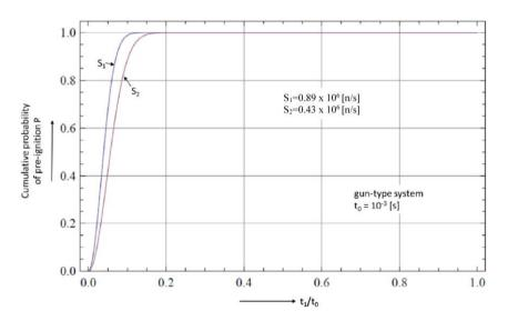
Figure 16.7: Cumulative probability of pre-ignition for a time period of  $t_0 = 10^{-3}$  s of compaction by a gun-type system as a function of  $t_1/t_0$ . Neutron source  $S_1 = 0.89 \times 10^6$  n/s and  $S_2 = 0.43 \times 10^6$  n/s.
