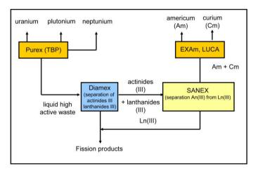
Figure 7.18: Partitioning processes for uranium, plutonium, neptunium, americium and curium in Europe [34].
