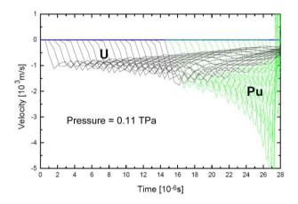
Figure 9.17: Particle velocity,  $u_P$ , of the different spherical shells at different times (10<sup>-6</sup> s) in a solid plutonium sphere with a natural-uranium reflector. The outside pressure at the reflector boundary is a constant 0.11 TPa.
