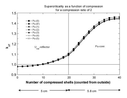
Figure 9.21: k<sub>eff</sub> for all Pu-mixtures Pu-(0) to Pu-(5), and a compression ratio, cr = 2 (spherical shells successively compressed from the outside; only every second value is shown).
