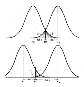
Figure 8.1: Relations between detection probability, rate of false alarms, detectable quantity and measuring accuracy.
