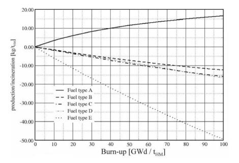
Figure 12.6: Denatured reactor plutonium inventory changes in 1 tonne fuel when loaded into PWR core as a function of burnup of fuel types considered.
