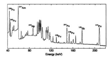
Figure 8.4: High resolution gamma spectra of Sb, Np-, Pu- and Am-fraction [13].
