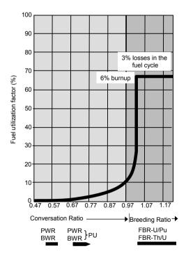
Figure 4.12: Fuel utilization [%] as a function of the conversion ratio for LWRs (PWRs or BWRs), plutonium recycling PWRs or BWRs and FBRs operating in the U/Pu-cycle or the Th/U-cycle [31].
