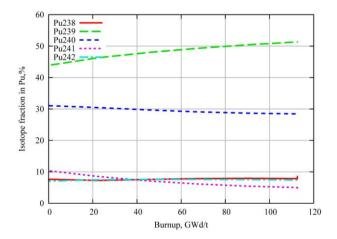
Figure 13.11: Average plutonium isotopic composition in the FR breeder (core and breeder fuel mixed after unloading) [17].
