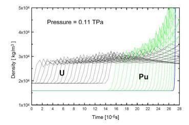
Figure 9.16: Density of each spherical shell as a function of time (10<sup>-6</sup>s) in a solid plutonium sphere with a natural uranium reflector. The outside pressure at the reflector boundary is a constant 0.11 TPa.
