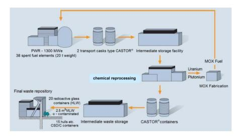
Figure 7.9: HLW radioactive glass containers and α-emitter contaminated decay heat producing MLW from a 1.3 GWe LWR plant generated per year (VGB).
