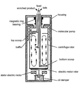
Figure 3.6: Russian gas centrifuge design according to Kamenev [11].
