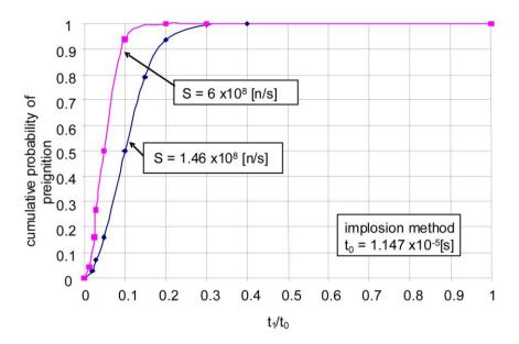
Figure 9.25: Cumulative probability of pre-ignition (Case A for 0.06 TPa) and two different spontaneous fission neutron sources.
