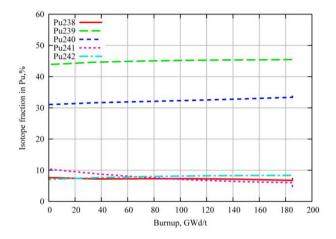
Figure 13.10: Plutonium isotopic composition in the core of the FR operating as burner [17].
