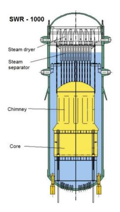
Figure 5.10: Reactor Pressure Vessel of SWR-1000 (AREVA).
