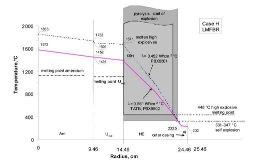
Figure 11.7: Radial temperature profile for a reactor americium based HNED (option H LMFBR).
