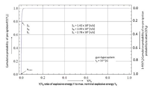
Figure 18.6: Cumulative probability of pre-ignition as a function of the ratio *x* of the attainable nuclear explosive yield *Y* to the maximum nominal yield *Y<sub>o</sub>* for the time period of compaction  $t_0 = 10^{-3}$  s. Spontaneous fission and ( $\alpha$ ,n)-neutron source *S*<sub>A</sub>, *S*<sub>B</sub>, and *S*<sub>C</sub>.
