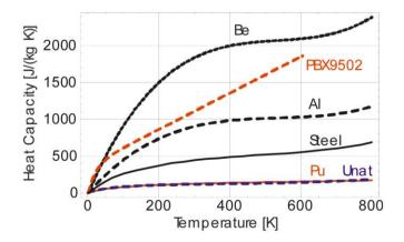
Figure 10.13: Heat capacity of metals down to cryogenic temperatures.
