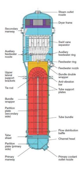
Figure 5.5: Cutaway of EPR steam generator (AREVA).
