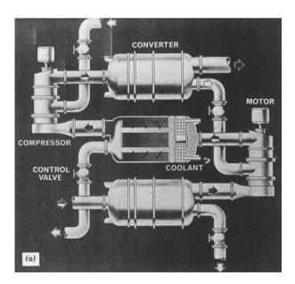
Figure 3.5: Basic stage equipment in a gaseous diffusion cascade [7].
