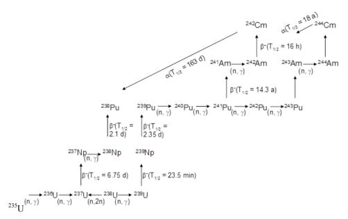
Figure 4.7: Uranium-plutonium reaction chain with buildup of neptunium, americium and curium.
