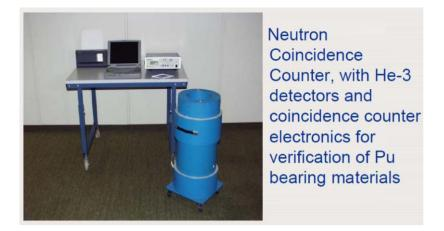
Figure 8.6: Neutron coincidence counter used by IAEA [30,31,34].
