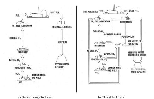
Figure 2.2: The nuclear fuel cycle (once through and closed fuel cycle) (NUREG).
