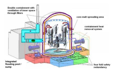
Figure 5.6: EPR double containment with RPV, cooling systems and molten core spreading area (AREVA).
