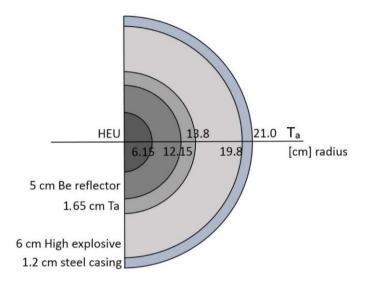
Figure 16.14: Geometric dimensions of the high-technology HNED.
