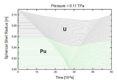
Figure 9.14: Spherical shell radius as a function of time [10<sup>-6</sup> s] in a solid plutonium sphere and a natural uranium reflector.
