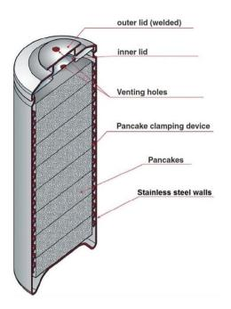
Figure 7.8: CSD-C container with compacted hulls and steel parts [13].
