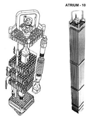
Figure 5.9: ATRIUM-10 boiling water reactor fuel element [7,9,10].
