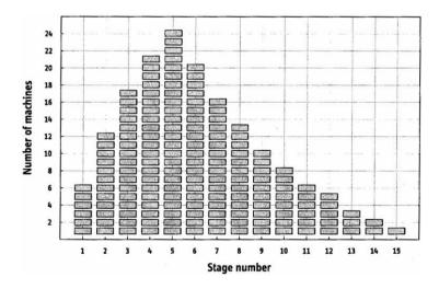
Figure 15.4: Possible arrangement of 164 machines in a 15-stage cascade [7].
