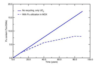
Figure 7.14: Balance of plutonium collected from a cluster of M = 8 UOX: PWRs with 10 GWe total power operating in the once through direct spent fuel disposal mode (full line) and inventory of plutonium in the cluster of M = 8 UOX and MOX PWRs with 10 GWe power (Pu content or inventory normalized to 1 GW(e)) [28].
