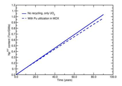
Figure 7.15: Amount of neptunium generated by a cluster of M = 8 UOX PWRs (full line). Amount of neptunium generated by a cluster of M = 8 UOX and MOX PWRs operating in the SGR-mode (dotted line). The amounts are normalized to 1 GWe [28].
