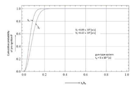
Figure 16.8: Cumulative probability of pre-ignition for a time period of  $t_0 = 5 \times 10^{-4}$  s of compaction by gun-type system as a function of  $t_1/t_0$ . Spontaneous neutron source  $S_1 = 0.89 \times 10^6$  n/s and  $S_2 = 0.43 \times 10^6$  n/s.
