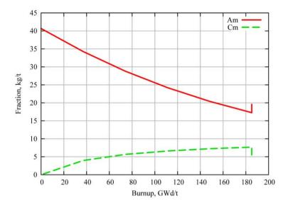
Figure 13.16: Americium and curium content in the burner during reactor operation [17].
