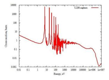
Figure 4.3: Microscopic capture cross section of U-238.
