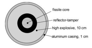
Figure 11.5: Geometric arrangement and dimensions for scoping studies of critical masses for reactor americium.
