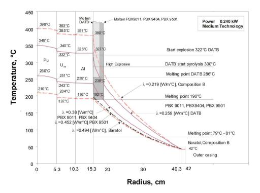
Figure 10.8: Temperature profiles in a medium-technology HNED with an alpha-particle heat power of 0.240 kW.
