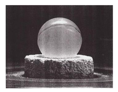
Figure 10.5: A 100 W heat source of about 3 cm diameter containing 250 g of 238-PuO2. The oxide glowed at red heat. It was manufactured by Los Alamos Laboratory, USA for the thermoelectric generators of the Voyager space mission [30].
