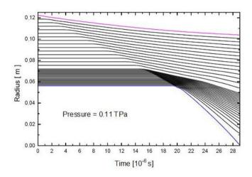
Figure 9.19: The boundaries of each spherical shell as a function of time  $10^{-6}$  s in a hollow plutonium sphere and a natural-uranium reflector. The gradient of the shell boundaries as a function of time represents the particle velocity, u<sub>P</sub>. The outside pressure at the reflector boundary is a constant 0.11 TPa.
