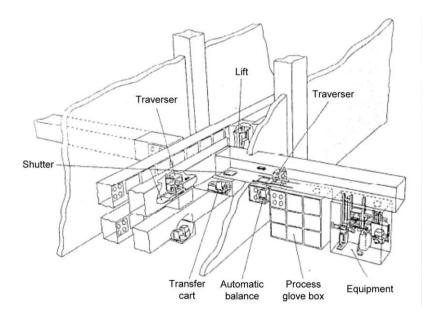
Figure 8.20: Glove box and intermediate storage area. These are connected by automatic transfer machines. During maintenance periods, the nuclear material can be removed from the glove box and placed in the storage area to reduce personnel exposure.
