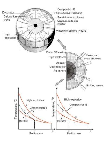
Figure 10.3: Explanation of the conservative one-dimensional approach for an unknown 3-dimensional high explosive lense structure.
