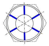
Figure 10.18: Schematic cross-section through a spherical HNED with thermal bridges.
