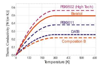
Figure 10.12: Thermal conductivity of chemical high explosives down to cryogenic temperatures.
