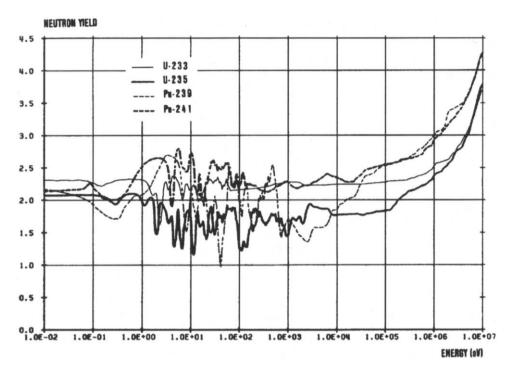
Figure 17.4: Neutron yield as a function of neutron energy for various fissile fuel isotopes [4].
