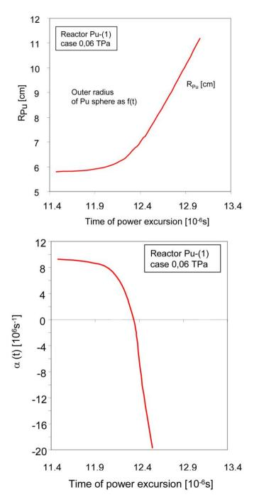
Figure 9.43: Expansion of the outer radius of the Pu-sphere, including internal density changes and the corresponding Rossi alpha change,  $\alpha_{tot}(t) = \alpha_{comp} + \alpha_{expa}$ , for the 0.06 TPa case.
