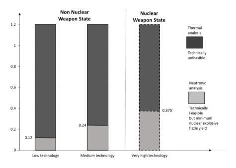
Figure 10.16: Limits for alpha-particle heat power above which HNEDs with reactor-grade plutonium become technically unfeasible for different levels of technology when cooled by air and radiation (Kessler et al. [16]).
