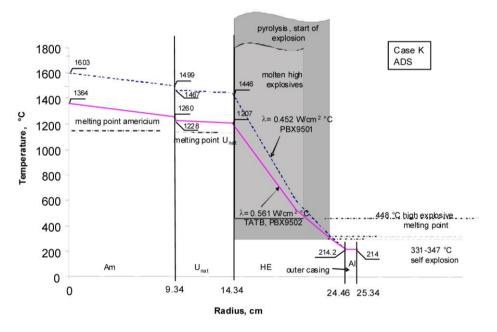
Figure 11.8: Radial temperature profile for a reactor-americium HNED (option K ADS).
