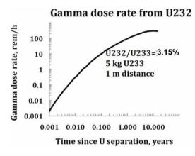
Figure 16.16:  $\gamma$ - dose rate from U-232 (adapted from [20]).
