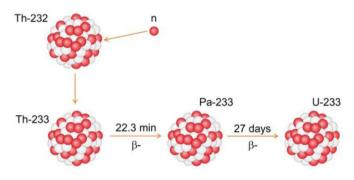
Figure 17.1: Conversion or breeding process of U-233 [1].
