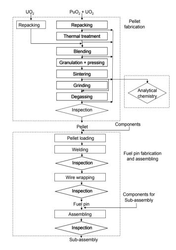
Figure 7.11: Process scheme for the fabrication of MOX elements.
