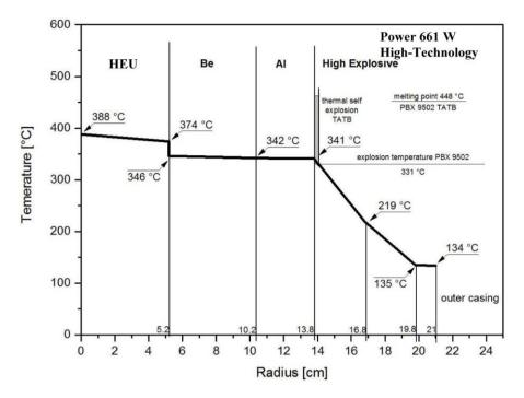
Figure 18.13: Radial temperature profile in a high-technology HNED with an internal  $\alpha$ -heat power of 661 W (fuel type example A).
