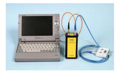
Figure 8.7: Electronic optical sealing system with fibre-optic cable [27,30,34].
