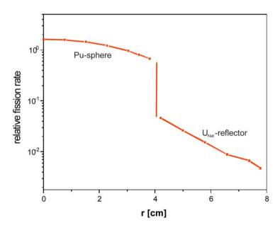
Figure 9.8: Sandmeier example, we apons-grade plutonium, relative fission rate as a function of radius at t = 0.
