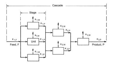
Figure 3.2: Separating unit, stage and cascade [2].
