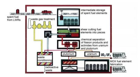
Figure 7.5: Head end with waste gas purification as well as reprocessing of spent fuel and waste conditioning.
