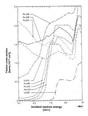
Figure 9.2: Fission neutron cross sections of the principal plutonium and uranium isotopes (and americium-241, decay product of Pu-241) as a function of neutron kinetic energy [19].
