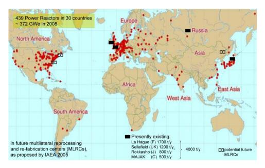
Figure 14.4: Future multilateral reprocessing and refabrication centers (MLRCs) in the world (adapted from IAEA).
