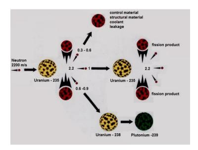
Figure 4.10: Conversion process of U/Pu fuel cycle.
