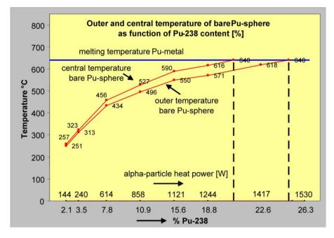
Figure 10.4: Outer and central steady state temperature of a bare metallic Pu-sphere as function of Pu-238 content [%] of reactor-grade plutonium and its alpha heat power.
