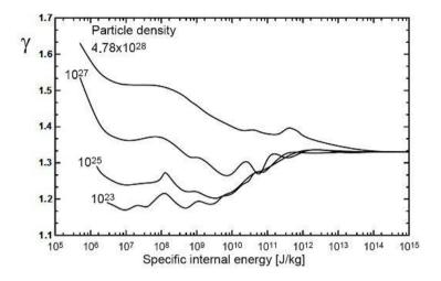
Figure 9.7:  $\gamma = c_p/c_v$  as a function of the specific internal energy E (J/kg) and particle density per (m<sup>3</sup>) uranium [34,51].
