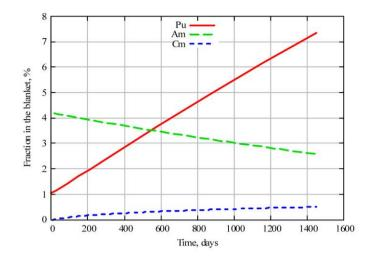
Figure 13.13: Fraction (%) of americium, curium and plutonium in radial blanket fuel elements of BN-600 type FBR (Initial fractions 4.2% reactor americium, 1.08% proliferation-proof plutonium with 11.4% Pu-238) [30].
