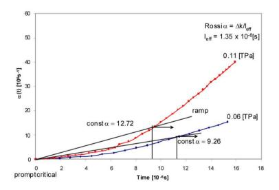
Figure 9.24: Rossi alpha, α(t), for Case A (0.06 TPa) and Case B (0.11 TPa). From prompt criticality to the time when α(t) remains constant, the sigmoidal curve is approximated by a ramp function for pre-ignition analysis.
