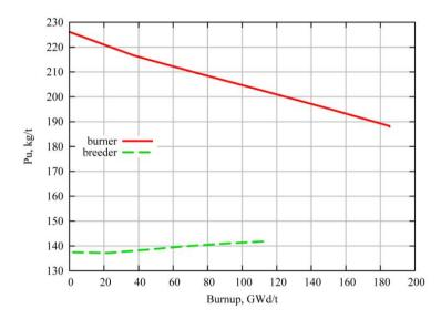
Figure 13.15: Plutonium content per  $t_{HM}$  fuel in the FR burner and in the FR breeder (reactor average) during reactor operation [17].
