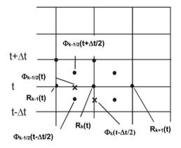
Figure 9.6: Mesh for space and time.
