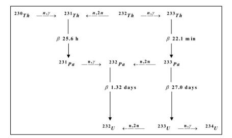
Figure 13.1: Buildup of isotopes in the thorium fuel cycle.
