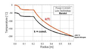
Figure 10.15: Temperature distribution in a low technology HNED with reactor-grade plutonium of 0.240 kW alpha-particle heat power (cooling by liquid nitrogen).
