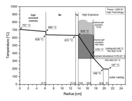
Figure 16.15: Radial temperature profile in the high-technology HNED for an α-heat power of 1,383 W.
