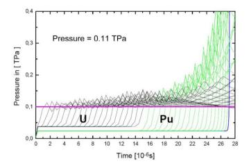
Figure 9.15: Pressures in each spherical shell as a function of time (10<sup>-6</sup> s) in the solid plutonium sphere with a natural-uranium reflector. The outside pressure at the reflector boundary is a constant 0.11 TPa.
