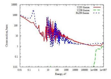
Figure 4.2: Microscopic fission cross section for U-235, U-238 and Pu-239.
