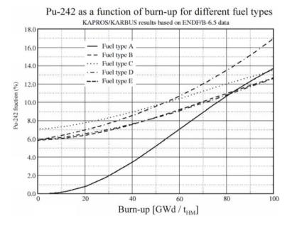
Figure 12.3: Buildup of Pu-242 in wt% for different fuel types.
