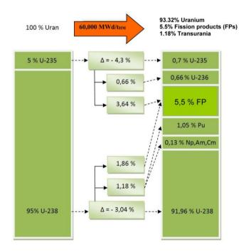
Figure 7.3: Contents (%) of fresh uranium fuel (U-235, U-238) and spent fuel after 60,000 MWd(th)/ton uranium (U-235, U-236, U-238), fission products, plutonium and minor actinides (Np, Am, Cm).
