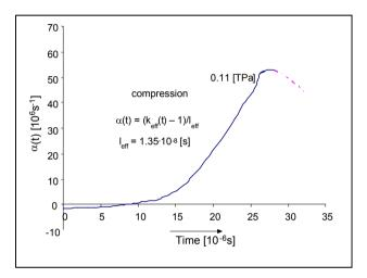
Figure 9.22: Rossi alpha,  $\alpha(t)$ , as a function of time (10<sup>-6</sup> s) for reactor-grade plutonium of the composition Pu-(1) and the pressure of 0.11 TPa ed on the outer surface of the reflector.
