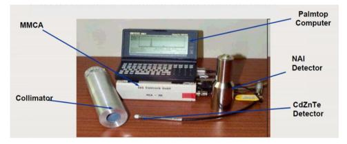
Figure 8.12: Mini-multi-channel analyzer (MMCA) with detectors for fresh fuel assay [4,5].
