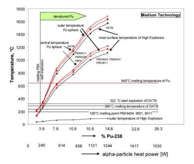
Figure 10.10: Temperature profiles in HNEDs for reactor-grade plutonium for the medium technology case.
