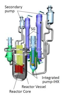
Figure 6.5: 1500 MWe sodium cooled JSFR design proposal (JAEA) [16,17,18,19].
