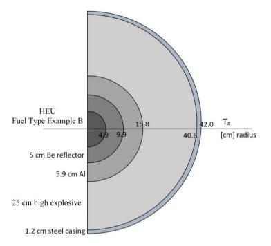
Figure 18.14: Geometric dimensions of a medium-technology HNED with fuel type example B.
