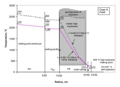
Figure 11.6: Radial temperature profile for a reactor-americium based HNED (option G PWR).
