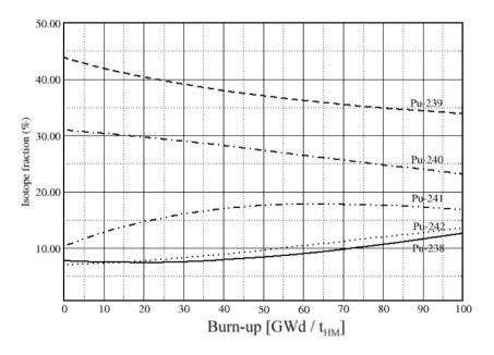
Figure 12.7: Fraction development of plutonium isotopes of denatured plutonium when loaded into PWR core with fuel type C.
