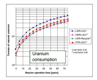
Figure 2.3: Natural uranium consumption (tonnes of natural uranium) for different reactor systems as a function of time.
