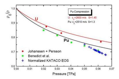
Figure 9.13: Equation of state or compression data for plutonium and uranium metal.
