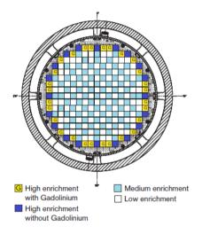
Figure 5.2: Nuclear reactor core of EPR with fuel elements (AREVA).
