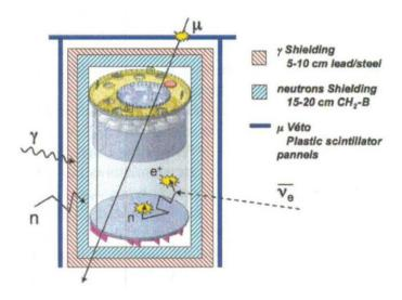
Figure 8.9: Detection principle for anti-neutrinos [37].
