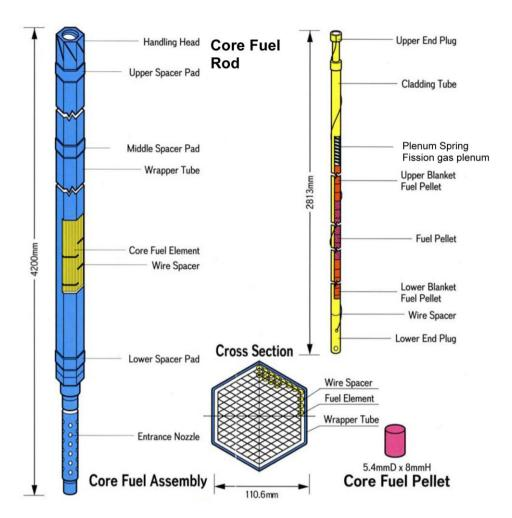
Figure 6.3: Hexagonal core fuel element of the MONJU demonstration FBR [12].
