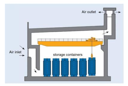
Figure 7.2: Storage of intermediate storage containers in air cooled storage building (VGB).
