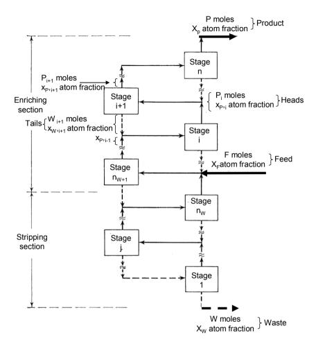
Figure 3.3: Countercurrent recycle cascade [8].
