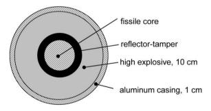
Figure 10.1: Schematic geometric arrangement of HNEDs and dimensions for thermal analyses.
