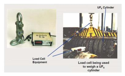
Figure 8.11: UF<sub>6</sub> cylinder containers and IAEA weigh cell (IAEA).
