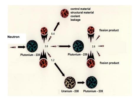
Figure 6.1: Breeding process (U-Pu-cycle).
