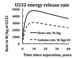
Figure 16.13: Heat rate and γ-radiation rate of U-232 as a function of time after reprocessing according to Moir [20].
