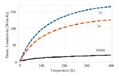
Figure 10.11: Thermal conductivity of aluminum, beryllium and stainless steel SS 304 down to cryogenic temperatures.
