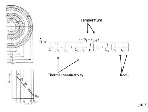
As will be seen below from Table 10.7 as well as already shown in Tables 10.1 through 10.3 the high explosives have the lowest thermal conductivities of all spherical shells without internal heat sources. It is therefore important to have reliable experimental data for the high explosives.
