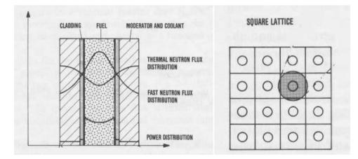
Figure 4.6: Square lattice cell with fuel rod, cladding, and moderator of a LWR-fuel element.
