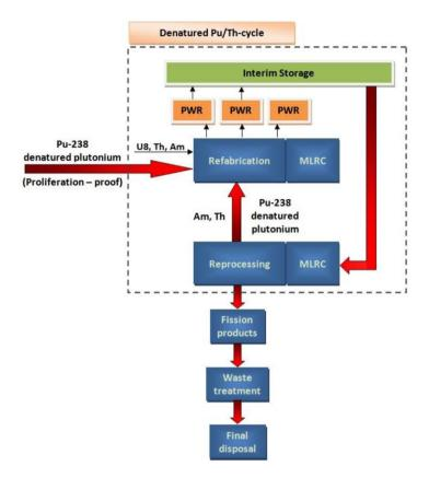
Figure 14.2: Incineration of proliferation-proof plutonium in PWRs in a future civil international proliferationproof fuel cycle. (Reprocessing and Refabrication step will in reality be collocated in one MLRC but shown separately).
