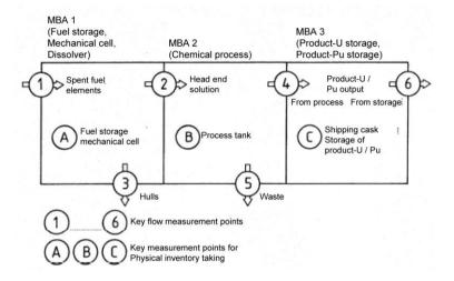
Figure 8.3: Material balance area and key measuring points, e.g. in a reprocessing facility.
