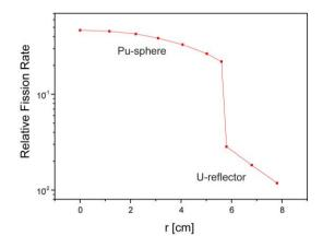
Figure 9.29: Radial distribution of the relative fission rate or power as a function of r at t = 0.
