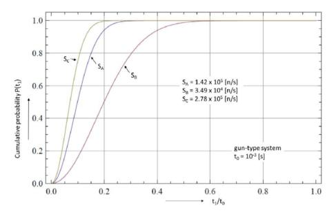
Figure 18.4: Cumulative probability of pre-ignition for a time period of  $t_0=10^{-3}$  s of compaction by gun-type system as a function of  $t_1/t_0$ . Spontaneous and  $(\alpha, n)$ -neutron sources  $S_A$ ,  $S_B$ , and  $S_C$
