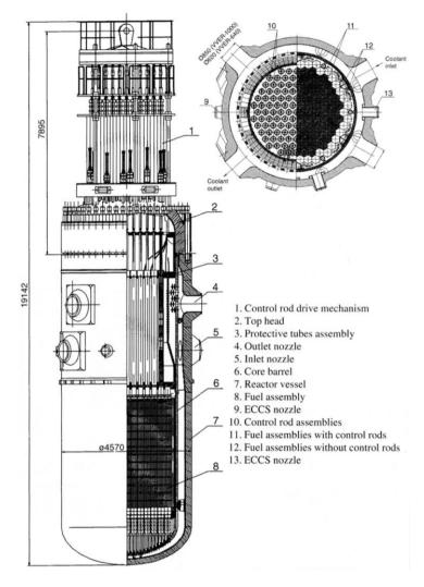
Figure 5.7: Cross section view of Russian VVER reactor pressure vessel with core and control rod drive mechanics [6].
