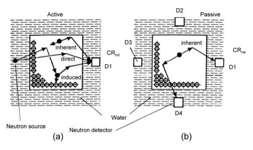
Figure 8.15: Principle of the method of active and passive neutron interrogation [6].
