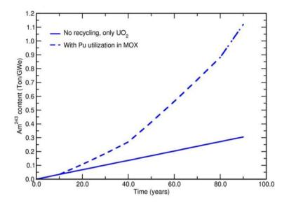
Figure 7.16: Amount of americium generated by a cluster of M = 8 UOX PWRs (full line). Amount of americium generated by a cluster of M = 8 UOX and MOX PWRs (dotted line) operating in the SGR mode. Amounts are normalized to 1 GWe [28].
