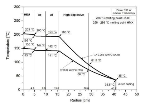
Figure 18.15: Radial temperature in a medium-technology HNED and fuel type example B with an  $\alpha$ -heat power of 133 W and DATB and HMX as high explosives.
