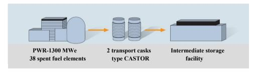
Figure 7.1: Transport of spent fuel elements from reactor to intermediate storage (VGB).
