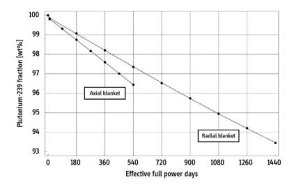
Figure 13.12: Plutonium-239 fraction of the plutonium produced in the Indian Prototype Fast Breeder Reactor (PFBR) as a function of irradiation time in the axial or radial blanket fuel elements [27].
