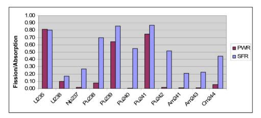
Figure 13.8: Impact of energy spectrum on incineration and transmutation performance [26].
