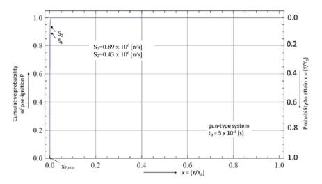
Figure 16.10: Cumulative probability of pre-ignition as a function of the ratio x of the attainable nuclear explosive yield Y to the maximum nominal yield  $Y_o$  for the time period of compaction  $t_0 = 5 \times 10^{-4}$  s. Spontaneous fission neutron source  $S_1=0.89 \times 10^6$  n/s and  $S_2=0.43 \times 10^6$  n/s.
