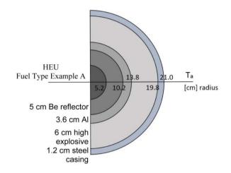
Figure 18.12: Geometric dimensions for a high-technology HNED with fuel type examples A and C.
