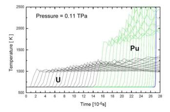
Figure 9.18: Temperature (K) in the different spherical shells as a function of time  $(10^{-6} \text{ s})$  in a solid plutonium sphere with a natural-uranium reflector. The outside pressure at the reflector boundary is a constant 0.11 TPa.
