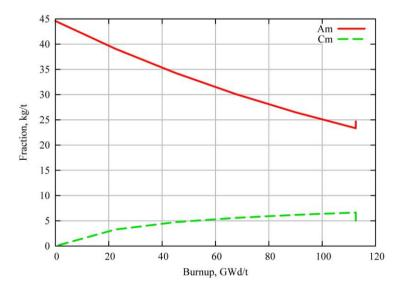
Figure 13.17: Am and Cm content in the breeder during reactor operation [17].
