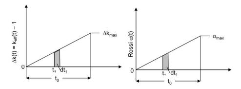
Figure 9.23: (a)  $\Delta k(t)$  as a ramp function of time, t<sub>1</sub>, starting from prompt criticality, (b) Rossi  $\alpha(t)$  as a ramp function of time, t<sub>1</sub>, starting from prompt criticality.
