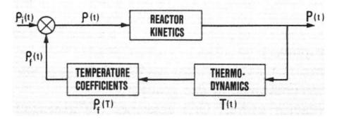
Figure 4.13: Schematic of the reactor dynamics feedback loop.
