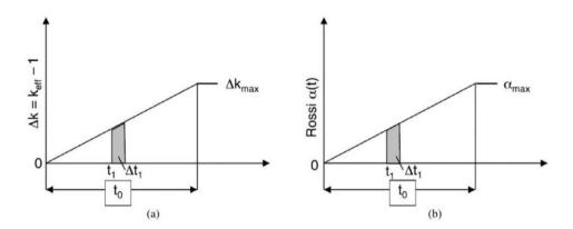
Figure 16.6: Fig. 16.6: (a)  $\Delta k(t)$  as a ramp function of time  $t_1$  and (b) Rossi  $\alpha(t)$  as a ramp function of time  $t_1$ .
