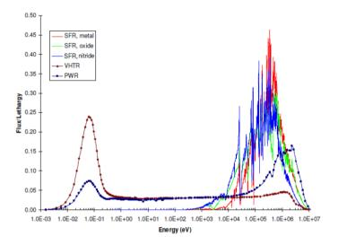
Figure 4.4: Neutron energy distribution (spectrum) in a PWR and VHTR and FRs [36].
