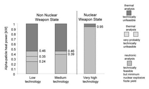
Figure 10.17: Limits for alpha-particle heat power above which HNEDs with reactor grade plutonium become technically unfeasible for different levels of technology and cooling at the outside by liquid helium (Kessler [16]).
