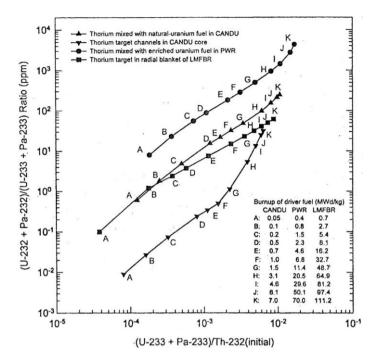
Figure 18.1: (U-232+Pa-232)/(U-233+Pa-233) ratio as a function of (U-233+Pa-233)/Th-232 ratio in different reactor types (CANDU, PWR and LMBFR) [1].
