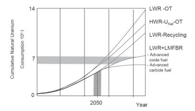
Figure 2.4: General projection of natural uranium consumption for different reactor types including fast neutron spectrum breeder reactors.
