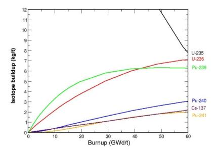
Figure 4.8a: Isotope concentrations for U-235, U-236, Pu-239, Pu-240, Pu-241 and Cs-137 as a function of burnup [GWd/to] of LWR fuel. Initial fuel enrichment: 5% U-235 [32].
