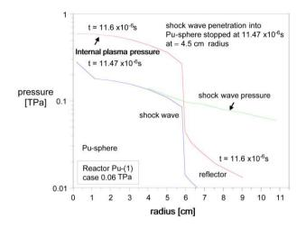
Figure 9.30: Dependence on time and space of shock wave pressure and internal plasma pressure for the 0.06 TPa case.
