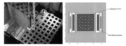
Figure 8.14: FORK detector and partially lifted fuel element.
