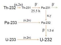
Figure 16.2: Production routes of U-232 via  $(n,\gamma)$  and (n,2n)-reactions [22] (adapted).
