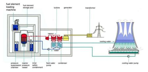
Figure 5.8: Main design principle of the boiling water reactor SWR-1000 (AREVA).
