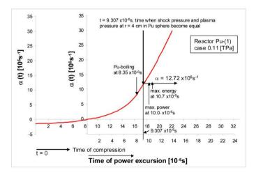
Figure 9.32: Dependence on time of Rossi alpha,  $\alpha(t)$ , after compression or after transition through prompt criticality (0.11 TPa case).
