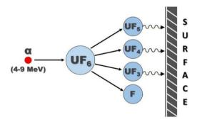
Figure 16.4: Destruction of UF<sub>6</sub> by  $\alpha$ -particles.
