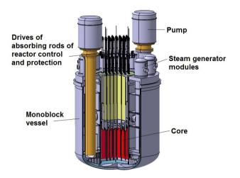
Figure 6.6: SVBR-75/100 reactor design [29,30].
