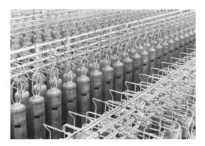
Figure 8.10: Centrifuge cascade hall of a gas centrifuge enrichment plant (URANIT).
