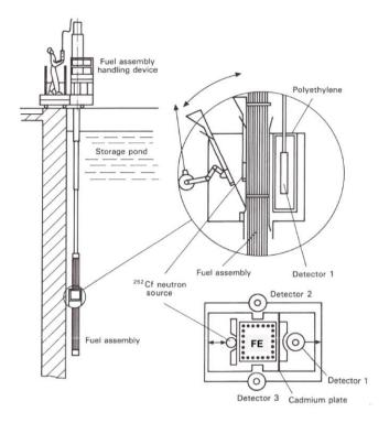
Figure 8.16: Arrangement of LWR fuel element and Cf-252 neutron source.
