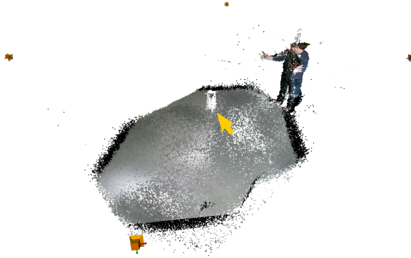
Figure 5.3.: 3D point cloud, combined from the data of the four Kinects in Figure 5.1 and Figure 5.2.
