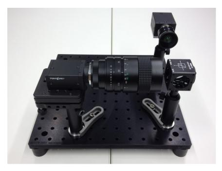
Figure 2.3: Prototype of the proposed system for capturing ground truth SR data
