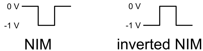
Figure C.41: Sketch of a NIM-pulse and an inverted NIM-pulse.
