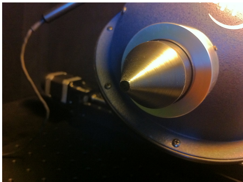
Figure B.5: Photograph of the PVC-collimator ColA mounted on the integrating sphere.
