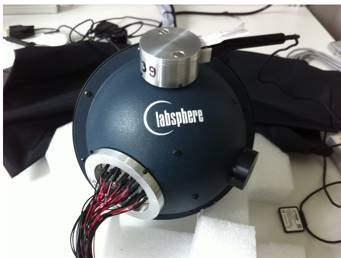
Figure B.3: Photograph of the set-up for the position dependent flux measurements. Here LED-array AR2 ( entrance ) and a photodiode ( top ), with its respective mount, are attached to the sphere. The second exit port ( side ) is closed with a lid coated with Spectralon.
