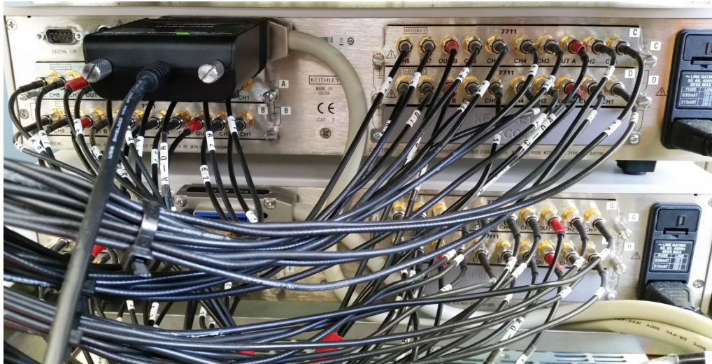
Figure B.8: View of the back side of the two Keithley 2750 frames with each four Keithley 7711 multiplexer cards.
