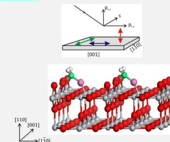
The dioxymethylene (DOM) is detected as a minority species formed via reaction of Ti<sub>5c</sub>-bound CH<sub>2</sub>O with adjacent O<sub>br</sub> along the [1-10] direction.
