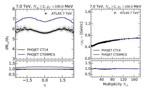
Figure 7.8: Effect due to the change of PDF on charged particle minimum-bias distributions in PHOJET using a tune for CT14. The CT09MCS distributions are generated with parameters of the CT14 tune. Measurements performed by ATLAS [3].
