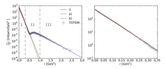
Figure 6.7: Fits and interpolations compared to the combined EPL95 and EPL96 TOTEM data. *i*) is the result of interpolation, *a*) the exponential fit with a curvature parameter and *b*) a simple gaussian fit using the  $B_0(t = 0)$  value from EPL96. The right pane enlarges the small *t* region.
