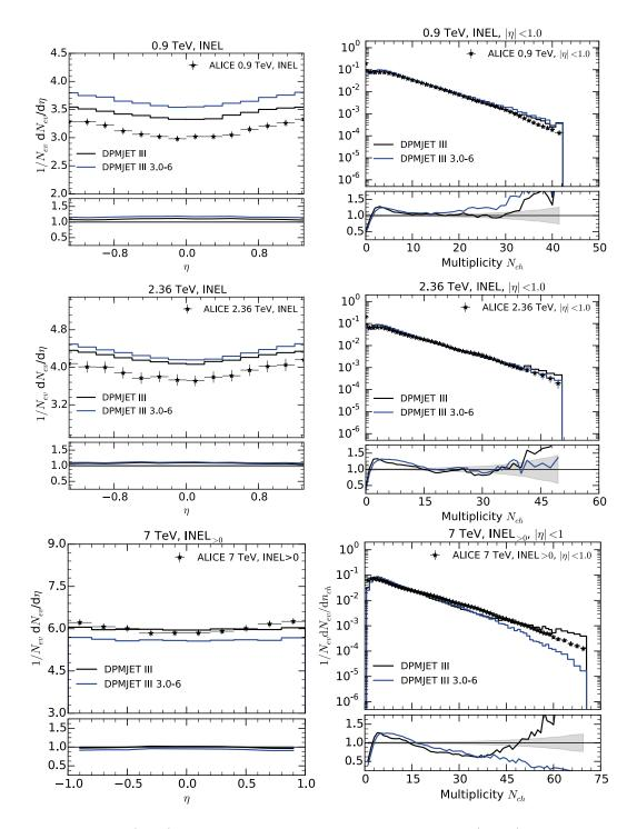
Figure 7.18: (Left) Charged-particle pseudo-rapidity and (right) multiplicity distributions for the INEL(astic) event selection. This measurement is for  $p_T > 0$  MeV by ALICE [6, 5].
