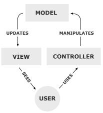
Figure 4.1: Model-view-controller pattern
