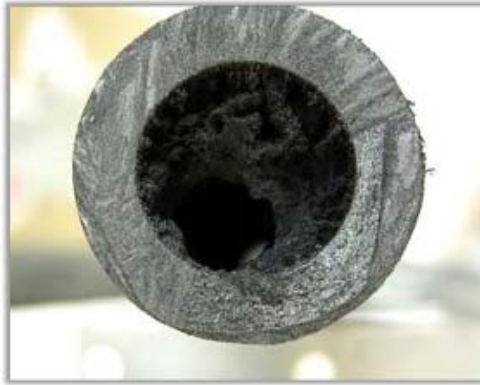
Fig. 4 - Carbon clogging in a tubular experimental reactor [14].
