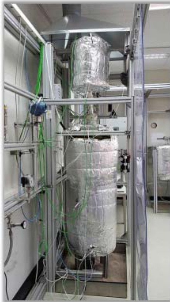
Fig. 7 - Photograph of the methane cracking experimental facility at KIT showing the insulated liquid metal reactor in the bottom.
