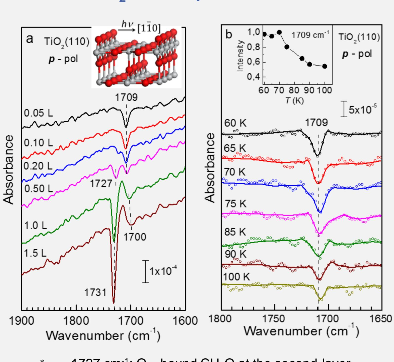
$\text{CH}_2\text{O}$  polymerization at the  $\text{Ti}_{5c}$  rows
