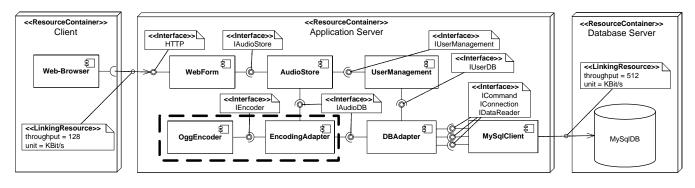
Figure 8: The software architecture of the MediaStore [6]
