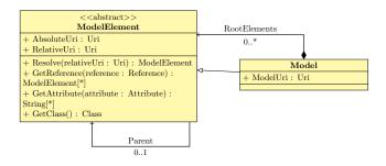
Figure 2: The base metaclasses in NMeta
