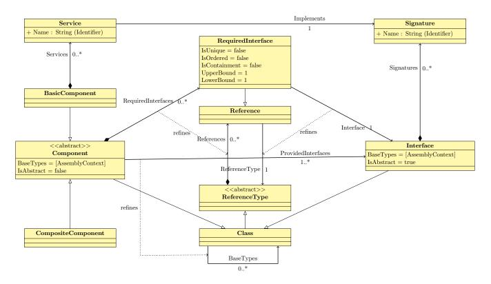
Figure 5: Component types in DeepADL
