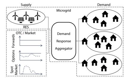
Figure 8.1: Integration of a flexibility aggregator into a microgrid with supply from RES, forwards, options and the spot market and demand consisting of household cooperatives which consume base, shiftable, and curtailable load on the demand side
