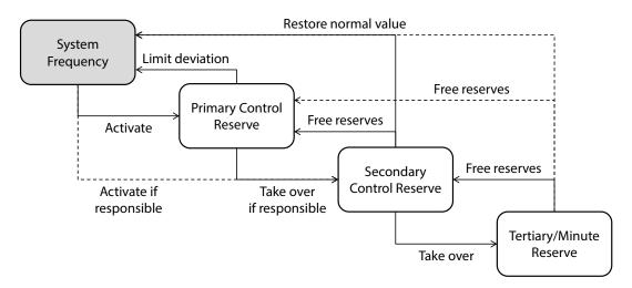
Figure 2.7: Reserve power activation, adapted from Entsoe (2004)
