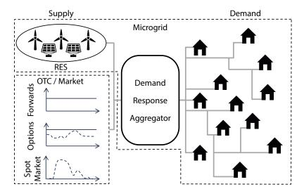
Figure 6.1: Illustration of supply and demand abstraction level in a local microgrid scenario with supply from RES, forwards, options and the spot market considering single households which consume base, shiftable, and curtailable load on the demand side
