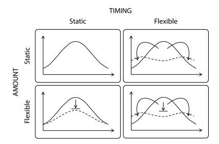
Figure 2.11: Demand response type characterization, adapted from Flath (2013)
