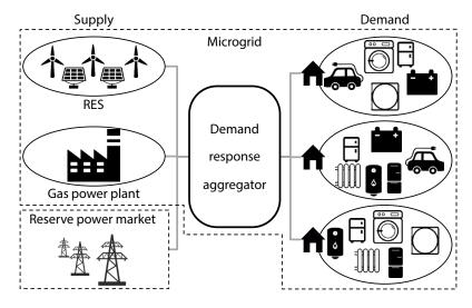
Figure 4.1: Integration of the demand response aggregator into the local microgrid scenario with supply from RES, a gas turbine, and reserve power considering single devices' flexibility
