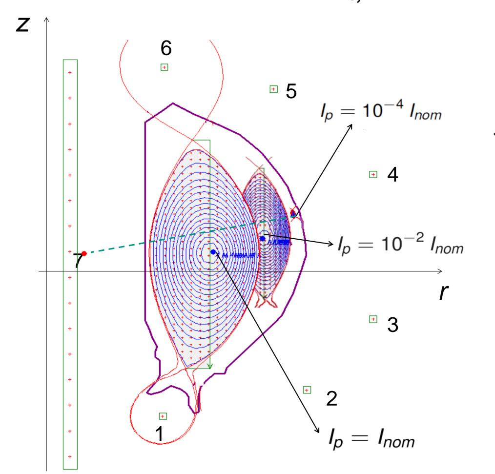
$$\begin{cases} B_{s}(\boldsymbol{p_{x}}(t_{i})) = \sum_{k} G_{s,k}(\boldsymbol{p_{x}}(t_{i}))I^{(k)} = 0 \\ \sum_{k} I^{(k)} = -I_{p}(t_{i}) \\ I_{p}(t_{i} = \tau_{RU}) = I_{nom} \end{cases}$$
