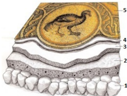
Fig. 1: Graphic reproduction of mosaic stratigraphy adapted from ancient literary. 1) Statumen - Layer which is made of large stones laid on the ground. This layer only exists if the mosaic has been constructed on a natural soil. 2) Rudus - Layer which is spread over the statumen . This layer is made of a lime mortar with large aggregates. 3) Nucleus - Layer which is spread over the rudus in a thinner layer. The nucleus is made of a mortar with fine aggregates. 4) Bedding layer - Layer of mortar which is very rich in lime, and thinly applied in small sections over the nucleus . Tesserae are inserted in this layer before the mortar sets. 5) Tessellatum - Layer which constitutes the mosaic surface and is composed of tesserae and mortar filling the interstices between them [13].
