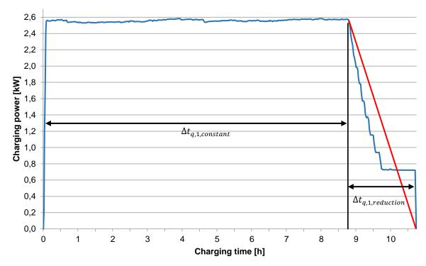
Figure 3: Recorded charging curve of project EV (e-Wolf Delta 2) at domestic power outlet
