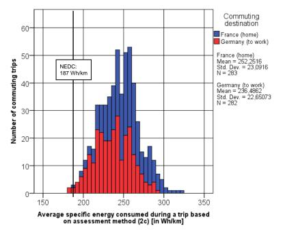
Figure 5: Distributions of the specific energy consumed (measurement point 3, Figure 2) during the binational commuting trips by the 3 project EV
