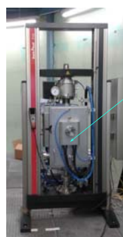
Test section 1: universal traction facility
