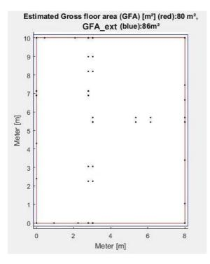
Figure 5-7: Gross floor area of the four-room apartment (case study 1), blue: outer envelopment, red inner envelopment
