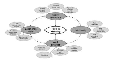
Figure 2-6: Overview on project management parameters for deconstruction projects<sup>26</sup>
