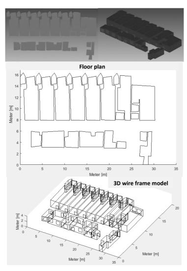
Figure 5-31: Case study 2 with floor plan and reconstructed 3D model based on sensor data in the processing tool (top) and in the developed model (bottom) (center: floor plan; bottom: 3D view in isometric projection<sup>14</sup>)
