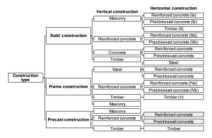
Figure 2-1: Typology of residential and non-residential buildings with regard to their type of construction<sup>2</sup>
