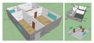
Figure 5-1: Google SketchUp model view in three different perspectives of the exemplary four-room apartment (case study 1) and its building elements (IDs)
