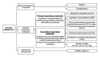
Figure 2-2: Classification of main hazardous and interfering substances/materials in building elements<sup>5</sup>
