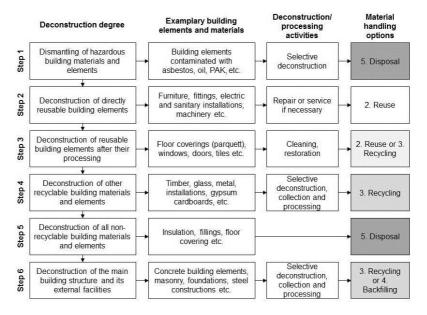
Figure 2-7: Deconstruction degrees, exemplary building elements and materials, resulting deconstruction and processing activities and material handling options (no.)<sup>36</sup>
