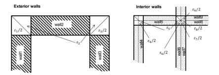
Figure 4-6: Schematic cutaway floor plan of exterior and interior walls and correction factor  $\varepsilon$  in exterior (left) and in interior (right) wall volume calculation
