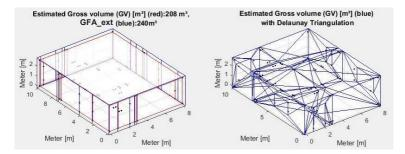
Figure 5-8: Gross volume of the four-room apartment (case study 1), blue: outer envelopment, red inner envelopment
