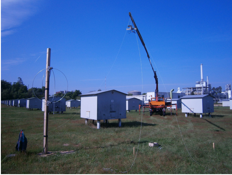
Figure 2: Setup of the Tunka-Rex antenna calibration in Karlsruhe. A crane holds a reference source above the antenna aligned from the ground using strings. With the known emitted field strength of the reference source, the characteristics of the SALLA can be determined.
