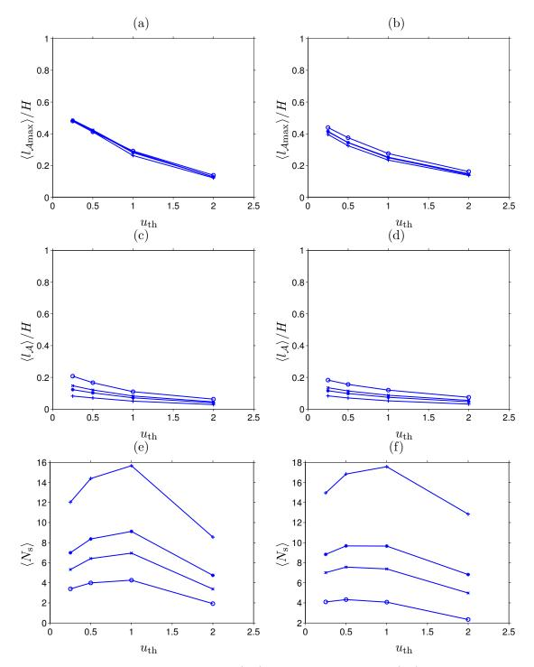
FIGURE 3.20: Ensemble average of: (a,b) maximum length-scale; (c,d) length-scale; (e,f) number of velocity streaks per cross-section as a function of threshold velocity  $u_{\rm th}$ . (a,c,e) high-velocity streaks; (b,d,f) low-velocity streaks. Symbols indicate different Reynolds numbers:  $\circ$ ,  $Re_b = 1450$ ;  $\times$ ,  $Re_b = 2205$ ; \*,  $Re_b = 3000$ ; +,  $Re_b = 5000$ .
