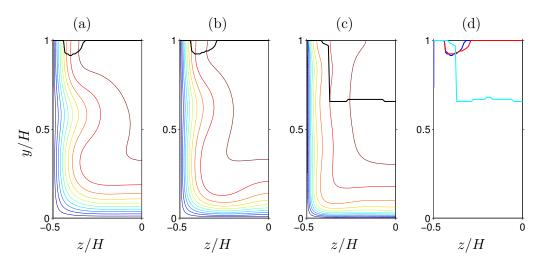
FIGURE 4.35: Mean streamwise velocity contour with the location of the maximum velocity as function of z/H (black solid line). (a)  $Re_b = 2205$ , (b)  $Re_b = 3000$ , (c)  $Re_b = 5000$ . A = 0.5. (d) Summary of the the location of the maximum velocity for all Reynolds numbers, whose colours of the solid lines indicate different Reynolds number where: blue,  $Re_b = 2205$ ; red,  $Re_b = 3000$ ; cyan,  $Re_b = 5000$ .
