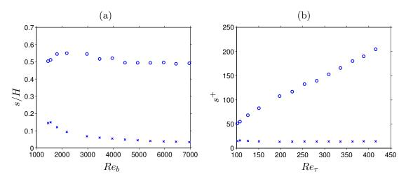
FIGURE 3.12: Positions of extrema of  $\langle \omega_x \rangle(y,z)$  of outer secondary vorticity cell in: (a) external coordinates vs.  $Re_b$  and (b) wall coordinates vs.  $Re_{\tau}$ . Symbols:  $\circ$  distance to z/H = -A;  $\times$  distance to y/H = 1.
