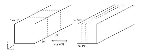
FIGURE 2.2: "Slice" data decomposition strategy used for parallelisation of the pseudospectral DNS code. This figure is from Sakai and Uhlmann (2016).
