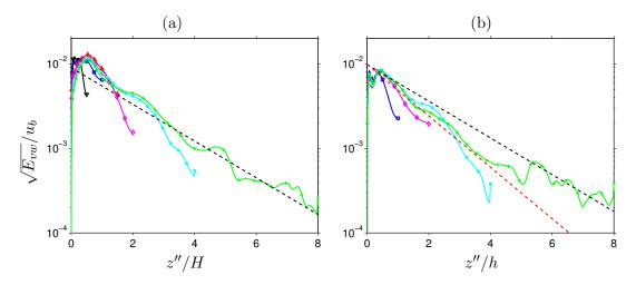
FIGURE 4.28: Spanwise distribution of secondary flow energy  $E_{vw} = \frac{1}{2} \int_0^H (\langle v \rangle^2 + \langle w \rangle^2) dy$  as a function of distance from side-wall z''/H = (AH - |z|)/H, of (a) open and (b) closed duct flow. Reynolds number is fixed at  $Re_b = 2205$  and coloured symbol code is as of Figure 4.19. Black dashed lines indicate  $\approx \exp(-0.5z''/H)$ , whereas red line in (b) indicates  $\approx \exp(-0.7z''/h)$ .
