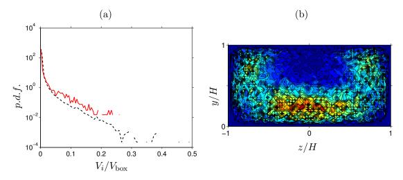
FIGURE 5.9: (a) Probability density function of the tracked vortex volume normalised by the numerical box volume  $V_{\text{box}}$ . Different coloured lines indicate: red solid, vortex connections with single vortex; black dashed, vortex connections with more than one vortices. (b) Probability density function of the centroid locations of the vortex trajectories with the length equals to unity.
