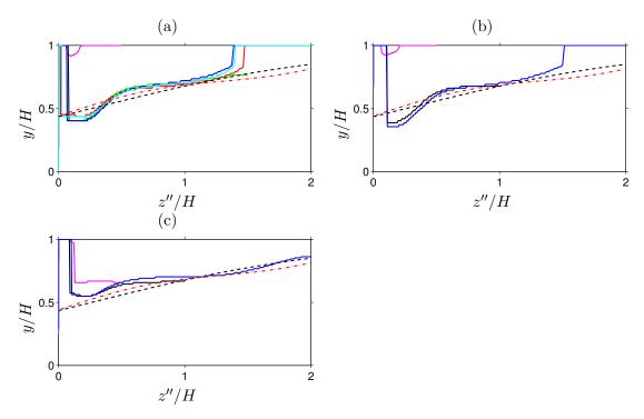
FIGURE 4.40: Locations of the maximum mean streamwise velocity as function of z''/H = (AH - |z|)/H (black solid line). (a)  $Re_b = 2205$ , (b)  $Re_b = 3000$ , (c)  $Re_b = 5000$ . Colours of the solid lines represent different aspect ratio: magenta, A = 0.5; black, A = 1; blue, A = 1; green, A = 1.5; blue, A = 2; cyan, A = 4; red, A = 8. Red dotted dash and black dashed lines indicate the predicted values by the models of Wang et al. (2001) and Yang et al. (2004) respectively.
