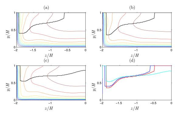
FIGURE 4.37: Mean streamwise velocity contour with the location of the maximum velocity as function of z/H (black solid line). (a)  $Re_b = 2205$ , (b)  $Re_b = 3000$ , (c)  $Re_b = 5000$ . A = 2. (d) Summary of the the location of the maximum velocity for all Reynolds numbers, whose colours of the solid lines indicate different Reynolds number where: blue,  $Re_b = 2205$ ; red,  $Re_b = 3000$ ; cyan,  $Re_b = 5000$ .
