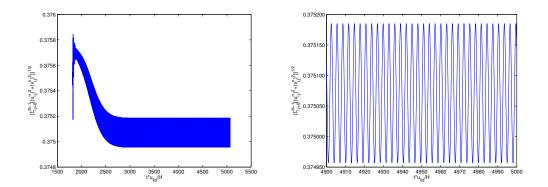
FIGURE E.14: Evolution of E for the regularised cavity at Re = 10500 starting from the steady-state solution of Re = 10000. Computed by 4th-order scheme. Oscillation period  $T \approx 3$
