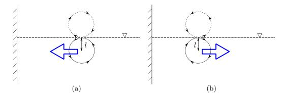
FIGURE 3.14: Conceptual sketch of mixed-boundary vortex dynamics. Dashed-line vortex represents the mirror image generated by free-slip boundary in order to satisfy impermeability constrain. Blue arrow indicates the induced motion due to the vortex dipole effect. Vortex with the sense of rotation corresponding to: (a) mean inner secondary vorticity cell; (b) outer secondary vorticity cell.
