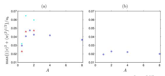
FIGURE 4.30: Intensities of maximum mean secondary velocity  $\max\{(\langle v \rangle^2 + \langle w \rangle^2)^{1/2}\}$ as function of aspect ratio A, of (a) open and (b) closed duct flow. Coloured symbols indicate different bulk Reynolds number  $Re_b$ :  $\circ$ ,  $Re_b = 2205$ ;  $\triangle$ ,  $Re_b = 3000$ ; \*,  $Re_b = 5000$ .
