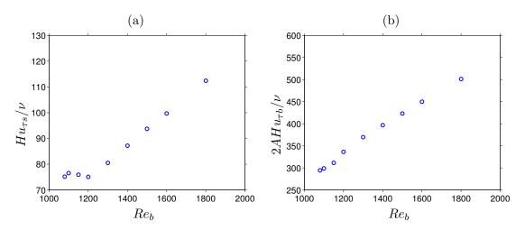
FIGURE 4.14: (a) Duct full-height H and (b) full-span as a function of bulk Reynolds number  $Re_b$ , normalised by the side-wall and bottom-wall friction length respectively. Open duct flow with A = 2.
