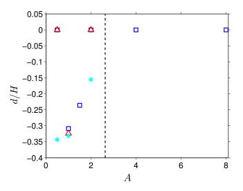
FIGURE 4.39: Submerged distance d from the free-slip plane y/H = 1 to the location of the maximum mean streamwise velocity  $\langle u \rangle$  along the duct mid-span z/H. The distances are normalised by H and express as function of aspect ratio A. Coloured symbols indicate different bulk Reynolds number  $Re_b$ :  $\Box$ ,  $Re_b = 2205$ ;  $\triangle$ ,  $Re_b = 3000$ ; \*,  $Re_b = 5000$ . Black dashed line indicates the critical aspect ratio  $A_c = 2.5$  suggested by Nezu and Rodi (1985).
