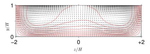
FIGURE 4.10: Mean secondary flow vector and mean streamwise velocity contour of open duct flow with A = 2 and  $Re_b = 1080$ . Red contour lines indicate 0.1(0.1)0.9 times the maximum value of the mean streamwise velocity  $\langle u \rangle$ .
