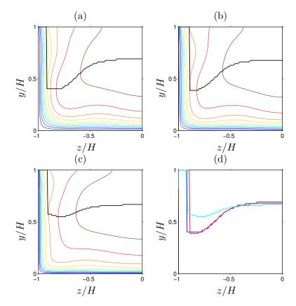
FIGURE 4.36: Mean streamwise velocity contour with the location of the maximum velocity as function of z/H (black solid line). (a)  $Re_b = 2205$ , (b)  $Re_b = 3000$ , (c)  $Re_b = 5000$ . A = 1. (d) Summary of the the location of the maximum velocity for all Reynolds numbers, whose colours of the solid lines indicate different Reynolds number where: blue,  $Re_b = 2205$ ; red,  $Re_b = 3000$ ; cyan,  $Re_b = 5000$ .
