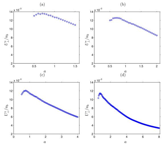
FIGURE 4.31: Side-wall secondary flow intensity dependence to side-wall coefficient a, for different aspect ratio A: (a) A = 1.5; (b) A = 2; (c) A = 4; (d) A = 8. Open duct flow with a fixed bulk Reynolds number at  $Re_b = 2205$ .
