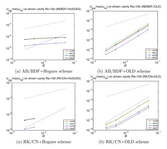
FIGURE C.5: Temporal convergence of  $L_2$ -error in slip-velocity normalised by the maximum lid velocity. "north", "east", "south" and "west" indicate individual walls, while red and blue bashed lines represent 1st and 2nd order temporal convergence. Used time-integration schemes are (a,b) AB/BDF; (c,d) RK/CN. (c) RK/CN has two less data points since the simulations diverged with those dt values.  $M_x = 3$ ,  $M_y = M_z = 33$ . (FORTRAN)
