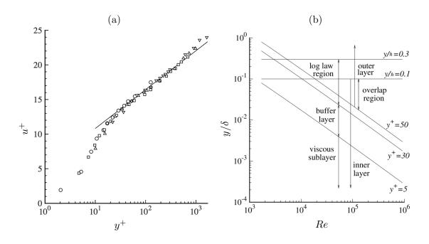
FIGURE 1.6: (a) Mean velocity profiles in fully developed turbulent channel flow by Wei and Willmarth (1989), with a range of Reynolds numbers  $Re_0 =$ [2970, 14914, 22776, 39582]. (b) Wall-distance in outer scales of the different regions in turbulent wall-bounded flow as a function of the Reynolds number. Both figures are from Pope (2000).
