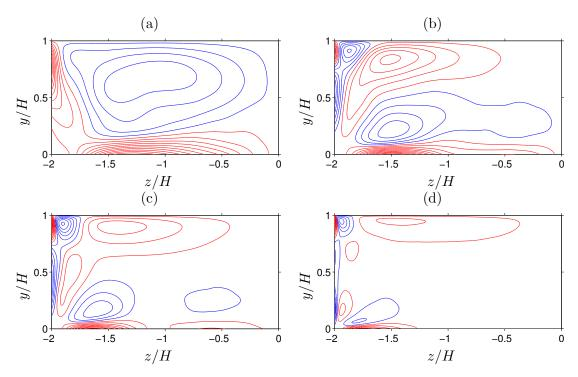
FIGURE 4.11: Contours of ⟨ω<sub>x</sub>⟩(y, z) of mean secondary flow computed using ⟨v⟩ and ⟨w⟩ with reflective symmetry about duct mid-span (with increment [max⟨ω<sub>x</sub>⟩ - min⟨ω<sub>x</sub>⟩]/20). Red lines correspond to positive values and blue lines to negative ones.
