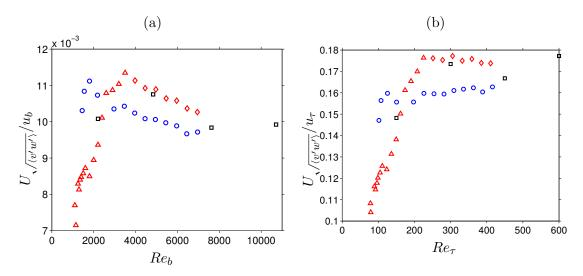
FIGURE 3.17: Intensities of cross-plane averaged cross-correlation velocity  $U_{\sqrt{\langle v'w'\rangle}} = \left[\frac{1}{2AH^2}\int_{-AH}^{+AH}\int_0^H |\langle v'w'\rangle| dydz\right]^{1/2}$ . The values are normalised by: (a)  $u_b$  and vs.  $Re_b$ ; (b)  $u_\tau$  and vs.  $Re_\tau$ . Symbols indicate:  $\circ$ , open duct of current study;  $\triangle$ , closed duct of Pinelli et al. (2010);  $\diamond$ , closed duct of current study;  $\Box$ , closed duct of Zhang et al. (2015).
