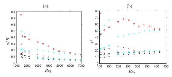
FIGURE 3.11: Positions of extrema of  $\langle \omega_x \rangle(y,z)$ : (a) external coordinates vs.  $Re_b$ and (b) wall coordinates vs.  $Re_{\tau}$ . Colours: black, inner secondary vorticity cell; red, bottom-wall vorticity cell; cyan, side-wall vorticity cell. Symbols:  $\circ$  distance to z/H =-A;  $\times$  distance to y/H = 1 (black symbols) and y/H = 0 (red and cyan symbols).
