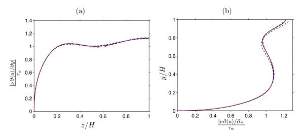
FIGURE A.1: Grid-convergence study in terms of wall shear stress distribution  $\nu \partial \langle u \rangle / \partial n$  along: (a) duct bottom-wall, (b) side-wall. Lines indicate: black solid,  $[M_x, M_y, M_z] = [256, 97, 193]$  (averaged over 12940  $u_b/H$ ); blue dashed,  $[M_x, M_y, M_z] = [192, 65, 129]$  (4580  $u_b/H$ ); red dotted dash,  $[M_x, M_y, M_z] = [384, 129, 257]$  (2674  $u_b/H$ ) respectively.
