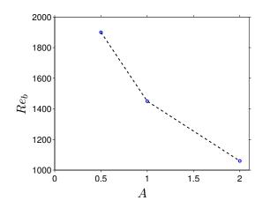
FIGURE 4.17: Minimal sustainable bulk Reynolds number as function of a spect ratio A.
