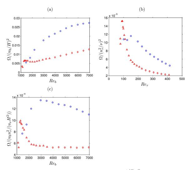
FIGURE 3.18: Cross-section averaged Enstrophy  $\Omega = \frac{1}{2AH^2} \int_{-AH}^{+AH} \int_{0}^{H} (\langle \omega_x \rangle^2 / 2) \, dy \, dz$ normalised by (a) bulk units  $(u_b/H)^2$ ; (b) wall units  $(u_\tau^2/\nu)^2$ ; (c) mixed units  $(u_b u_\tau^2/(u_\nu H^2))$ . Symbols indicate:  $\circ$ , open duct of current study;  $\Delta$ , closed duct of Pinelli et al. (2010);  $\diamond$ , closed duct of current study.
