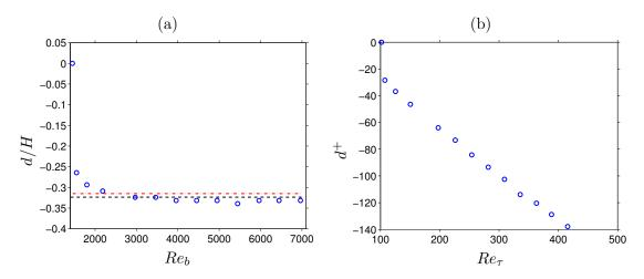
FIGURE 3.19: (a,b) Submerged distances d from the free-slip plane y/H = 1 to the location of the maximum mean streamwise velocity  $\langle u \rangle$  along the duct mid-span z/H = 0, respectively in: (a) external coordinates vs.  $Re_b$  and (b) wall coordinates vs.  $Re_{\tau}$ . Red dotted dash and black dashed lines indicate the predicted values by the models of Wang et al. (2001) and Yang et al. (2004) respectively.
