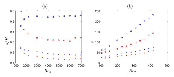
FIGURE 3.8: Positions of extrema of  $\langle \psi \rangle (y, z)$ : (a) external coordinates vs.  $Re_b$  and (b) wall coordinates vs.  $Re_{\tau}$ . Colours: blue, outer secondary flow cell; red, bottom-wall cell. Symbols:  $\circ$  distance to z/H = -A;  $\times$  distance to y/H = 1 (blue symbols) and y/H = 0 (red symbols).
