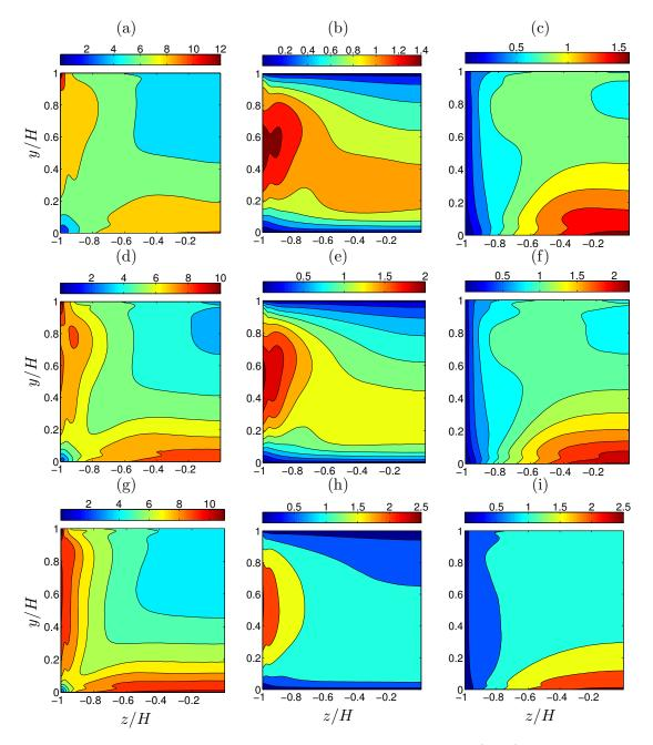
FIGURE A.3: Ratio of the grid spacing  $\Delta x_i$  to the local  $\eta$ , in: (a,d,g) streamwise; (b,e,h) wall-normal; (c,f,i) spanwise direction. (a-c)  $Re_b = 2205$ ; (d-f)  $Re_b = 3000$ ; (g-i)  $Re_b = 5000$ .
