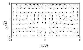
FIGURE 5.16: Mean cross-plane vortex advection velocity vectors, computed from  $\langle v_{\rm v} \rangle$ and  $\langle w_{\rm v} \rangle$ .
