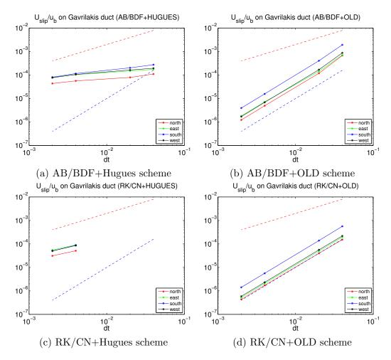
FIGURE C.6: Temporal convergence of  $L_2$ -error in slip-velocity normalised by bulk velocity. "north", "east", "south" and "west" indicate individual walls, while red and blue bashed lines represent 1st and 2nd order temporal convergence. Used time-integration schemes are: (a,b) AB/BDF (c,d) RK/CN. (c) RK/CN+HUGUES has two less data points since the simulations diverged with those dt values.  $M_x = 256$ ,  $M_y = M_z = 97$ . (FORTRAN)
