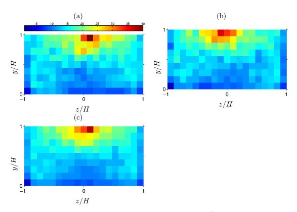
FIGURE 5.10: Spatial distribution of averaged vortex lifetime  $\langle \tilde{T}_i \rangle$  normalised by viscous time unit  $\nu/u_{\tau}^2$ . (a) Vortex with *positive*  $\omega_x$ ; (b) *negative*  $\omega_x$ ; (c) average of (a) and (b). The vortex lifetime was associated with every terminal centroid locations of the tracked vortices. The statistics were then averaged over square boxes enclosed by 10-by-20 equidistant grid points (not C-G-L points).
