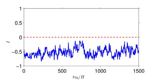
FIGURE 4.6: Temporal evolution of the indicator function I of the open duct simulation with  $Re_b = 1900$  and A = 0.5. Red dashed line indicates I = 0.
