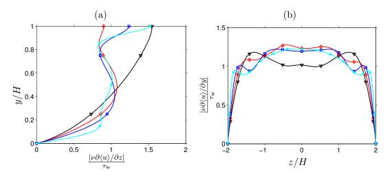
FIGURE 4.8: Mean wall stress of open duct flow with A = 2, distributions along: (a) side-wall and (b) bottom-wall, normalised by the whole no-slip wall average value  $\tau_{\rm w}$ . Coloured symbols indicate the value of the bulk Reynolds numbers:  $\bigtriangledown$ ,  $Re_b = 1080$ ;  $\triangle$ ,  $Re_b = 1900$ ;  $\Box$ ,  $Re_b = 2205$ ; \*,  $Re_b = 5000$ .
