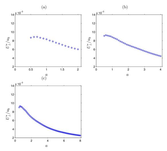
FIGURE 4.32: Side-wall secondary flow intensity dependence to side-wall distance coefficient *a*, for different aspect ratio *A*: (a) A = 2; (b) A = 4; (c) A = 8. Closed duct flow with a fixed bulk Reynolds number at  $Re_b = 2205$ .
