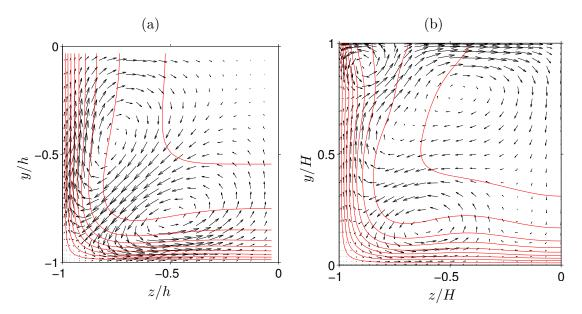
FIGURE 1.2: Mean secondary flow vector and mean streamwise velocity contour of: (a) closed and (b) open duct flow at  $Re_b = 2205$ . Only lower left quadrant and left half of the duct cross planes are shown respectively.
