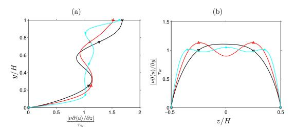
FIGURE 4.3: Mean wall stress of open duct flow with A = 0.5, distributions along: (a) side-wall and (b) bottom-wall, normalised by the whole no-slip wall average value  $\tau_{\rm w}$ . Coloured symbols indicate the value of the bulk Reynolds numbers:  $\nabla$ ,  $Re_b = 1900$ ;  $\triangle$ ,  $Re_b = 3000$ ; \*,  $Re_b = 5000$ .
