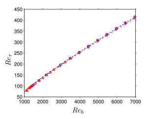
FIGURE 3.3: Friction Reynolds number  $Re_{\tau}$  vs. bulk Reynolds number  $Re_b$ . Symbols indicate:  $\circ$ , open duct;  $\triangle$ , closed duct. Blue dashed and red dash-dot line indicate predictions by the empirical formula of Jones (1976).
