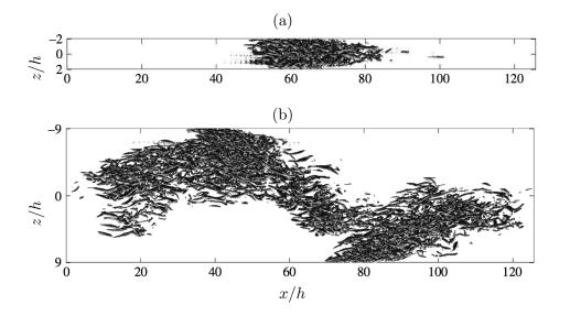
FIGURE 1.4: Examples of turbulent (a) *puff* and (b) *band*. The flow configurations are the rectangular closed duct with the aspect ratios at: (a) 2 and (b) 9. The visualised turbulent structures are the iso-contours based on the Q-criterion of Hunt et al. (1988). The figures are from Takeishi et al. (2015).
