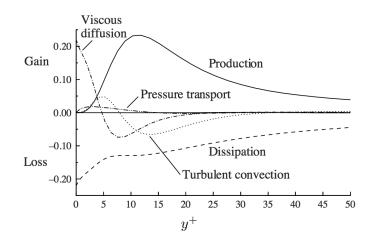
FIGURE 1.7: The turbulent-kinetic-energy budget in the viscous wall region of plane channel flow with  $Re_{\tau} = 180$  (DNS data from Kim et al. (1987)). All quantities are in the wall units. This figure is from Pope (2000).
