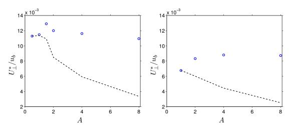
FIGURE 4.34: Side-wall secondary flow intensity  $U_{\perp}^*$  vs. aspect ratio A. Black dashed line indicates the corresponding full secondary flow intensities  $U_{\perp}$ . Value of a is fixed at unity, whereas  $Re_b$  is fixed at 2205. (a) open, (b) closed duct flow.
