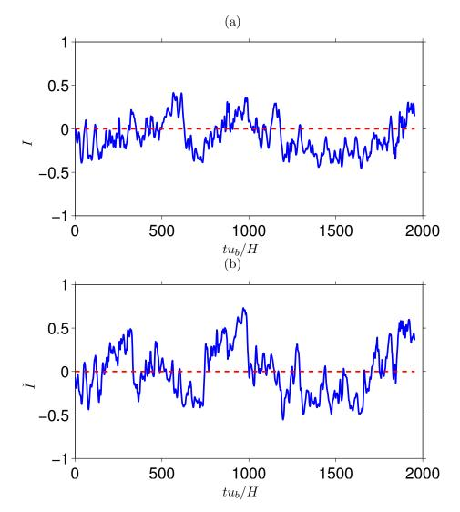
FIGURE 4.16: (a) Temporal evolution of the indicator function I of the open duct simulation with  $Re_b = 1080$  and A = 2. (b) same plot with the alternative indicator function  $\check{I}$ . Red dashed lines indicate  $I = \check{I} = 0$ .
