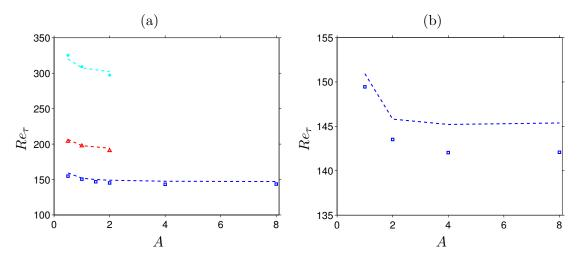
FIGURE 4.1: Friction-based Reynolds number  $Re_{\tau}$  as function of aspect ratio A, of (a) open and (b) closed duct respectively. Coloured symbols indicate the value of the bulk Reynolds numbers:  $\Box$ ,  $Re_b = 2205$ ;  $\triangle$ ,  $Re_b = 3000$ ; \*,  $Re_b = 5000$ . Dashed lines indicates predictions by the empirical formula of Jones (1976).
