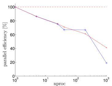
FIGURE 2.4: Parallel efficiency for two numbers of Chebyshev modes in y-direction:  $M_y = 33$ ,  $\circ$ ;  $M_y = 67$ , +. The number of modes in the x-/z-direction are fixed at  $M_x = 3075$  and  $M_z = 1025$  respectively. The runs were performed on Cray XC40 HORNET at HLRS. This figure is from Sakai and Uhlmann (2016).
