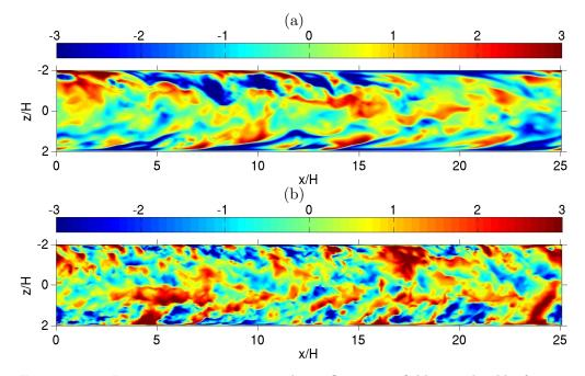
FIGURE 4.38: Instantaneous streamwise velocity fluctuation field normalised by friction velocity  $(u'/u_{\tau})$ , plotted on xz-plane approximately  $10\delta_{\nu}$  below the free-slip plane, in open duct flow with A = 2. (a)  $Re_b = 2205$ , (b)  $Re_b = 5000$ .
