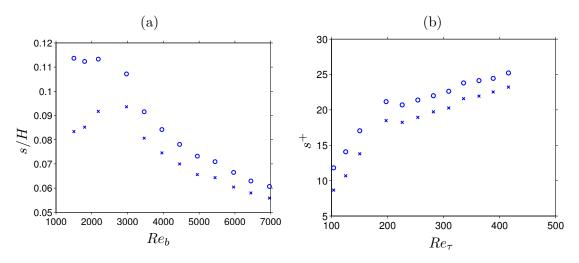
FIGURE 3.9: Positions of extrema of  $\langle \psi \rangle(y,z)$  of inner secondary flow cell in: (a) external coordinates vs.  $Re_b$  and (b) wall coordinates vs.  $Re_{\tau}$ . Symbols:  $\circ$  distance to z/H = -A;  $\times$  distance to y/H = 1.
