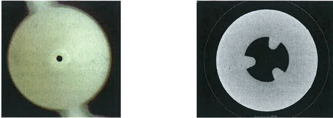
Fig. 6: Pictures of first samples, top view showing the nozzle orifice with a diameter of 100 \mu m (left) and CT image showing the alignment features.
