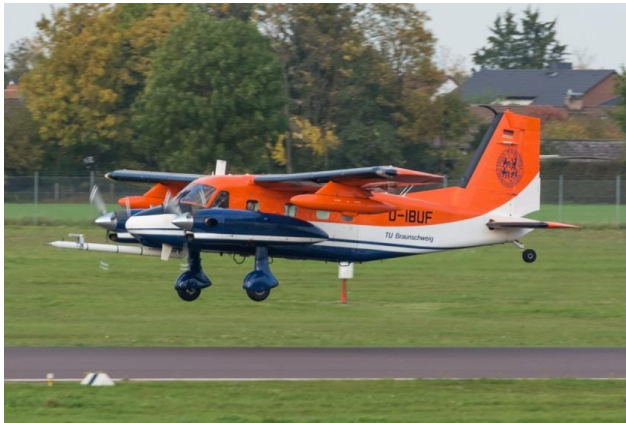
Figure 5. The research aircraft Do-128 D-IBUF of TU Braunschweig is equipped with a nose boom for meteorological measurements. The laser scanner is located in the cabin, looking downward (Photo: Uwe Bethke).
