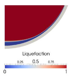
Figure 3.16: Liquid (red) and solid (blue) salt in LIVE-L1 calculated by the PECM
