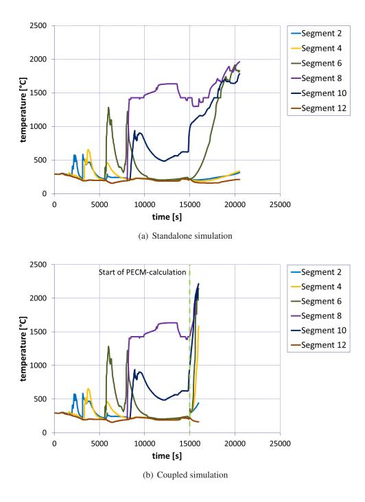
Figure 6.10: Temperatures of the inner lower head surface
