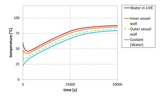
Figure 3.5: Temperature development in experiment *LIVE*-I1 simulated by *MELCOR* with modified heat transfer model
