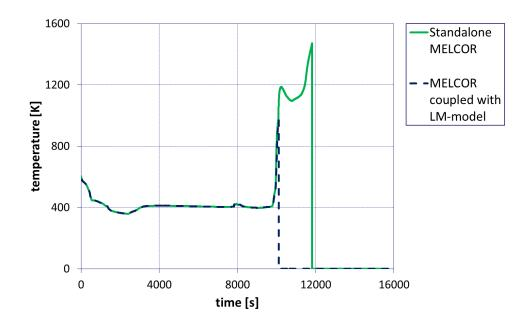
Figure 5.3: Temperature profile in the lower core support plate in *MELCOR* with and without the coupled Larson-Miller-Model
