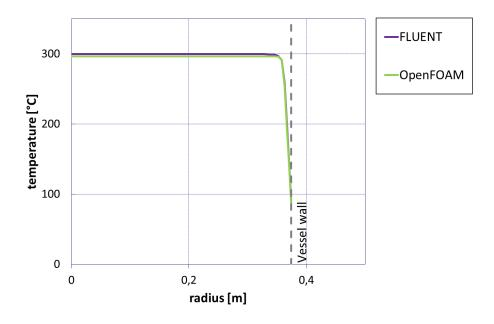
Figure 3.12: Temperature profiles in the melt pool along a horizontal line at a distance of 0.17 m from the bottom of the lower plenum
