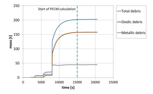
Figure 6.5: Debris masses in the lower plenum
