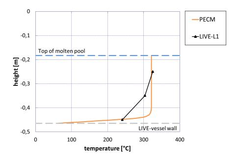
Figure 3.14: Temperature profiles in the melt pool along a vertical line at a distance 0.175 m from the symmetry axis compared to *LIVE*-L1 results
