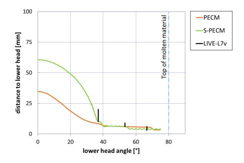
Figure 4.11: Crust thickness along the lower head in the *S-PECM* with a volumetric heating power of 29 kW compared to experimental data from *LIVE*-L7v and the traditional *PECM*
