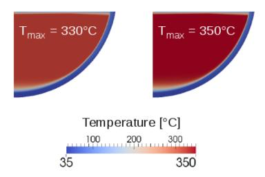
Figure 4.5: Temperature distribution in the modified PECM (left) compared to the traditional approach (right)
