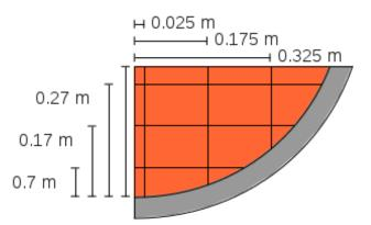
Figure 3.10: Positions of the evaluation lines to analyse the temperature profiles in the PECM
