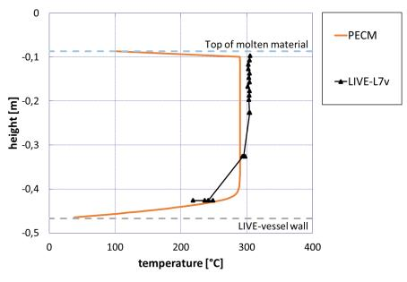
(a) Steady state with 18 kW volumetric heating power
