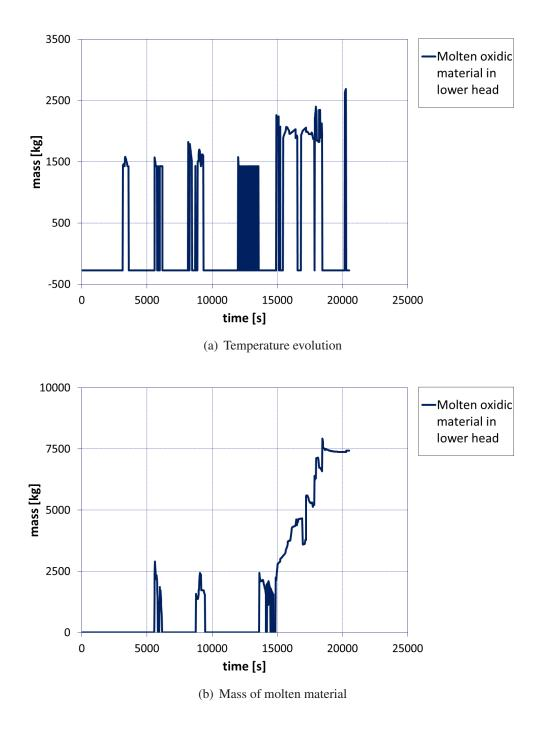
Figure 6.6: Temperature and mass of the molten oxidic material in the lower plenum of the RPV
