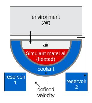
Figure 3.1: Thermohydraulic structure of the MELCOR input deck of the LIVE-facility
