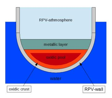
Figure 2.2: Material composition in the lower plenum during IVR
