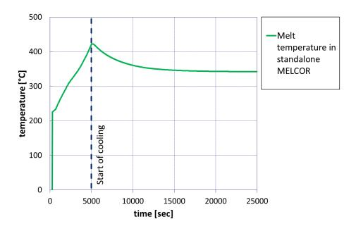
Figure 3.7: Temperature development in the molten pool for LIVE-L1 in MELCOR
