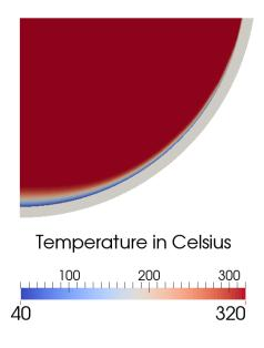
Figure 5.15: Temperature distribution in the coupled MELCOR-PECM simulation for LIVE-L10
