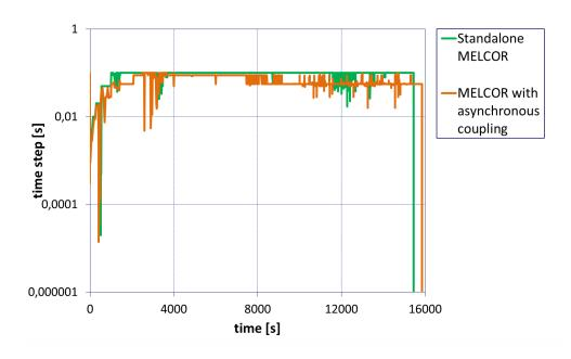
Figure B.2: Comparison of the MELCOR time step sizes to determine the influence of the coupling process
