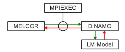
Figure 5.2: Schematic of the coupling process between to use the Larson-Miller-Model in MELCOR
