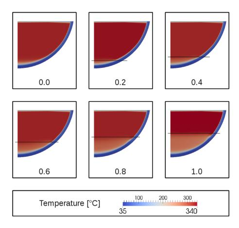
Figure 4.7: Temperature distribution with a volumetric heating power of 29 kW at different elevations (black lines) for the stratified zone
