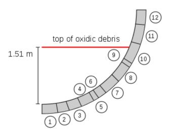
Figure 6.3: Nodalisation of the lower head of the generic NPP used to test the coupled MELCOR-PECM system
