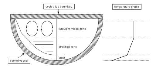
Figure 1.1: Different temperature and flow regimes in an internally heated fluid cooled through the adjacent boundaries
