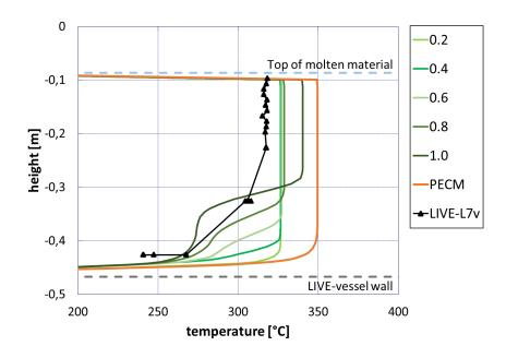
Figure 4.6: Vertical temperature profiles at 0.185 m from the centre with a volumetric heating power of 29 kW at different elevations for the stratified zone compared to experimental data from *LIVE*-L7v and the traditional *PECM*
