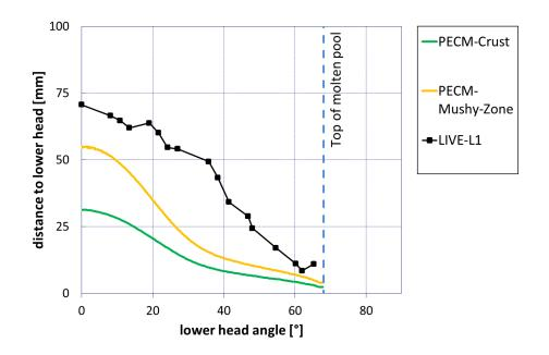
Figure 5.11: Crust and mushy-zone thickness along the *LIVE*-vessel inner wall in the coupled *MELCOR-PECM* simulation compared to experimental data from *LIVE*-L1
