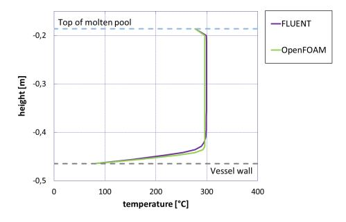
Figure 3.11: Temperature profiles in the melt pool along a vertical line at a distance 0.175 m from the symmetry axis
