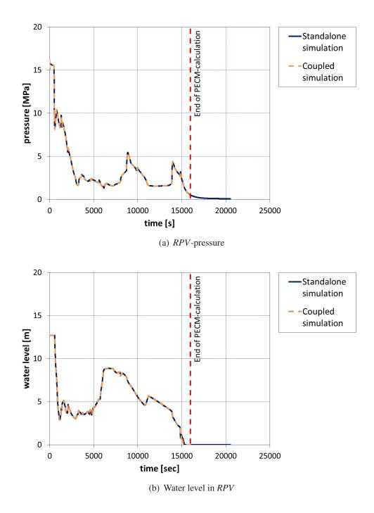
Figure 6.8: Pressure and water level development in the coupled severe accident simulation compared to standalone *MELCOR*
