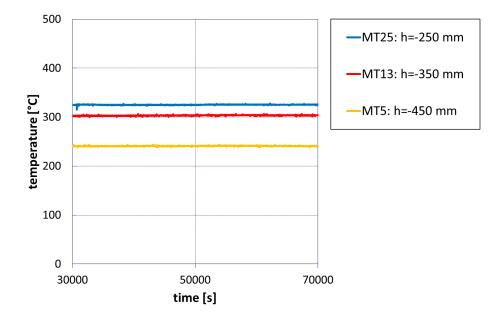
Figure 3.8: Temperatures of the molten salt in *LIVE*-L1 at different positions [58]
