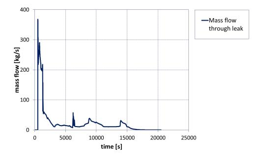
Figure 6.4: Mass flow rate through the leak in the cold leg FL 228
