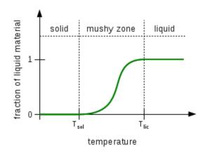
Figure 2.5: Fraction of liquid material depending on the local temperature
