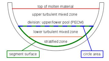
Figure 4.8: Surfaces to determine the height of the stratified region in a hemispherical lower head
