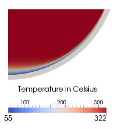
Figure 3.15: Calculated temperature distribution in the salt melt in *LIVE*-L1 with the *PECM*
