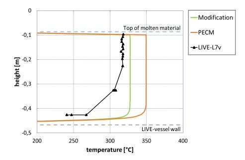
Figure 4.4: Vertical temperature profile at 0.185 m from the centre with a volumetric heating power of 29 kW in the modified *PECM* compared to experimental data from *LIVE*-L7v and the traditional *PECM*
