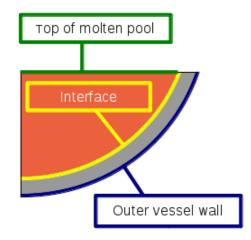
Figure 5.8: Active boundaries in the coupling process between MELCOR and the PECM
