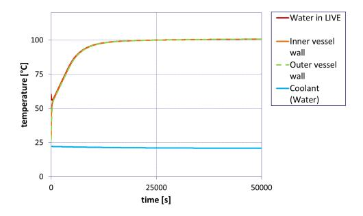
Figure 3.3: Temperature development in experiment LIVE-I1 simulated by MELCOR
