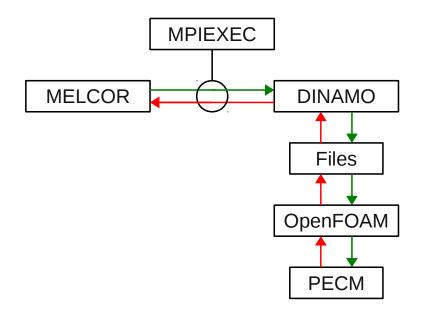
Figure 5.5: Scheme of the extended methodology to couple the PECM to MELCOR
