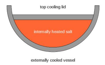
Figure 4.1: Simulation setup for the LIVE-L7v test with the PECM
