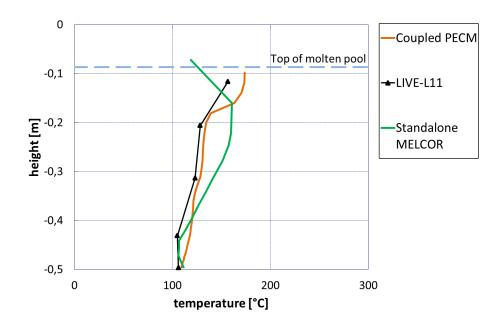
Figure 5.21: Temperatures at the inner vessel wall in the coupled *MELCOR-PECM* calculation compared to stand-alone *MELCOR* and experimental results from *LIVE*-L11
