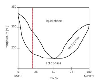
Figure 2.4: Phase-diagram of the KNO3-NaNO3 salt mixture
