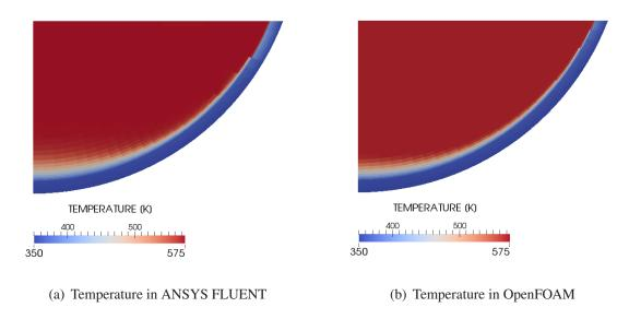
Figure 3.13: Comparison of the steady state temperature distribution with the *PECM* in ANSYS FLUENT and OpenFOAM
