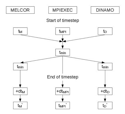
Figure B.3: Schematic of the synchronous time step progress
