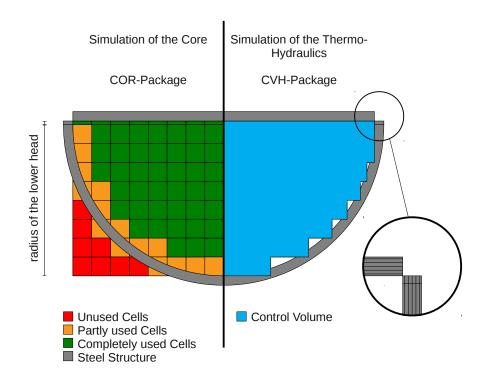
Figure 3.2: Nodalisation of the LIVE-vessel for simulating the core and the thermohydraulics
