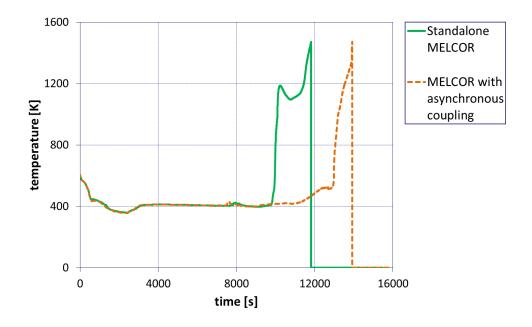
Figure B.1: Comparison of the temperature development in the lower core support plate to determine the influence of the coupling process
