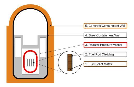
Figure 2.1: Successive barriers in the Defence-in-Depth approach according to [25]
