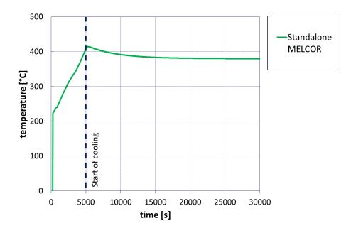
Figure 5.14: Temperature development in the molten salt pool in MELCOR for LIVE-L10
