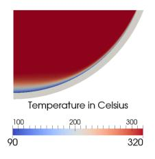
Figure 5.7: Temperature distribution for LIVE-L1 calculated by the PECM
