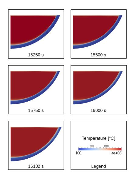
Figure 6.11: Temperature distribution in the oxidic material and the adjacent part of the lower head calculated by the *PECM* in a coupled simulation
