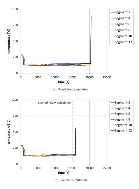
Figure 6.9: Temperatures of the outer lower head surface
