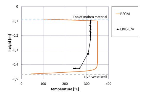
Figure 4.2: Vertical temperature profile at 0.185 m from the centre with a volumetric heating power of 29 kW in the *PECM* compared to experimental data from *LIVE*-L7v
