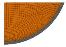
Figure 3.9: Grid for experiment *LIVE*-L1 used for the verification of the correct implementation of the *PECM* in OpenFOAM
