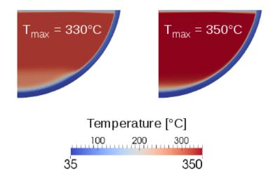
Figure 4.10: Temperature distribution in the S-PECM (left) compared to the traditional PECM-approach (right)
