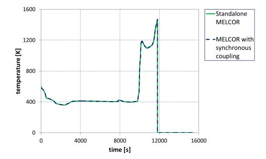
Figure B.4: Comparison of the temperature in the lower core support plate using the synchronized coupling process
