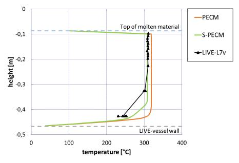
(b) Steady state with 24 kW volumetric heating power
