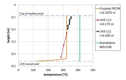
Figure 5.20: Vertical temperature profile in the coupled *MELCOR-PECM* calculation compared to stand-alone *MELCOR* and experimental results from *LIVE*-L11
