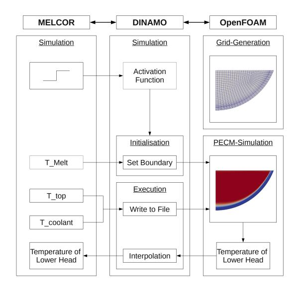
Figure 5.6: Coupling scheme between *MELCOR*, *DINAMO* and OpenFOAM for the implementation of the *PECM* to model molten core material in the lower plenum in *MELCOR*
