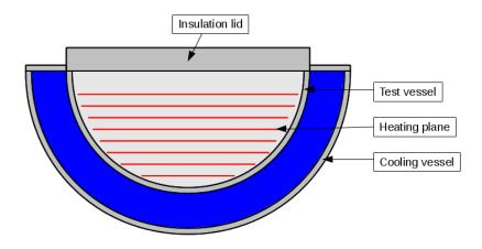
Figure 2.3: Schematic of LIVE-3D test vessel with insulation lid
