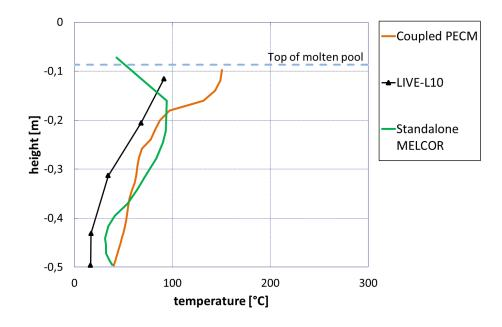
Figure 5.18: Temperatures at the inner vessel wall in the coupled *MELCOR-PECM* calculation compared to stand-alone *MELCOR* and experimental results from *LIVE*-L10
