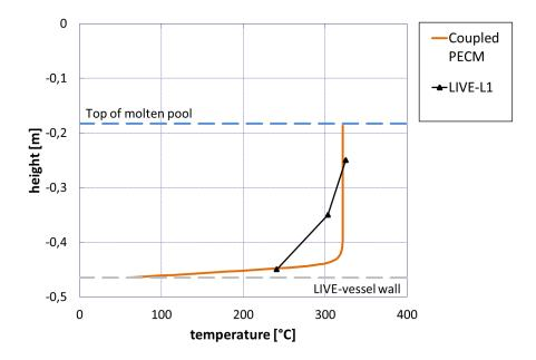
Figure 5.9: Vertical temperature profile along a vertical line at a distance of 0.175 m from the symmetry axis in the coupled *MELCOR-PECM*-simulation compared to experimental data from *LIVE*-L1
