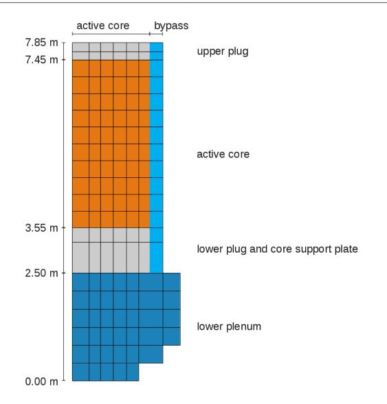
Figure 6.2: Nodalisation in the COR-package of the generic NPP used to test the coupled MELCOR PECM system
