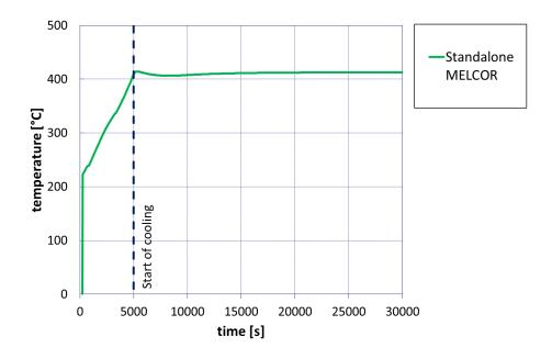
Figure 5.19: Temperature development in the molten salt pool in MELCOR for LIVE-L11
