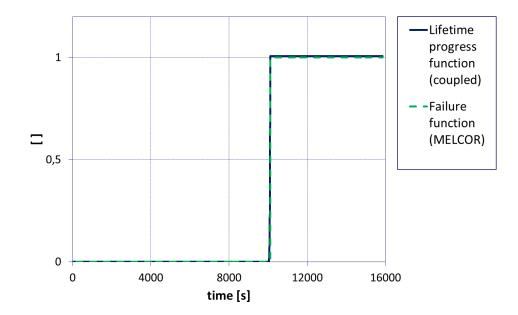
Figure 5.4: Progress of the life time progress function in *DINAMO* and the corresponding failure function in *MELCOR*
