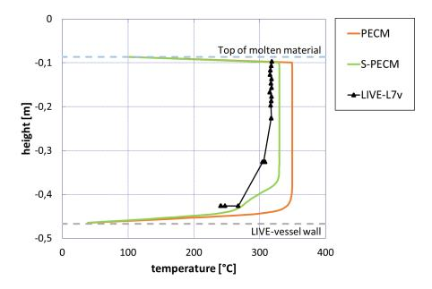
Figure 4.9: Vertical temperature profile in the *S-PECM* at a distance of 0.1875 m from the centre with a volumetric heating power of 29 kW compared to experimental data from *LIVE*-L7v and the traditional *PECM*
