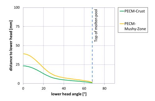
Figure 5.10: Crust and mushy-zone thickness along the *LIVE*-vessel inner wall in the coupled *MELCOR-PECM* simulation
