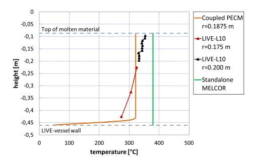
Figure 5.17: Vertical temperature profile in the coupled *MELCOR-PECM* calculation compared to stand-alone *MELCOR* and experimental results from *LIVE*-L10
