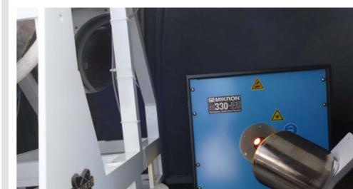
← High-temperature (1970 K) calibration blackbody source in the Zugspitze FTIR dome
