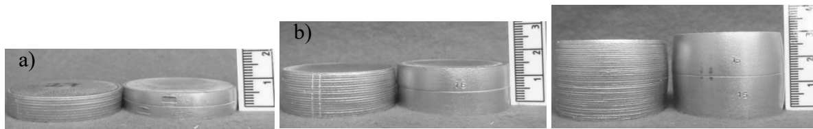
Figure 7: Comparison of diffusion-welded samples \phi=40 mm, h=10 (a); 20 (b) and 40 mm (c), made of two parts or of layers of 1 mm thickness.
