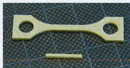
Printed tensile and bending test specimen
