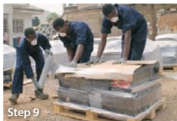
Step 9 Cover the top layer with cardboard and wrap with shrink wrap as many times as necessary to stabilize the load
