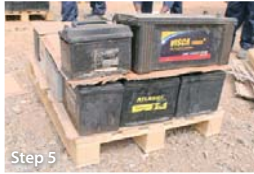
Step 5 Place a layer of card-board between every battery layer (also on the pallet)
