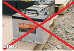
Step 7 Make sure that all batteries are placed within the horizontal limits of the pallet
