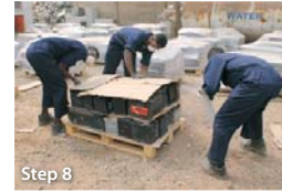
Step 8 Do not stack higher than 3 layers, place max. 1,000 kg on pallet, place damaged batteries in top layer
