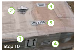
Step 10 Mark each pallet with the following warning labels: ① Package orientation ② Hazard label: Class 8, Corrosives ③ UN 2794: BATTERIES, WET, FILLED WITH ACID ④ Overpack
