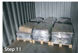
Step 11 Load the stacks into a container in a way that pallets are protected from sliding 4 Only load one layer of stacked pallets and avoid overloading 5
