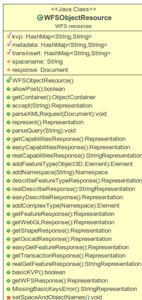
Figure 63 - UML class diagram of WFSObjectResource .
