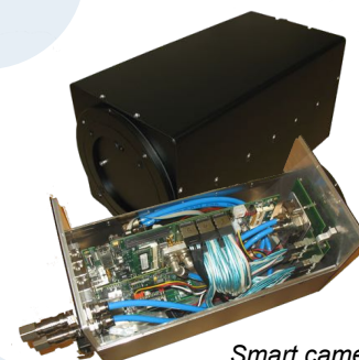
Smart camera for phase contrast X-ray tomography by Helmholtz-Zentrum Geesthacht and KIT.
