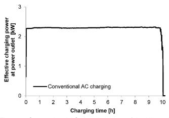
Figure 9: Conventional AC charging curve of the Nissan Leaf
