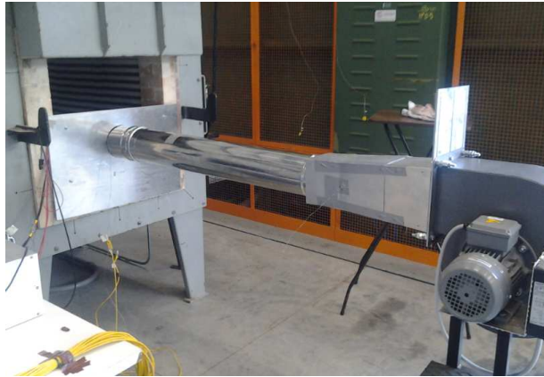
Figure 3 - View of the Fan-Inverter system
