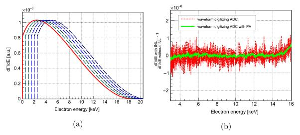
**Fig. 12.** (a) The original tritium β-decay spectrum (solid line) is shifted by post-acceleration for different post-acceleration voltages (dashed lines). (b) Ratio of tritium β-decay spectrum with/without INL and additional post-acceleration for a  $10^4$  pixels detector with waveform-digitizing ADCs. Due to the post-acceleration the fluctuations are mitigated down to a level of  $10^{-7}$ .
