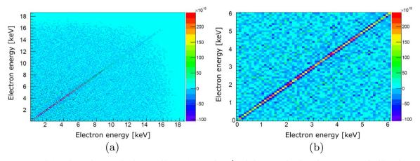
Fig. 13. Covariance Matrix of tritium decays of 1000 simulated KATRIN-like experiments with a 10<sup>4</sup> pixels detector, read out by peak-sensing ADCs with additional post acceleration of the electrons (a) and an expanded region of this matrix (b). The INL fluctuations behave like an additional statistical error on the energy spectrum and do not insert significant correlations between the energy bins.
