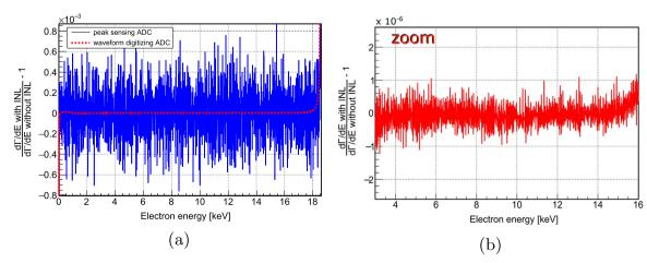
Fig. 11. (a) Ratio of tritium  $\beta$ -decay spectra with and without INL for the analytical simulation results for peak-sensing and waveform-digitizing ADCs for a multi-pixel detector with  $10^4$  pixels. The fluctuations for the peak-sensing case are of the order of  $10^{-4}$ . (b) A zoom in the ratio for the waveform-digitizing case shows fluctuations of the order of  $10^{-6}$ .
