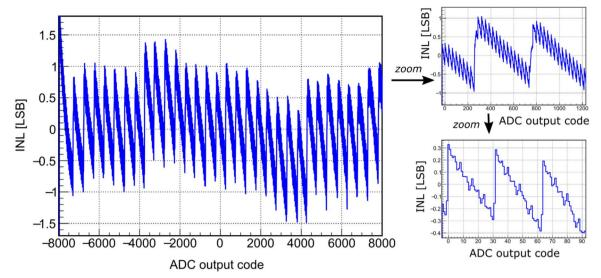
Fig. 4. INL of an AD6645 (Analog Devices) SAR-ADC of the GRETINA experiment [24] with 14 bits. The periodic structure reveals the internal structure of the comparators inside the ADC as approximately a 5 bits/4 bits/5 bits comparator with three steps of successive approximations.
