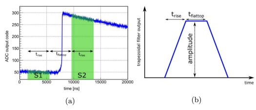
Fig. 7. Schematic of a trapezoidal filter. (a) For each point of the waveform the difference of the sums in the regions S2 and S1 is calculated and normalized to the number of sampling points in each of the regions. (b) Schematic of a trapezoidal filter output. The middle flat-top value of the filter output yields an amplitude proportional to the particle's energy.
