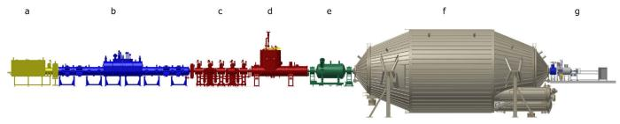
Fig. 1. Schematic overview of the KATRIN beam-line: rear section (a), windowless gaseous tritium source (b), differential pumping section (c), cryogenic pumping section (d), prespectrometer (e), main spectrometer (f) and focal plane detector system (g).
