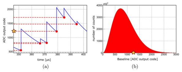
Fig. 10. (a) Simulated pulse-train. Due to the high rate the pulses sit on the tail of the previous pulse. Consequently the baseline of each signal varies. (b) The distribution of baselines as calculated from a pulse-train simulation shown in a) shows the frequency of the respective baseline ADC output codes of the simulated waveforms with the MC pulse train.
