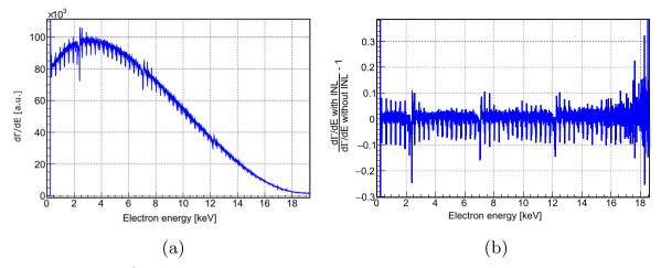
Fig. 8. (a) Tritium  $\beta$ -decay spectrum for  $10^8$  simulated signal pulses, whose energy outputs from the trapezoidal filter are de-corrected according to the INL value of the respective ADC output codes, modelling the working principle of a peak-sensing ADC. The steps in the INL are directly transferred into the resulting energy spectrum. (b) Shifted ratio of tritium  $\beta$ -decay spectra with and without INL.
