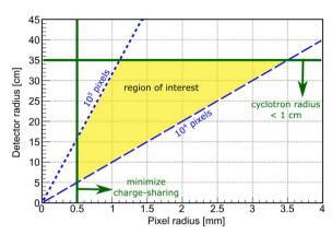
Fig. 15. The total number of pixels, the maximum allowed cyclotron radius and the minimization of charge-sharing effects set limits on the pixel and detector radius and define a region of interest.
