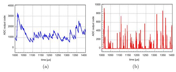
Fig. 6. (a) Excerpt of a simulated pulse train. Each pulse corresponds to an electron which creates a charge signal in a silicon detector. (b) After amplification and application of a trapezoidal filter, the peak heights of the shaped signals are used as a quantity which is proportional to the energies of the incident particles.
