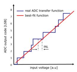
**Fig. 3.** Schematic of the transfer function and linear best-fit function of a real ADC with a non-uniform step width. The deviation between the transfer and the best-fit function is called integral non-linearity.
