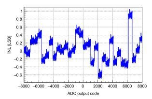
Fig. 5. Simulated INL spectrum of a 14-bit SAR-ADC with three successive approximation comparison steps (5-bit, 4-bit, 5-bit).
