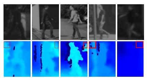
Figure 4.6: Collection of pedestrian samples with failing stereo-based head localization
