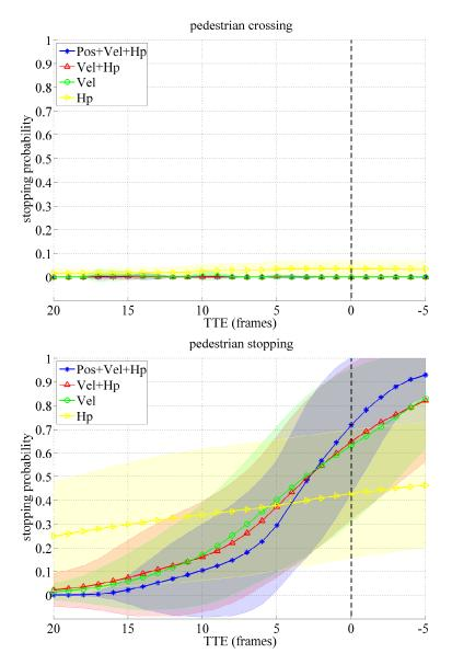
Figure 5.5: Stopping probabilities over TTE (frames) for the SC LDCRF model. Roadcrossing scenarios (upper graph) and stopping scenarios (lower graph). Visualized are mean and standard deviation (shaded area) over all tested sequences.
