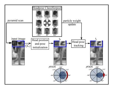
Figure 3.13: Head pose tracking system overview. The upper part (blue) of the pedestrian input image will be scanned by a set of head pose classifiers. Depending on the resulting confidence values  $\{C_i\}$  the head position and head pose get initialized. Additionally, tracking over time is realized using a particle filter, where the head pose classifiers are used once again to update the particle weights.
