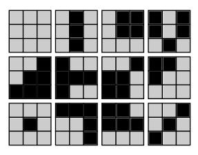
Figure 3.5: Examples of  $3 \times 3$  local structures: binary coded  $3 \times 3$  local structure leads to  $2^9$  possible structures that can represent lines, edges, points, etc.
