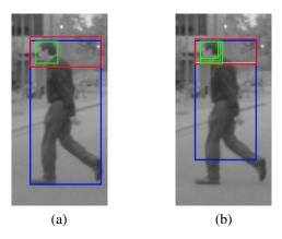
Figure 3.11: Pedestrian detection (blue), head search domain (red) and head detector search windows (green). The ideal height for the head search domain of 1/8 of the pedestrian's height (a), does not hold for imperfect aligned pedestrian detection hypothesizes (b). This has to be considered when defining the head search area.
