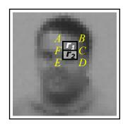
Figure 3.4: Two rectangle Haar-like feature calculation. Here the corner notations A, B, C, D, E and F represent the corner pixel values in the corresponding integral image.  $r_1$  and  $r_2$  represents the sum of all pixel values within the two rectangles. The feature value is the difference between  $r_1$  and  $r_2$ , as in equation (3.2).
