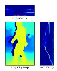
Figure 4.2: Calculated *u*- and *v*-disparity image for a given disparity map. Warmer colors correspond to larger disparities / smaller distances.
