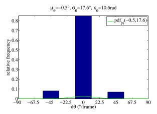
Figure 3.26: Process noise parameter estimation on the Bosch Inner-City dataset for the head pose state  $\theta$ . The probability density function (pdf) of a normal distribution gets fitted to the ground truth frame-wise angular changes for the pan angle  $\theta$ . The value of the estimate for the standard deviation  $\sigma = 17.6$  is directly related to the dispersion value  $\kappa_{\theta} = 10.6$  for the von Mises distribution.
