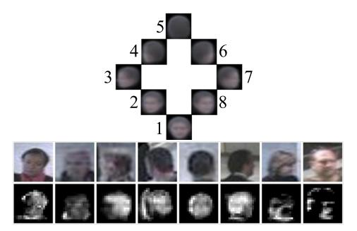
Figure 2.2: Method proposed by [Orozco et al., 2009]. Upper image: Head pose templates for each of eight discrete head pose classes using mean intensity image over training data. Lower Image Calculated Descriptor on a set of test samples.
