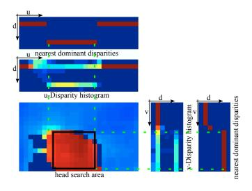
Figure 4.3: Stereo-based pedestrian head localization. Based on the u- and v-disparity images dominant foreground disparities are determined initially. Subsequently, concatenated areas or clusters are extracted, that have a common range of disparity values. The foreground clusters limit the head region in u- and v-direction and hereby described a rectangular region, which is then used as input for further pedestrian head pose estimation.
