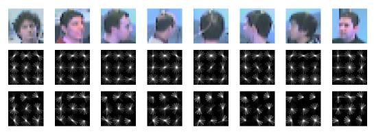
Figure 3.30: HoG descriptor from [Dalal and Triggs, 2005] calculated for different samples associated with 8 separated head pose classes. Upper row: Input images. Middle row: Original HoG settings with computed orientation angles in  $[0, \pi)$ . Lower row: Setup used in this work with computed orientation angles in  $[0, 2\pi)$ .
