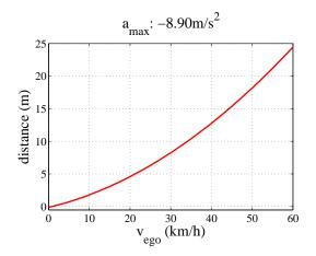
Figure 1.3: Typical brake characteristic curve for AEB systems. Object distance at which an AEB with a maximum deceleration of -8.9m/s<sup>2</sup> has to be triggered over ego vehicle speed.
