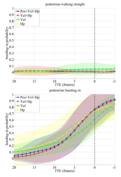
Figure 5.6: Bending-in probabilities over TTE (frames) for the BS LDCRF model. Straightwalking scenarios (upper graph) and bending-in scenarios (lower graph).
