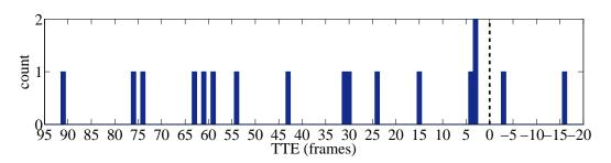
Figure 5.7: First occurrence of frontal head pose over TTE in stopping situations given by the Daimler dataset, [Schneider and Gavrila, 2013]. For some scenarios the expected pedestrian head turn towards the approaching vehicle occurs only after the actual stopping action.
