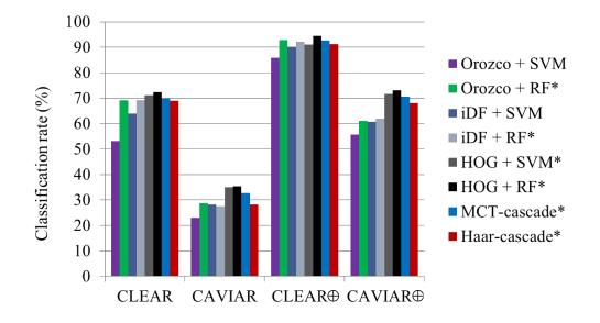
Figure 3.35: Comparison of different feature and classifier combinations on different datasets (CLEAR, CAVIAR).
