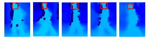
Figure 4.5: Collection of pedestrian samples with correct stereo-based head localization
