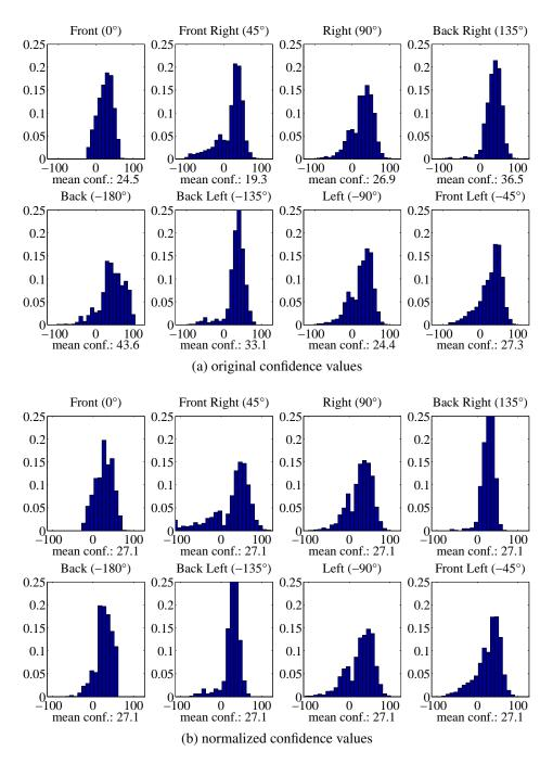
Figure 3.12: Distribution of confidence values for considered head pose classifiers over training data. (a) Original values with different ranges of values. (b) Normalized values with a common range of values.
