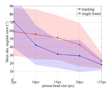
Figure 3.49: Mean absolute angular error (thick lines) and its standard deviation (shaded area) over ascending head sizes for the CAVIAR dataset.
