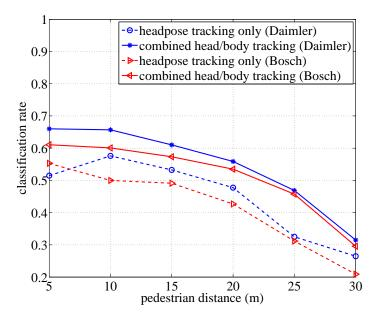
Figure 4.10: Head pose classification rates over pedestrian distance. Different curves show the results on different datasets (Bosch, Daimler), when using the origin head pose tracking module (Sec. 3.2.4) and the combined version incorporating the human body movement direction (Sec. 4.2).
