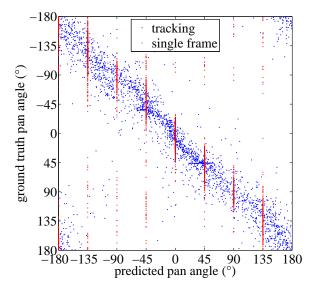
Figure 3.41: Distribution over predicted vs. ground truth head pan angles for the CLEAR dataset. Red data points: Estimates for single-frame based approach. Blue data points: Estimates for tracking approach.
