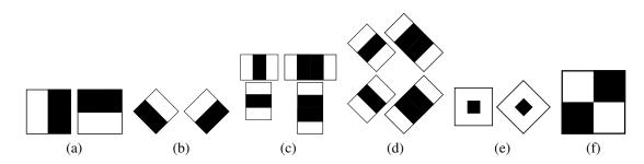
Figure 3.2: Haar-like features: the feature value is the difference between the intensity values sums between the black and white areas. a) edge features. b) Tilted edge features.c) Line features. d) Tilted line features. e) Center-surround features. f) Diagonal feature.
