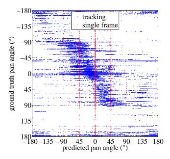
Figure 3.46: Distribution over predicted vs. ground truth head pan angles for the CAVIAR dataset. Red data points: Estimates for single-frame based approach. Blue data points: Continuous estimates for tracking approach.
