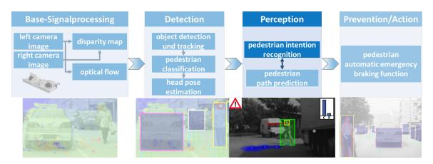
Figure 5.1: System Overview. Pedestrians are detected and tracked by a stereo generic obstacle detection approach and verified by a gray-value based classifier. For each pedestrian candidate the head orientation will be estimated. The previously extracted information is input for the intention recognition module.
