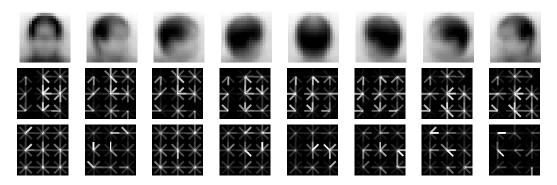
Figure 3.34: Most discriminative HoG features [Dalal and Triggs, 2005] learned with different classifiers. Upper row: Mean head pose templates. Middle row: Averaged support vectors for a trained one-vs.-all multiclass SVM. Lower row: most discriminative features learned with a one-vs.-all multiclass Random Forest.
