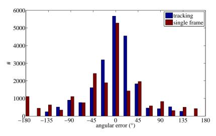
Figure 3.48: Distribution of angular errors in head pose estimation for the CAVIAR dataset
