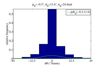
Figure 3.21: Process noise parameter estimation for the head pose state  $\theta$  on the CLEAR dataset. The probability density function (pdf) of a normal distribution gets fitted to the ground truth frame-wise angular changes for the pan angle  $\theta$ . The value of the estimate for the standard deviation  $\sigma = 11.6$  is directly related to the dispersion value  $\kappa_{\theta} = 24.6$  for the von Mises distribution.
