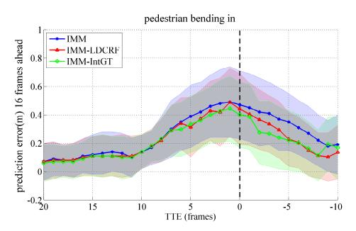
Figure 6.3: Lateral prediction error (*m*) when predicting 16 frames ahead around event occurrence for bending-in pedestrians. Visualized are the mean error and its standard deviation (shaded area) over all bending in scenarios from the evaluation dataset. Comparison between standard IMM filter prediction (blue), presented LDCRF-controlled IMM filter prediction (red) and a controlled IMM filter, when using the underlying GT intention for prediction (green).
