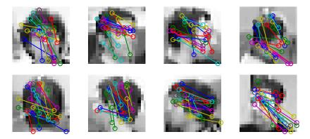
Figure 3.33: iDF classifier from [Siriteerakul et al., 2010]: 20 most powerful pixel pairs per head pose class for a one-vs.-all multiclass Random Forest.
