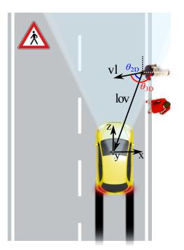
Figure 4.1: 3D head pan angle estimation with respect to vehicle located coordinate system. By calculating the line of view lov using stereo disparity estimates, the 3D head pan angle  $\theta_{3D}$  can be obtained from the 2D head pose estimate  $\theta_{2D}$ .
