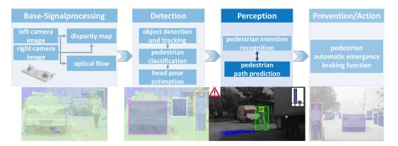
Figure 6.1: System overview. Pedestrians are detected and tracked by a stereo-video based generic obstacle detection and tracking approach and verified by an image intensity-value based classifier. For each pedestrian candidate the head orientation will be estimated from the image data. The previous extracted information serves as input for an iterative intention recognition and path prediction.
