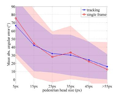
Figure 3.55: Mean absolute angular errors (thick lines) and its standard deviation (shaded area) over ascending head sizes for the Bosch Inner-City dataset.
