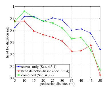
Figure 4.7: Head localization results over pedestrian distance on Daimler dataset. Blue curve: stereo-based only, see Section 4.3.1). Red curve: original 2D head pose detector-based version from Section 3.2.4. Green curve: combined version using updated measurement model from Section 4.3.2.
