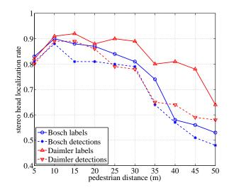
Figure 4.4: Stereo head localization rates over pedestrian distance (m) for the Bosch and Daimler dataset. Evaluation performed for pedestrian labels and system detections, separately.
