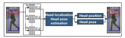
Figure 3.1: Signal processing chain for single frame based approach. Different head pose associated classifiers  $H_m$ , m = 1...8, evaluate all possible windows in the head search area (red) of a pedestrian detection (blue). The out-coming confidence values  $C_m$  are used to perform the head localization and pose estimation
