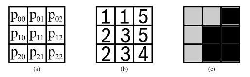
Figure 3.6: Modified Census Transform: (a)  $3 \times 3$  structure with the central Pixel  $\mathbf{p}_c = \mathbf{p}_{11}$ . (b) The intensity values in the neighborhood  $N(\mathbf{p}_c)$ . The mean intensity value can be calculated to  $\hat{I}(\mathbf{p}_c) = 2.89$ . (c) The resulting MCT structure by applying equation 3.4
