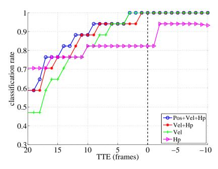
Figure 5.11: LDCRF classification rates in stopping scenarios for different feature combinations.
