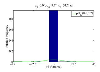
Figure 3.23: Process noise parameter estimation on the CAVIAR dataset for the head pose state  $\theta$ . The probability density function (pdf) of a normal distribution gets fitted to the ground truth frame-wise angular changes for the pan angle  $\theta$ . The value of the estimate for the standard deviation  $\sigma_{\theta} = 9.7^{\circ}$  is directly related to the dispersion value  $\kappa_{\theta} = 34.7$  for the von Mises distribution.
