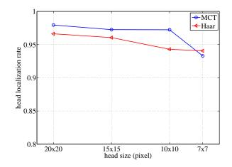
Figure 3.36: Correct head localization rates for different pedestrian heights in image pixels. The corresponding head sizes cover a range from  $20 \times 20$  pixels to  $7 \times 7$  pixels.
