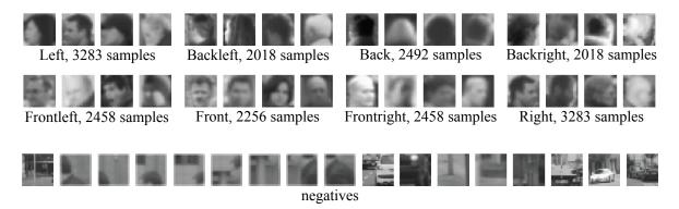
Figure 3.10: Examples of the training data for eight pedestrian head pose classes and negative samples
