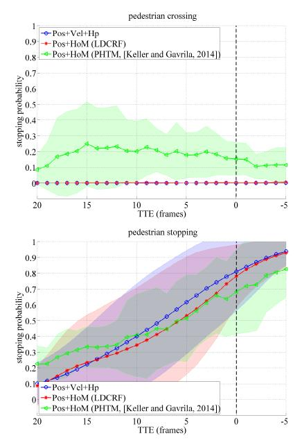
Figure 5.8: Stopping probabilities over TTE (frames) for the best LDCRF (blue), a LD-CRF model learned on pedestrian position and motion histograms (red) and the PHTM-like approach [Keller and Gavrila, 2014] (green).
