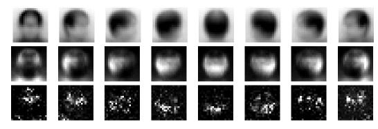
Figure 3.31: Most discriminative features learned with different classifiers. Upper row: Mean head pose templates. Middle row: Averaged support vectors for a trained one-vs.-all multiclass SVM using the method of [Orozco et al., 2009]. Lower row: most distinctive features learned with a one-vs.-all multiclass Random Forest.
