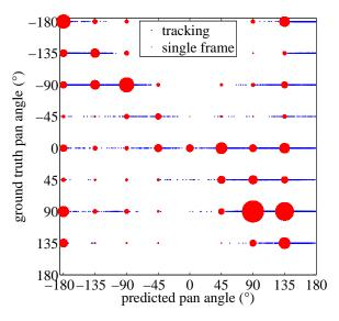
Figure 3.52: Distribution over predicted vs. ground truth head pan angles for the Bosch Inner-City dataset. Red data points: Discrete estimates for single-frame based approach. Blue data points: Continuous estimates for tracking approach
