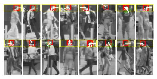
Figure 3.51: Pedestrian head pose estimation results in inner-city scenarios. Color gradient goes from green (frontal pose, i.e., less critical situation) to red (back poses, i.e., dangerous situation).
