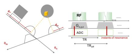
**Fig. 28:** Demonstration of the frequency sweep during readout gradients resulting in different instants of resonance for two different radial spokes for an off-isocenter voxel. The actual TR between two moments of excitation is referred to as effective TR,  $TR_{\rm eff}$ .
