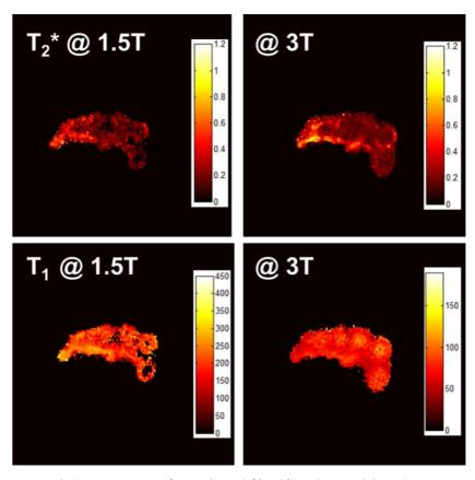
Fig. 51:  $T_2^*$  relaxation map in ms for 1.5T (upper left) and for 3T (upper right).  $T_1$  relaxation map in ms for 1.5T (bottom left) and for 3T (bottom right).
