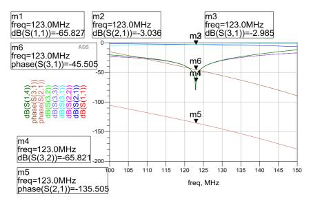
**Fig. A.6:** S parameter simulations for the hybrid coupler. Input power is equally divided between the ports 2 and 3, however with a 90° phase difference. Reflection coefficients and return losses are low enough to avoid unwanted signal leaks between transmit and receive ports.
