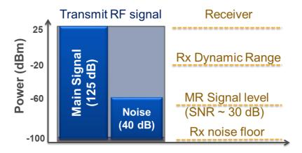
Fig. 25: Representative signal and noise level comparison.
