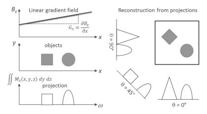
Fig. 8: Demonstration of frequency encoding applied to projection reconstruction in MRI.
