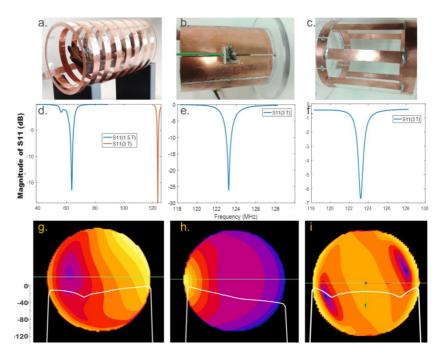
**Fig. 35:** Photos, reflection characteristics, and electromagnetic field simulations for three RF resonators. Photos of solenoid (a.), loop-gap (b.), and birdcage resonators (c.); corresponding S11 magnitude plots (d.),(e.),(f.); and simulated  $B_1$  field maps in axial plane with the line profile overlaid (g.),(h.), and (i.), respectively. Note the different axis ranges in d-f.
