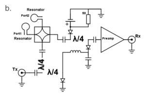
**Fig. 36:** Tx/Rx switch with high isolation and rapid switching time for linearly polarized single channel resonators (a.), and circularly polarized quadrature driven resonators, which uses a hybrid coupler to drive two ports of the resonator with  $\pi/2$  phase difference (b.)
