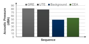
**Fig. 64:** Acoustic noise performance results. Continuous gradient-ramps in CEA reduced the acoustic noise significantly, close to the system's background noise.
