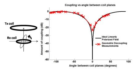
Fig. 57: Measured  $B_1$ -induced voltage for a rotation of the Rx resonator with respect to one of the Tx resonators. An ideal linearly polarized field is also calculated, and the angle between the resonators for both fields are scaled around  $0^{\circ}$ .
