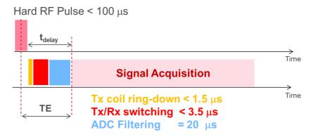
**Fig. 20:** Typical signal acquisition and RF pulse timing for FID based sequences. Acquisition delay depends on three factors. Design goals for each factor are given except the digital filtering which is not accessible for modifications.
