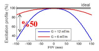
**Fig. 34:** Excitation profile simulation of sequences with different gradient levels. When the gradient level was halved during the RF pulse, a smoother slice was excited.
