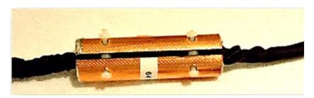
Fig. A.4: Floating BALUN placed on a shielded cable.
