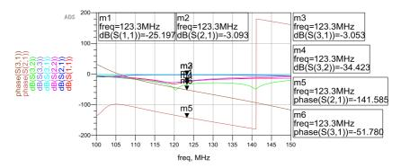
**Fig. A.8:** Quadrature Tx/Rx switch S-parameter simulation results. Isolation between Tx and Rx ports is 34.4 dB in Rx mode at 123.3 MHz (i.e. PIN diodes are in OFF state).
