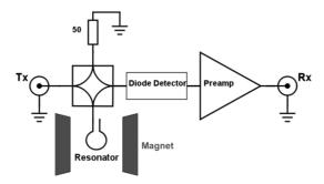
Fig. 7: Block diagram of a basic continuous-wave magnetic resonance spectrometer.
