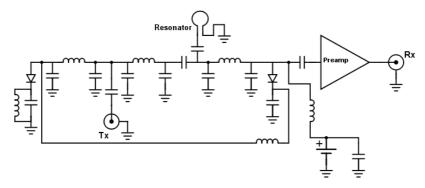
Fig. 17: Tx/Rx switch with shunt diode at the Tx side. There are three lumped element quarter wave transformers. Both PIN diodes are biased from the same source.
