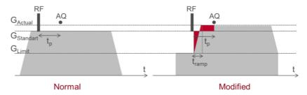
**Fig. 33:** Limitation of gradient level on RF excitation,  $G_{Limit}$ .  $G_{Actual}$  is the new peak amplitude for the modified gradient shape.
