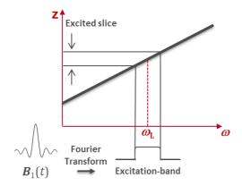
**Fig. 2:** Selective excitation. Fourier transform of  $B_1(t)$  approximates the slice profile.
