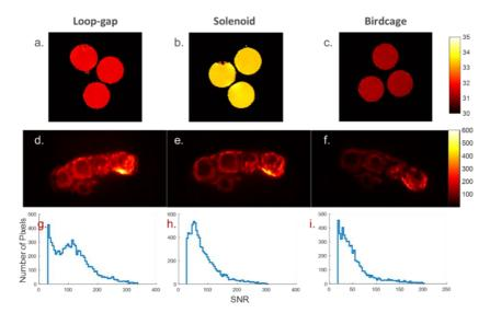
**Fig. 56:**  $B_1$  field maps when loaded with distilled water tubes described in section 3.1.3. for loop-gap (a.), solenoid (b.), and birdcage (c.) resonators. UTE images of the mummy hand acquired with each resonator (d.), (e.), (f.), and corresponding SNR histograms (g.), (h.), and (i.), respectively.
