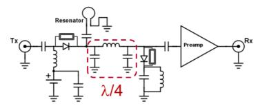
**Fig. 16:** Basic linear Tx/Rx switch.  $\lambda/4$  line is replaced by lumped elements. During Tx mode, PIN diodes are forward biased, thus the RF signal from the Tx port is sent to the resonator. In Rx mode, diodes are reverse biased blocking the RF path between the Tx and Rx port, thus the received signal from the resonator is sent to the Rx port via a preamplifier.
