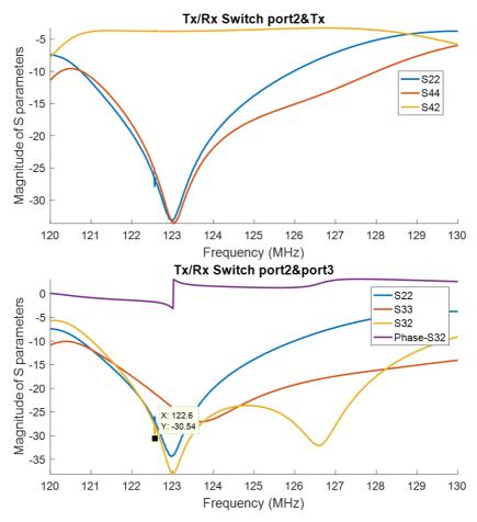
**Fig. A.10:** S parameter measurements between port 2 and Tx port (top), and port 3 and port 2 (bottom) of the quadrature Tx/Rx switch. S42 measurements verify that half of the power is transferred to the second port. S32 plots suggest that an isolation of more than 25 dB is secured between two ports connected to the resonator. Phase difference between S42 and S43 measurements is calculated as 87.7° at 123 MHz.
