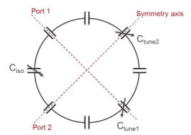
**Fig. 13:** Demonstration of tuning and isolation capacitor positions on an 8-leg high-pass quadrature birdcage resonator shown in axial plane.
