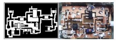
Fig. A.14: PCB Layout of 44x30 mm<sup>2</sup> (left), and the photo of the prototype LNA circuit (right).
