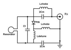
**Fig. 15:** PIN diode based active detuning circuit. When the diode is forward biased, the resonance shifts to a higher frequency due to increased inductance by Ldetune, thus the Rx resonator is decoupled from Tx resonators during RF excitation.
