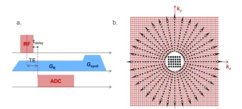
**Fig. 23:** PETRA sequence diagram. Gradients are always on during the RF pulse for the radial acquisition of outer sections of k-space. The center of k-space is missing because of the acquisition delay between the end of RF pulse and the beginning of the acquisition (a). SPI is used to cover the missing data points. PETRA k-space locations on a representative 2D grid (b).
