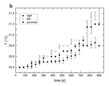
**Fig. 70:** (a) SE and GRE sequences were used for artifact width measurements. The edge of the container was used as reference for calculating the exact position of the electrodes. (b) Temperature measurement results over 15 min of RF transmission with TR = 30 ms. The temperature probes attached to the surface of the electrodes display higher temperature rises. Proximal probes was placed in close proximity (distance larger than 1 cm) of the electrodes.
