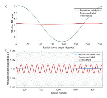
**Fig. 67:** Effective TR,  $TR_{\rm eff}$  with respect to the radial spoke angle for three different 2D k-space trajectories for a sample located in (x,y) = (150,150) on a 512x512 grid (a). Modulation in transverse magnetization with respect to the radial spoke number (b). The most extreme modulations are observed with golden angle ordering.
