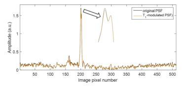
**Fig. 68:** Comparison of PSFs for  $T_1$ -modulated and constant TR reconstruction for a point source at the edge of the FOV (x,y) = (200,200) on 512x512 grid. Here the case with maximum of 5.2% difference in PSF is shown, which was calculated for golden angle ordering.
