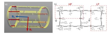
**Fig. 12:** Birdcage resonator and lumped element representation. (a) Schematic of birdcage leg and end-ring connections and representation of the leg current distribution resulting in a transverse magnetic field vertical to  $B_0$ . (b) Lumped element equivalent of a birdcage resonator for a hybrid design with capacitive elements in legs and end rings.
