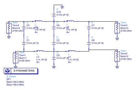
**Fig. A.5:** Hybrid coupler unit of the quadrature Tx/Rx switch. Capacitance of 25.9 pF and inductance of 65 nH were estimated for optimal performance at 12 MHz.
