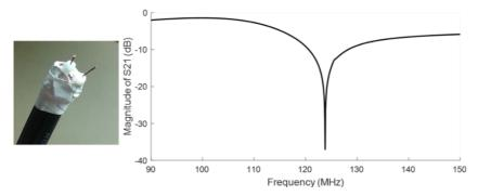
**Fig. A.2:** Measurement of a BALUN using an S21 common-ground probe (left) touched to the capacitor poles, and an exemplary S21 data acquired using a network analyser (right).
