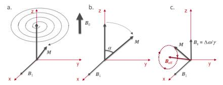
**Fig. 1:** RF Excitation and magnetization vectors. In the lab frame, actual motion of M is a spiral (left). In the rotating frame M precesses around the x-axis in response to an RF excitation,  $B_1$  (middle). When  $B_1$  is off-resonant with respect to Larmor frequency, M precesses in a cone around  $B_{\rm eff}$  at frequency  $\Delta \omega$ .
