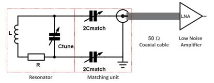
**Fig. 10:** A lumped element model of the RF resonator and the matching unit for an MR signal detector unit. Instead of a single matching capacitor of capacitance Cmatch at the inner conductor, capacitors of 2Cmatch are connected to both conducting lines for partially balanced matching.
