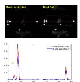
**Fig. 55:** Comparison of sequences with regular gradient level (top-right) and gradient level halved on RF (top-left) using a large loop resonator. Slice profile is smoother when the gradient level is halved during excitation, thus the edges are not suppressed (bottom).
