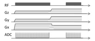
**Fig. 47:** Improved 3D radial CEA pulse sequence. Continuous gradient-ramps minimizes the acoustic noise. ADC and RF pulse events start after the gradient-ramp: gradient delay based systematic errors and ramp-up sampling are avoided.
