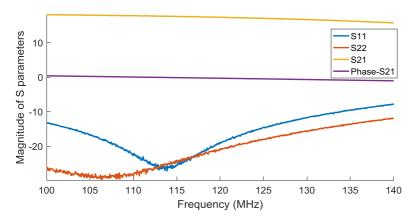
Fig. A.15: 17.4 dB gain at 123 MHz with 0.47 dB gain flatness within 10 MHz band is measured.
