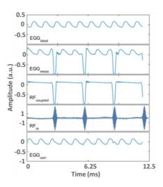
**Fig. 69:** Comparison of EGG signals for constant singing of A5: the ideal EGG signal with no RF pulse is applied (EGG<sub>ideal</sub>), EGG signal during 2D TrueFISP pulse sequence (EGG<sub>meas</sub>), RF induced voltage signal no singing (RF<sub>coupled</sub>), the applied RF pulse measured by oscilloscope (RF<sub>in</sub>) and the EGG signal after retrospective processing (EGG<sub>corr</sub>).
