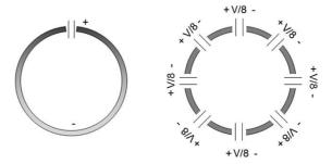
**Fig. 11:** Demonstration of the effect of distributing capacitance over the loop resonators. In single capacitor design (left) the magnetic field cancels out in the middle and the power on the capacitor is 64 times the power on each capacitor in the distributed capacitor design (right).
