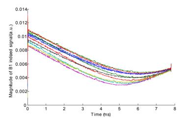
Fig. 62: Variation of  $B_1$ -induced leakage signal over subsequent measurements after decoupling. Due to the deviations in the leakage signal, the resulting images are prone to artifacts since the leakage signal is assumed to be constant during the acquisition of the entire k-space.
