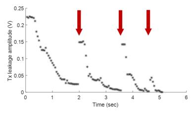
**Fig. 44:** Voltage level of the residual Tx induced leakage signal during automated feedback cancellation. Arrows show the instants when the hand position was changed and re-iteration was triggered.
