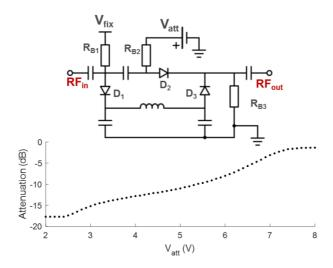
**Fig. 42:** Voltage controlled attenuator circuit schematic and voltage vs attenuation in logarithmic scale.  $R_{B1,2,3}$  are the bias resistors. Attenuation/Voltage ratio is  $3.0\pm0.3$  dB/V for  $V_{att}=2.5-8.0$  V, where  $V_{fix}=4.5$  V. Bypass capacitors, RF chokes and the impedance matching elements are excluded for simplicity.
