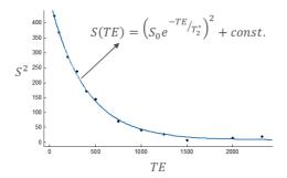
Fig. 24:  $T_2^*$  calculation for a strip band using an exponential fit over the data points acquired at different TE. Resulting  $T_2^*$  value is 205  $\mu$ s.
