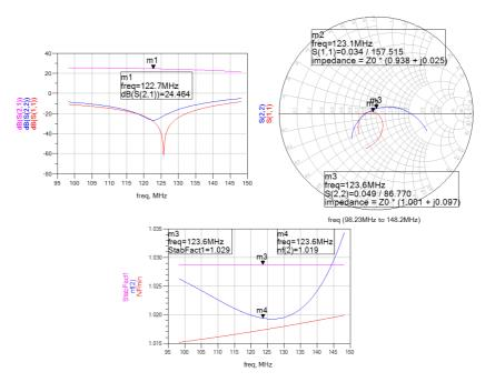
**Fig. A.13:** LNA simulation results. S parameter magnitude plots (left) shows a gain of 24.46 dB. Input and output matching conditions are shown in smith chart plot (middle). Stability factor and noise figure plots shows that the LNA is unconditionally stable and the noise figure is less than 1.02 dB between 120 MHz and 132 MHz.
