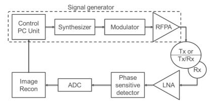
Fig. 14: Main elements of the Tx and Rx circuitry in MRI systems.
