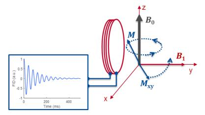
**Fig. 5:** Behavior of magnetization after excitation. Transversal component of the precessing magnetization induces a measureable voltage signal in a resonator. The generated signal is called FID, which is a damped sinusoid due to combined of precession and relaxation effects.
