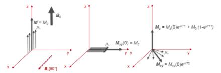
**Fig. 3:** Spin behavior demonstrated for the time frames of equilibrium (left), after excitation of 90° flip angle (middle), longitudinal ( $T_1$ ) and transverse ( $T_2$ ) relaxation (right). After the spins lose all their energy and become completely dephased, equilibrium state is reached again.
