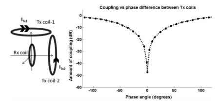
**Fig. 58:** Decoupling vs. phase of an RF generator unit. Phase and amplitude (PA) decoupling is represented by changing the phase of one Tx channel step by step over one cycle. The data are scaled around 0°.
