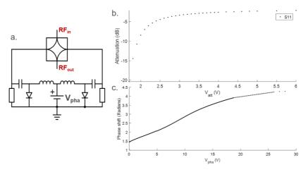
**Fig. 45:** Hybrid coupler based voltage controlled reflection type attenuator circuit design (a.), and the voltage vs. attenuation response for fixed phase shift (b.). Voltage response of the modified phase shifter (c.)
