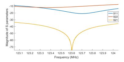
**Fig. 43:** Network analyzer measurement results for manually tuned analog cancellation circuit using the experimental resonator setup.
