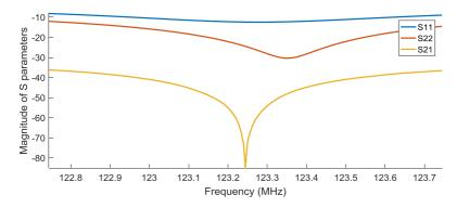
**Fig. 46:** Network analyzer measurement results for the analog cancellation circuit with matched attenuator using geometrically decoupled resonator setup. Isolation is higher (i.e. |S21| is lower) with the new analog cancellation circuit.
