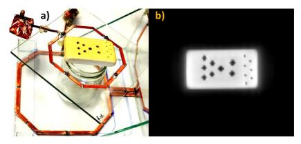
**Fig. 60:** (a) Rubber phantom with a  $T_2$ \* value of 500 μs with holes, (b) CEA image with a base resolution of 256 and 768 radial spokes; TR= 200 ms. There is blurring at the edges, but the holes of various dimensions (0.1-0.4 mm) drilled on the rubber are clearly visible.
