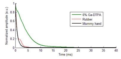
**Fig. 19:** Recording of the MR signal accumulated from the whole sample using a simple hard pulse excitation and immediate acquisition sequence. Signal from the mummified hand (cf. section 2.3.1.) decays faster than the 6% Ga-DTPA contrast agent solvent and a rubber sample.
