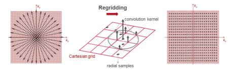
**Fig. 9:** Schematic of the re-gridding operation. The data is acquired as sequential radial spokes: dense in the center, sparse in periphery. Data values corresponding to each Cartesian grid points is calculated by interpolation of radial sampling points on to the Cartesian grid based on the selected convolution kernel. Finally, Cartesian k-space with uniform sampling is formed with proper density correction
