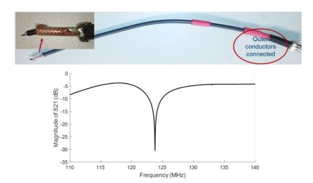
**Fig. A.3:** Bazooka BALUN was formed using a tri-axial cable (top), and corresponding S21 plot (bottom).
