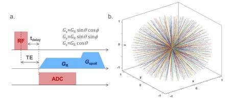
**Fig. 21:** UTE sequence diagram and radial trajectory. Pulse sequence diagram for UTE sequence with data acquisition starting at the ramp-up of gradients (a). The resulting k-space sampling points as radial inside-out spokes where the last data points of each spoke forms equidistant points distributed on a sphere (b).
