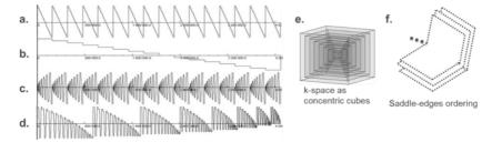
**Fig. 32:** A screen shot of gradient waveforms from sequence development software, IDEA (Siemens, Erlangen) for Gy of Seq. 1 (a.), Gz of Seq. 1 (b.), Gx of Seq. 2 (c.), Gz of Seq. 3 (d.) Demonstration of saddle-like ordering starting from concentric cubes (e.) and sampling points from outer most shell to the inner shells (f.).
