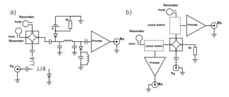
**Fig. 18:** Tx/Rx switch configurations for quadrature driven circularly polarized resonators. In (a), hybrid coupler divides and combines the signal both in Tx and Rx mode, whereas in (b) it is used only in Tx mode.
