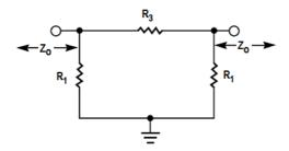
**Fig. 27:** A resistive  $\pi$  network applies controlled attenuation to the input RF signal.
