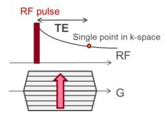
**Fig. 22:** SPI pulse sequence. Gradients are active during a very short block RF pulse. Here minimum echo time depends on the furthermost k-space point which is limited by the gradient strength.
