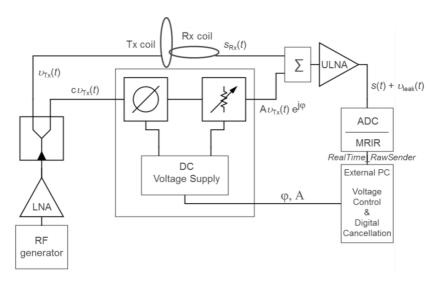
**Fig. 40:** System setup for analog cancellation with real-time feedback. An external PC controls the phase and attenuation level of a small copy of the Tx signal to minimize the mean of the residual leakage signal. This control is based on serial communication via USB connection. Data transfer from MR image reconstruction unit (MRIR) to the external PC is realized by TCP/IP protocol.
