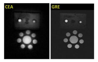
**Fig. 65:** Coronal slice from the 3D CEA MR image of the tube and rubber phantoms (left) and GRE image as the structural reference.
