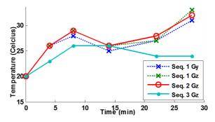
**Fig. 54:** Temperature measurements for four different gradient waveforms described in Methods, Fig.32. Measured temperature increase for the modified saddle-like k-space trajectory is substantially lower at the end of the measurement, and unlike the other gradient waveforms, it does not increase monotonically after 15 min.
