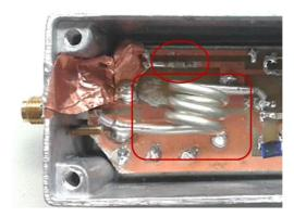
**Fig. A.1:** Solenoid BALUN part of an active detuning circuit. A resonant LC circuit is formed on the ground line to suppress unbalanced shield currents.
