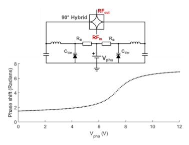
**Fig. 41:** Voltage controlled phase shifter simplified circuit and voltage vs. phase plot.  $R_B$  stands for bias resistors. Phase shifter enables  $280^\circ$  coverage for  $0 \text{ V} < V_{pha} < 12 \text{ V}$ . Nonlinear behavior is taken into account by using variable voltage step sizes in automated feedback decoupling.
