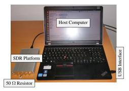
Figure 5.4: A measurement setup for acquiring the noise power.
