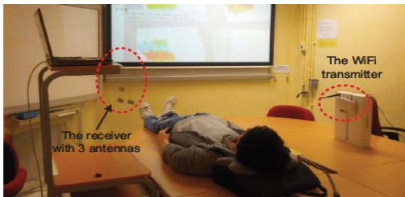
**Fig.1 WiFi devices, transmitter and receiver**
