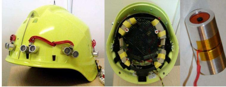
**Fig. 6.** The Tactile Helmet with its sensors on the outside and stimulators within, adjacent to a single stimulator element [1]
