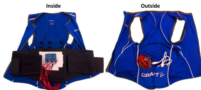
**Fig. 1.** Vibrotactile vest used by Novich and Eagleman [14] to compare encoding types and analyze tactual resolution on the lower back. The vest features an array consisting of 3x3 vibromotors. It also includes wireless controlling hardware and a power supply.
