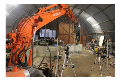
Figure 5-18: Setup of the second experimental series for other methods than mortising: equipment (left side), concrete block in a steel fitting (in the middle) and measurement systems (right side, at the back in the middle and at the front)
