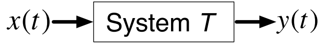
Figure 3.1: The system T maps the input signal x(t) to the output signal y(t) .
